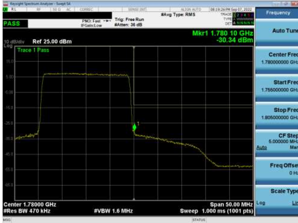
Plot 7-66. Upper Band Edge Plot (LTE Band 66 - 20MHz QPSK – Full RB)
