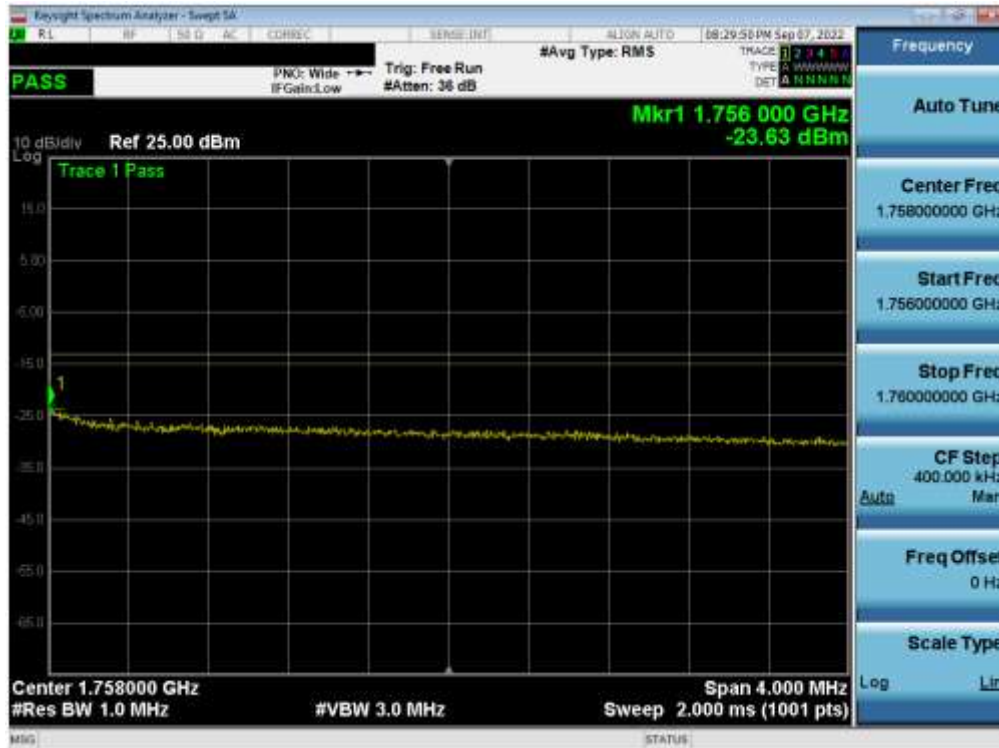
Plot 7-77. Upper Extended Band Edge Plot (LTE Band 4 - 10MHz QPSK – Full RB)
