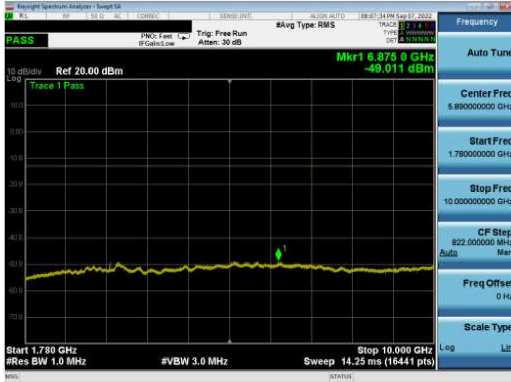
Plot 7-41. Conducted Spurious Plot (LTE Band 66/4 - 20MHz QPSK - 1 RB - Mid Channel)
