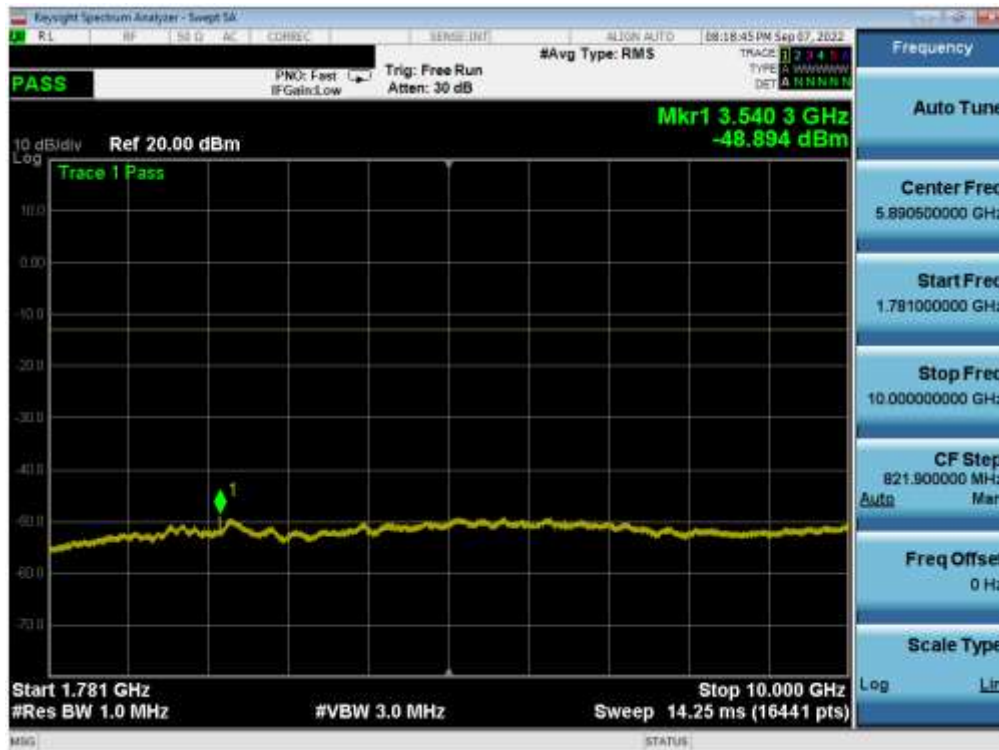
Plot 7-44. Conducted Spurious Plot (LTE Band 66/4 - 20MHz QPSK - 1 RB - High Channel)
