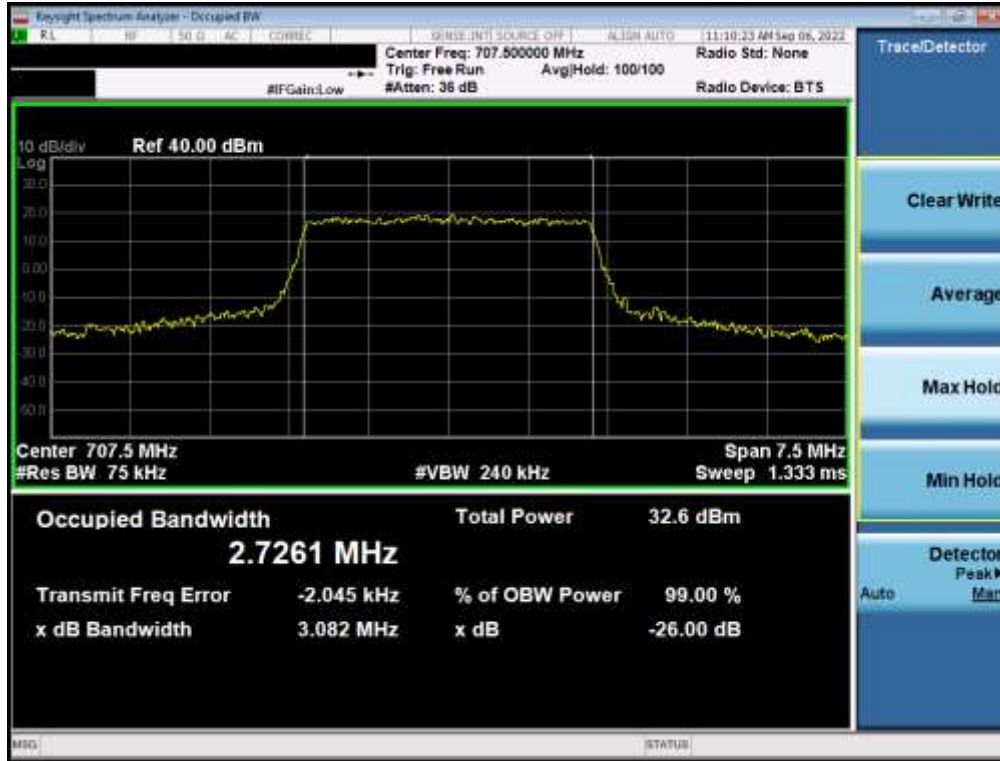
Plot 7-5. Occupied Bandwidth Plot (LTE Band 12 - 3MHz QPSK - Full RB Configuration)
