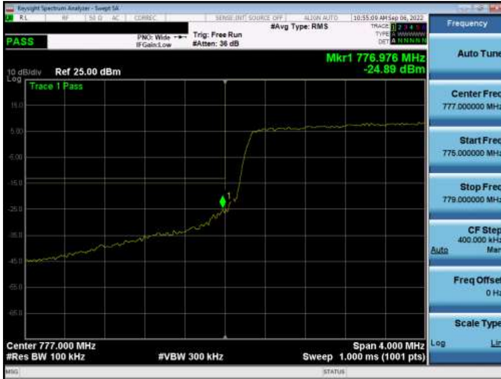
Plot 7-58. Lower Band Edge Plot (LTE Band 13 - 5MHz QPSK – Full RB)
