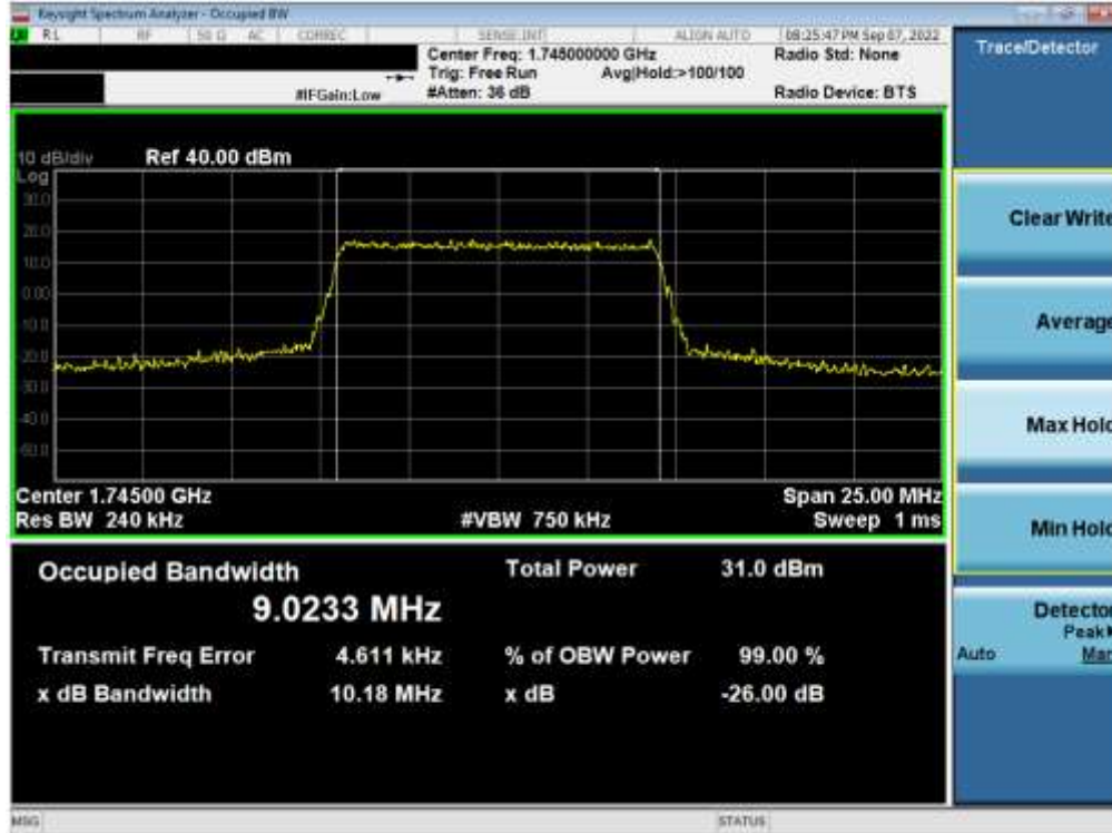
Plot 7-17. Occupied Bandwidth Plot (LTE Band 66/4 - 10MHz QPSK - Full RB)
