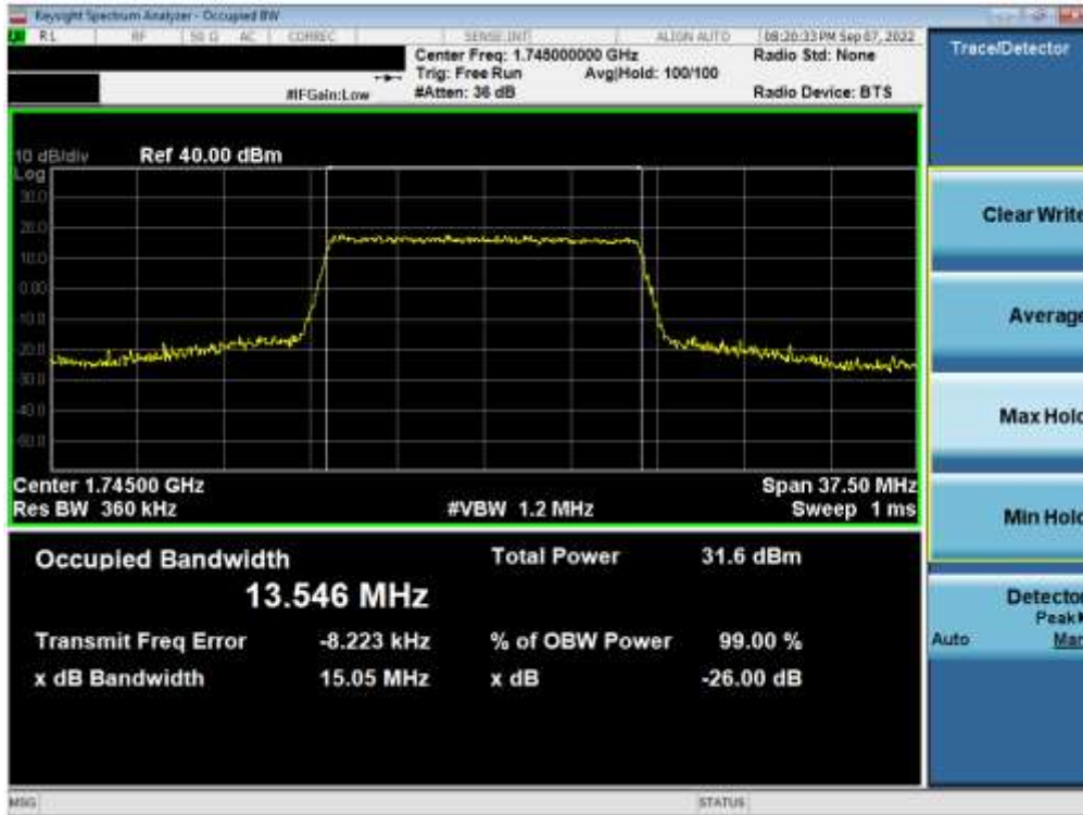
Plot 7-15. Occupied Bandwidth Plot (LTE Band 66/4 - 15MHz QPSK - Full RB)
