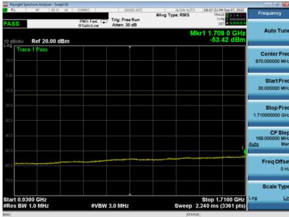
Plot 7-40. Conducted Spurious Plot (LTE Band 66/4 - 20MHz QPSK - 1 RB - Mid Channel)
