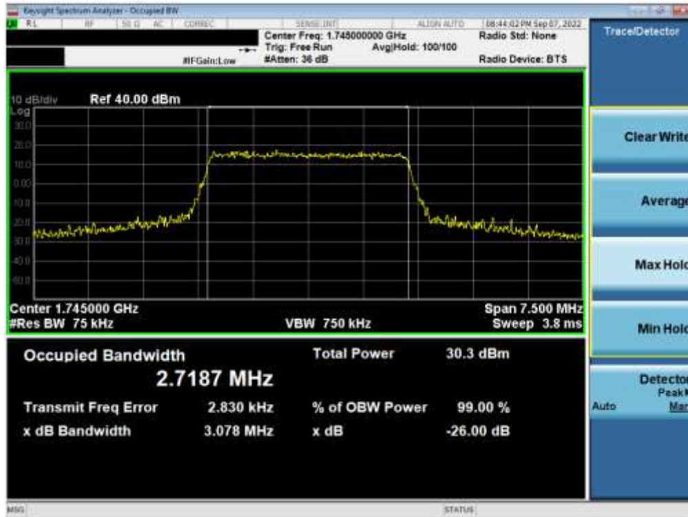
Plot 7-22. Occupied Bandwidth Plot (LTE Band 66/4 - 3MHz 16-QAM - Full RB)
