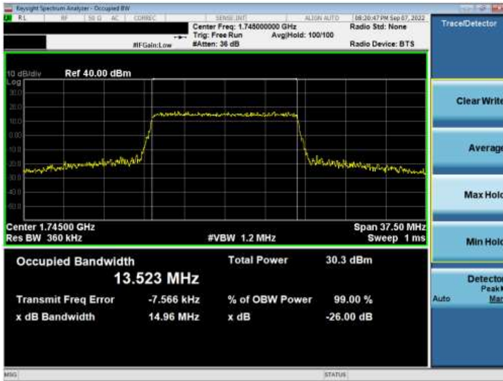
Plot 7-16. Occupied Bandwidth Plot (LTE Band 66/4 - 15MHz 16-QAM - Full RB)
