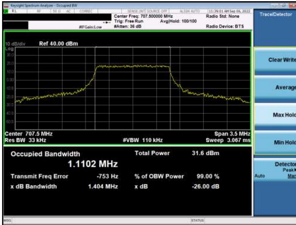
Plot 7-8. Occupied Bandwidth Plot (LTE Band 12 – 1.4MHz 16-QAM - Full RB Configuration)
