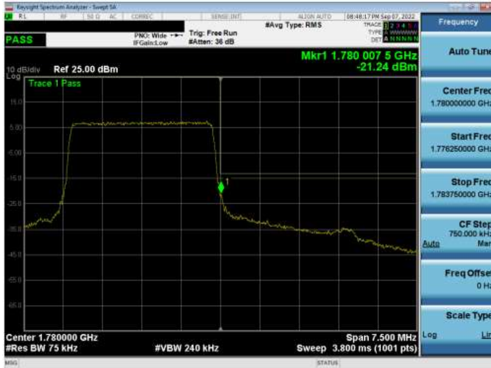
Plot 7-90. Upper Band Edge Plot (LTE Band 66 - 3MHz QPSK – Full RB)
