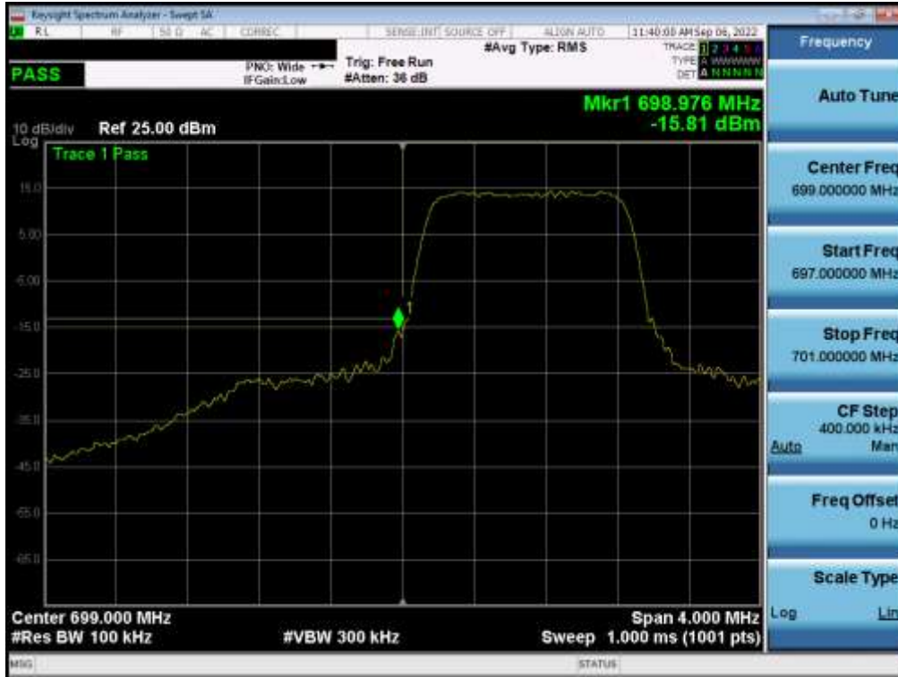
Plot 7-52. Lower Band Edge Plot (LTE Band 12 – 1.4MHz QPSK – Full RB)
