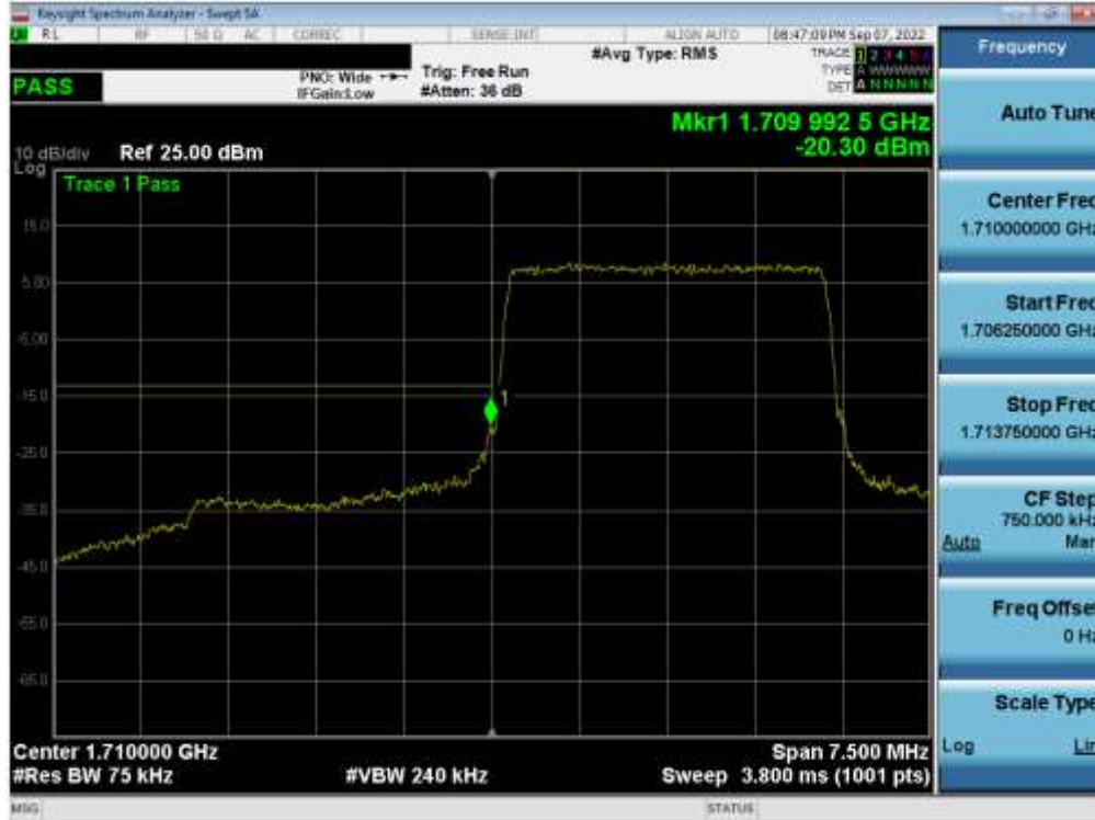
Plot 7-86. Lower Band Edge Plot (LTE Band 66/4 - 3MHz QPSK – Full RB)
