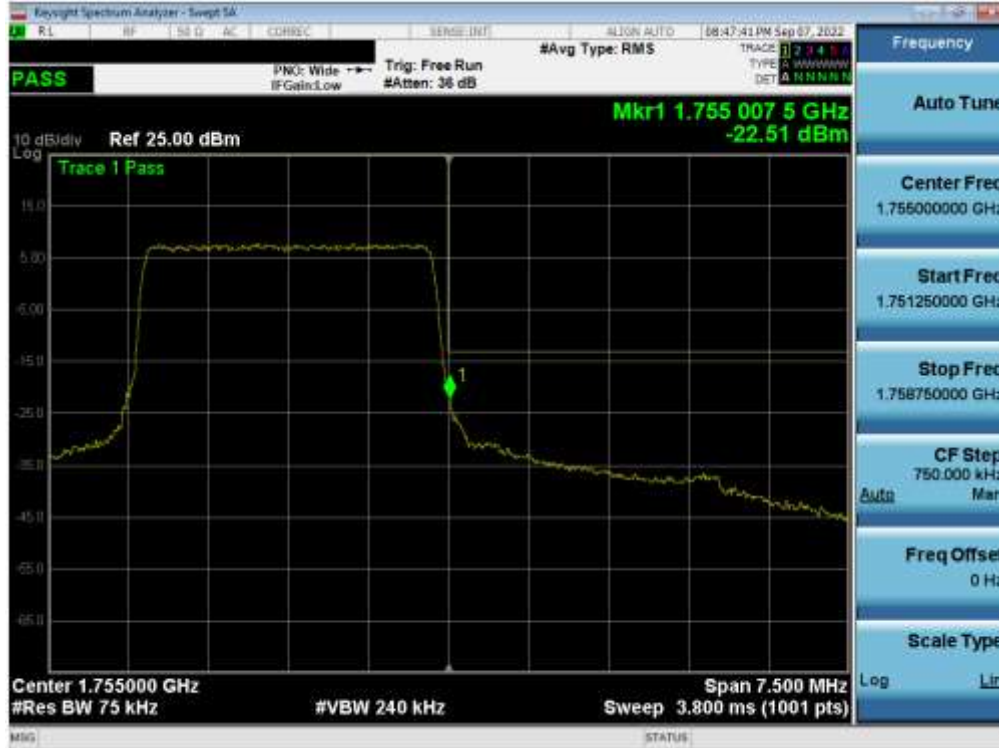
Plot 7-88. Upper Band Edge Plot (LTE Band 4 - 3MHz QPSK – Full RB)
