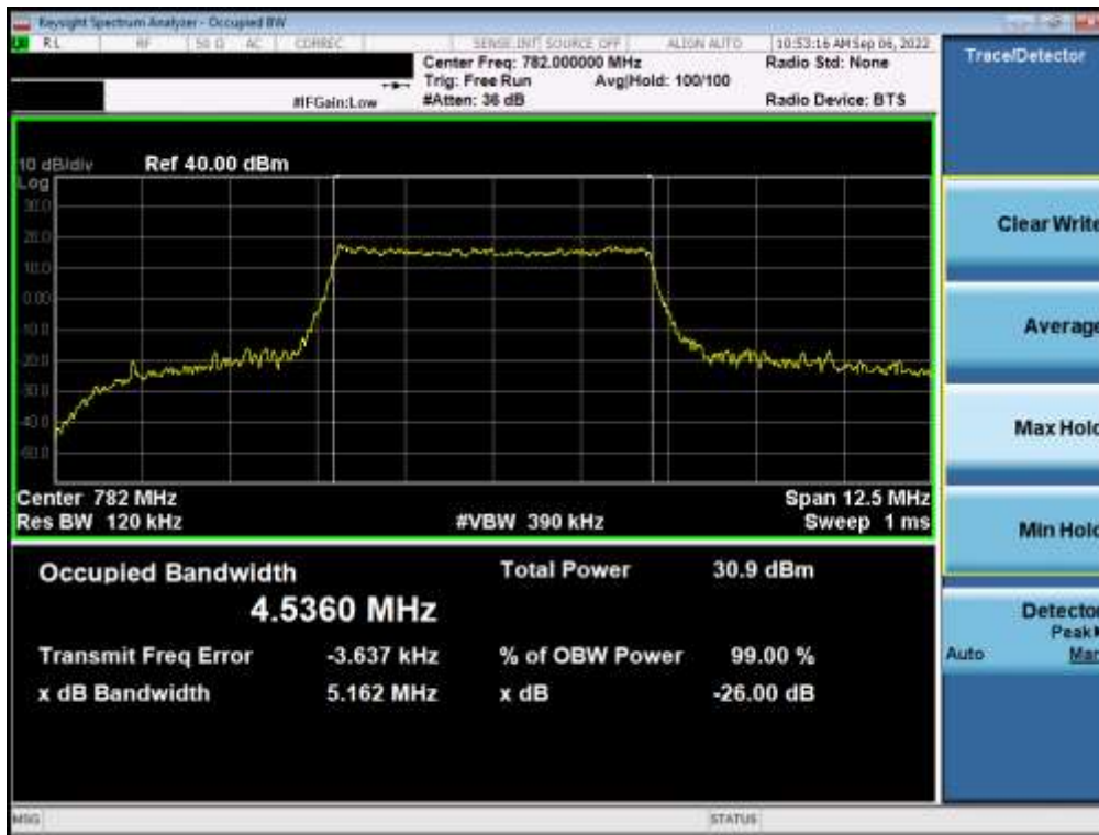
Plot 7-12. Occupied Bandwidth Plot (LTE Band 13 - 5MHz 16-QAM - Full RB)
