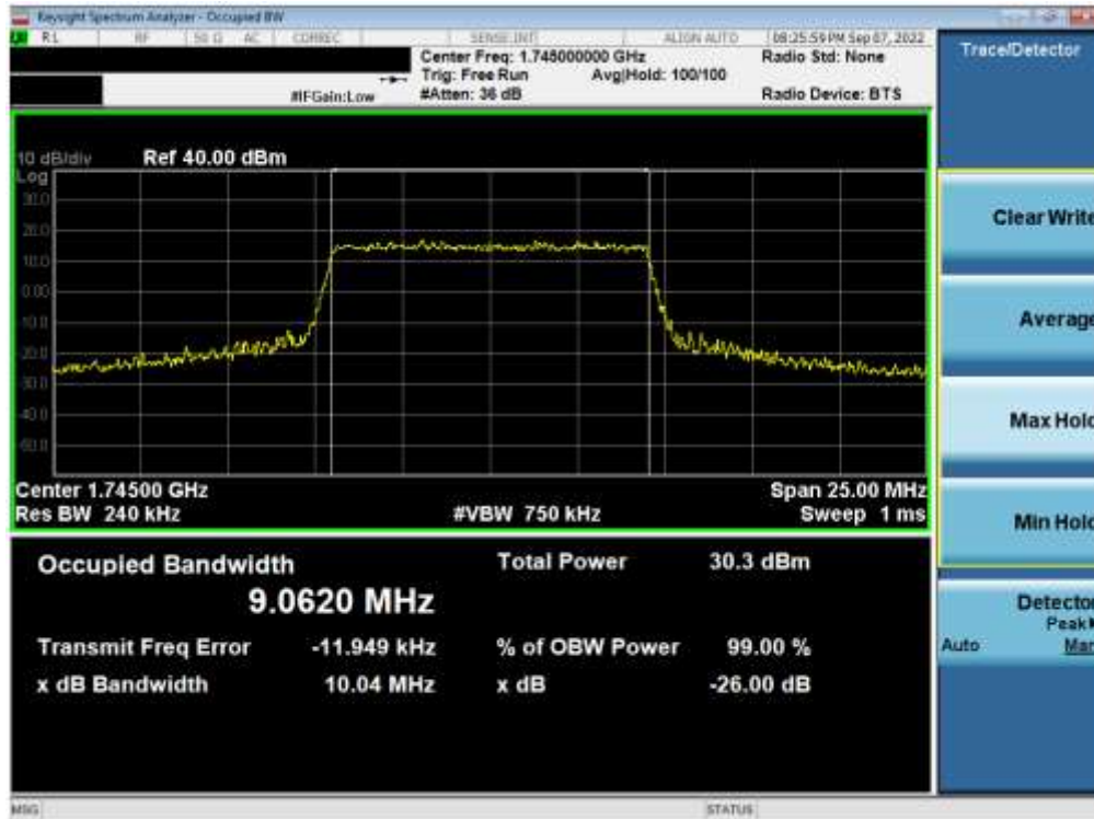
Plot 7-18. Occupied Bandwidth Plot (LTE Band 66/4 - 10MHz 16-QAM - Full RB)
