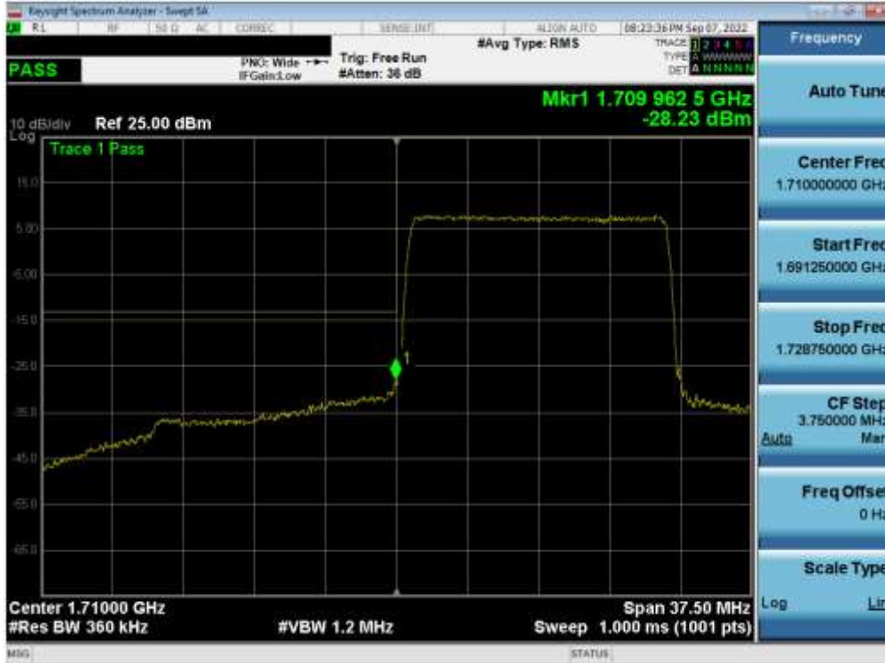
Plot 7-68. Lower Band Edge Plot (LTE Band 66/4 - 15MHz QPSK – Full RB)
