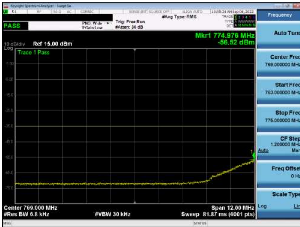
Plot 7-59. Lower Emission Mask Plot (LTE Band 13 - 5MHz QPSK – Full RB)
