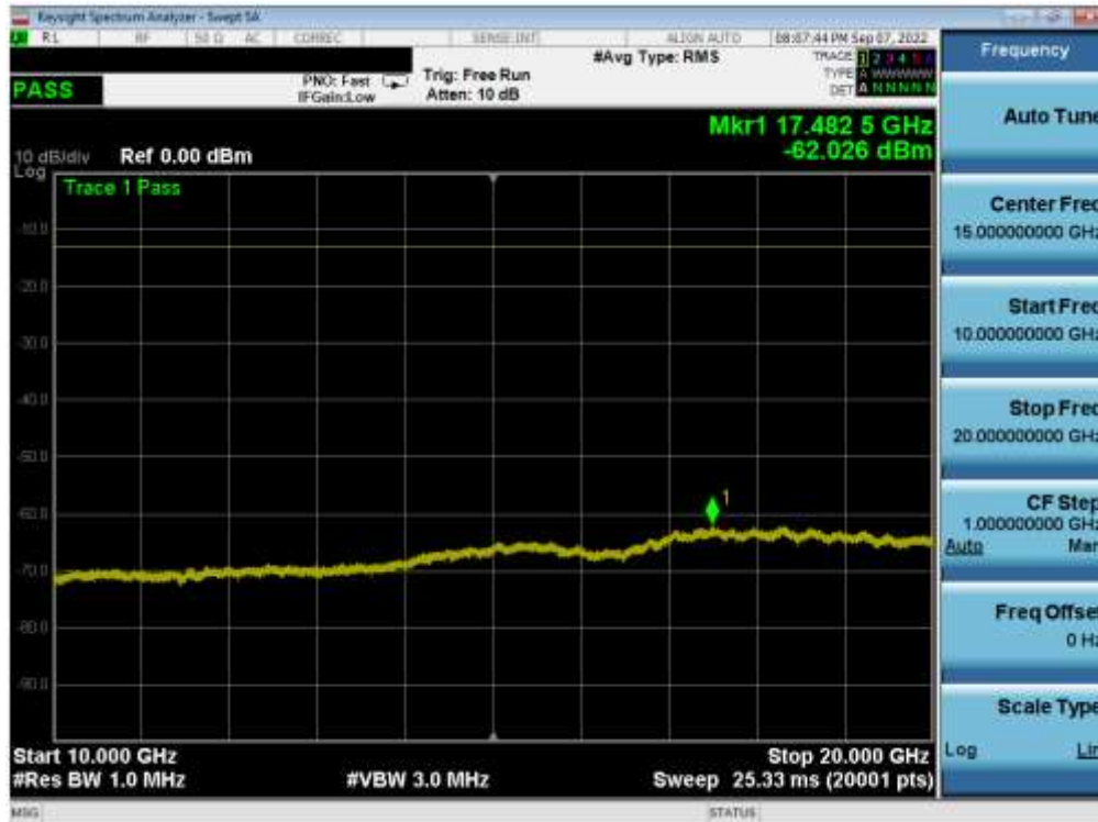
Plot 7-42. Conducted Spurious Plot (LTE Band 66/4 - 20MHz QPSK - 1 RB - Mid Channel)
