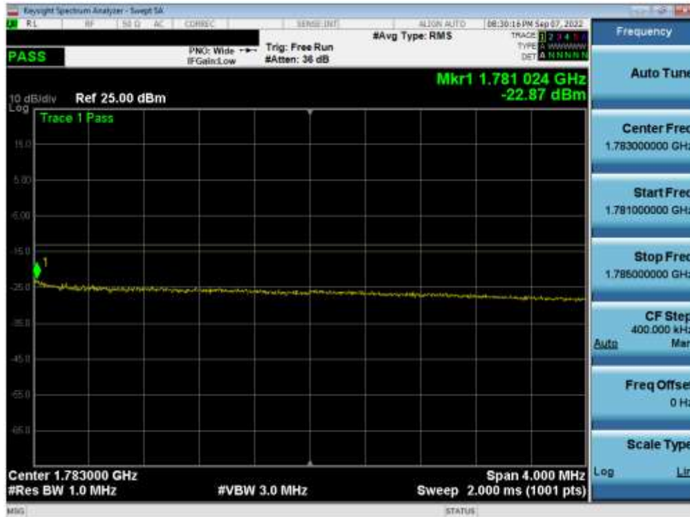
Plot 7-79. Upper Extended Band Edge Plot (LTE Band 66 - 10MHz QPSK – Full RB)
