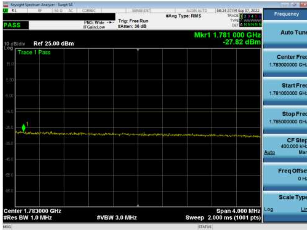
Plot 7-73. Upper Extended Band Edge Plot (LTE Band 66 - 15MHz QPSK – Full RB)
