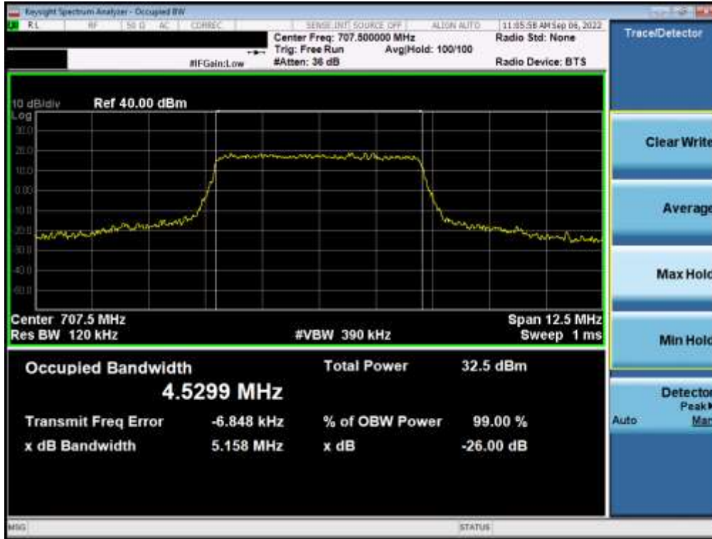
Plot 7-3. Occupied Bandwidth Plot (LTE Band 12 - 5MHz QPSK - Full RB)
