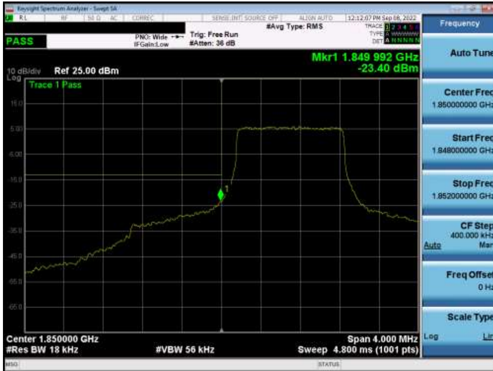
Plot 7-53. Lower Band Edge Plot (LTE Band 2 – 1.4MHz QPSK – Full RB)
