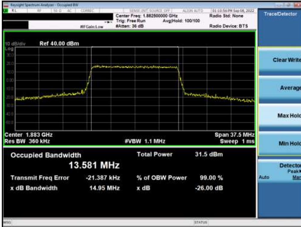
Plot 7-3. Occupied Bandwidth Plot (LTE Band 2 - 15MHz QPSK - Full RB)
