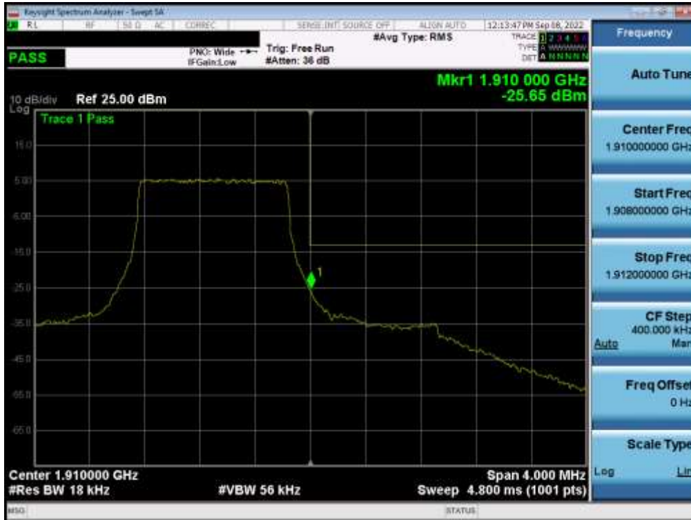
Plot 7-55. Upper Band Edge Plot (LTE Band 2 – 1.4MHz QPSK – Full RB)
