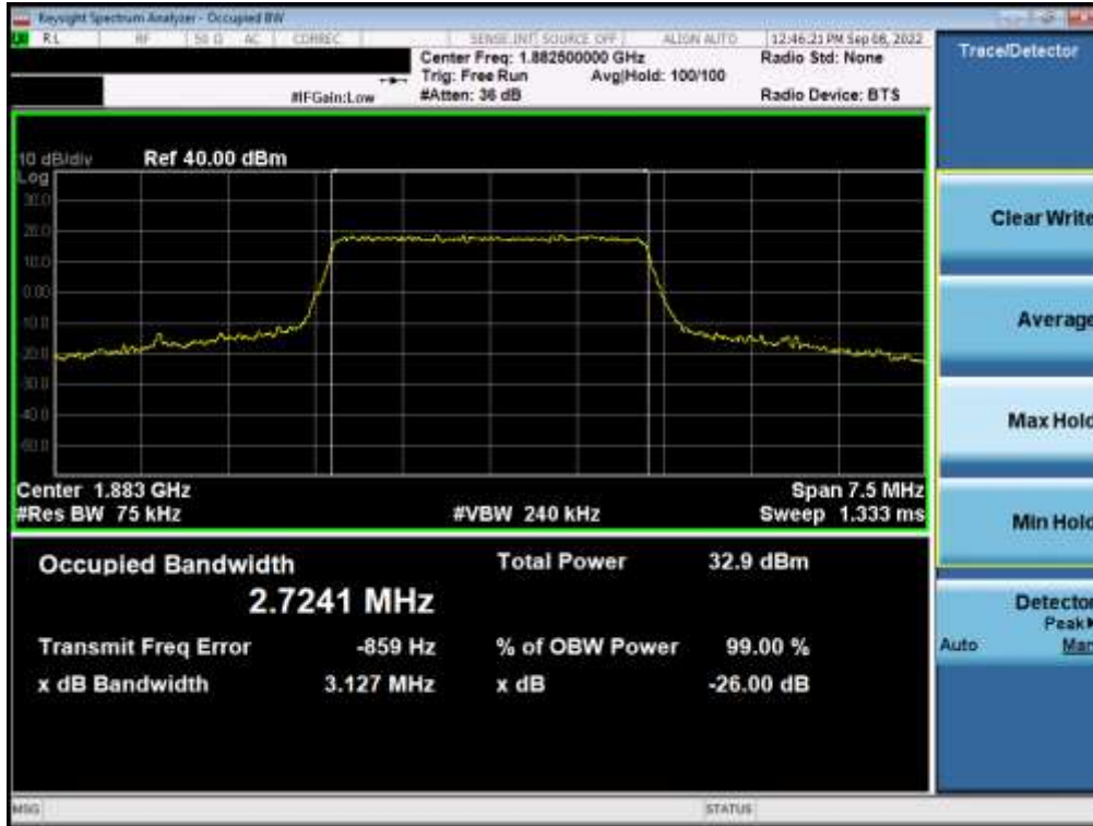
Plot 7-9. Occupied Bandwidth Plot (LTE Band 2 - 3MHz QPSK - Full RB)
