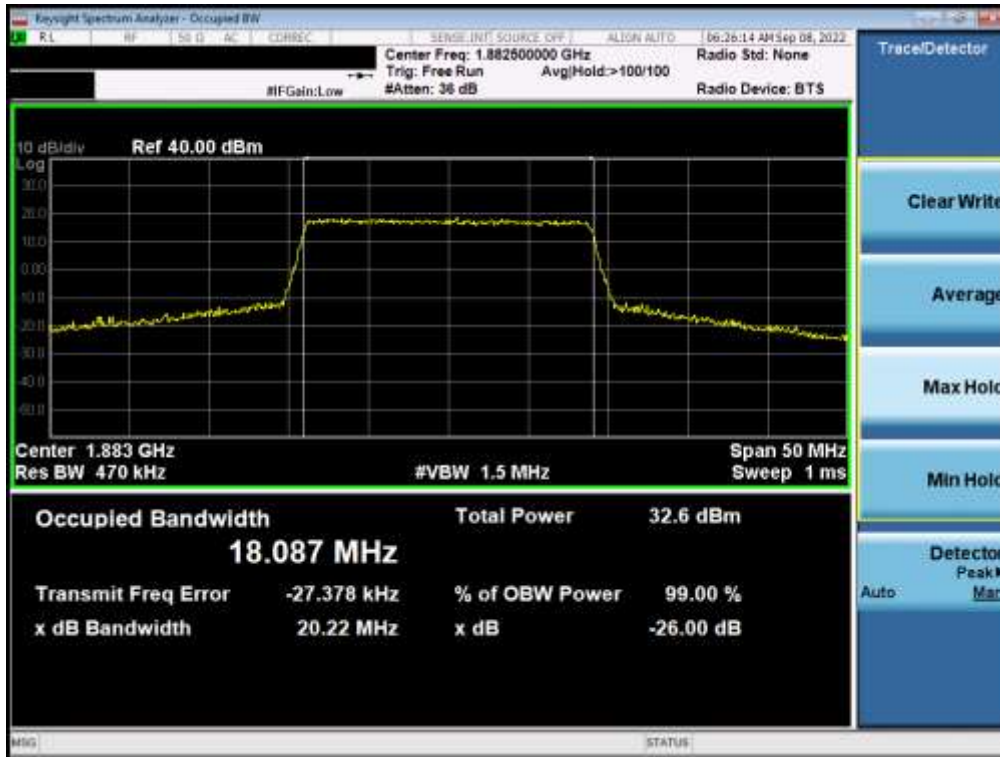
Plot 7-1. Occupied Bandwidth Plot (LTE Band 2 - 20MHz QPSK - Full RB)
