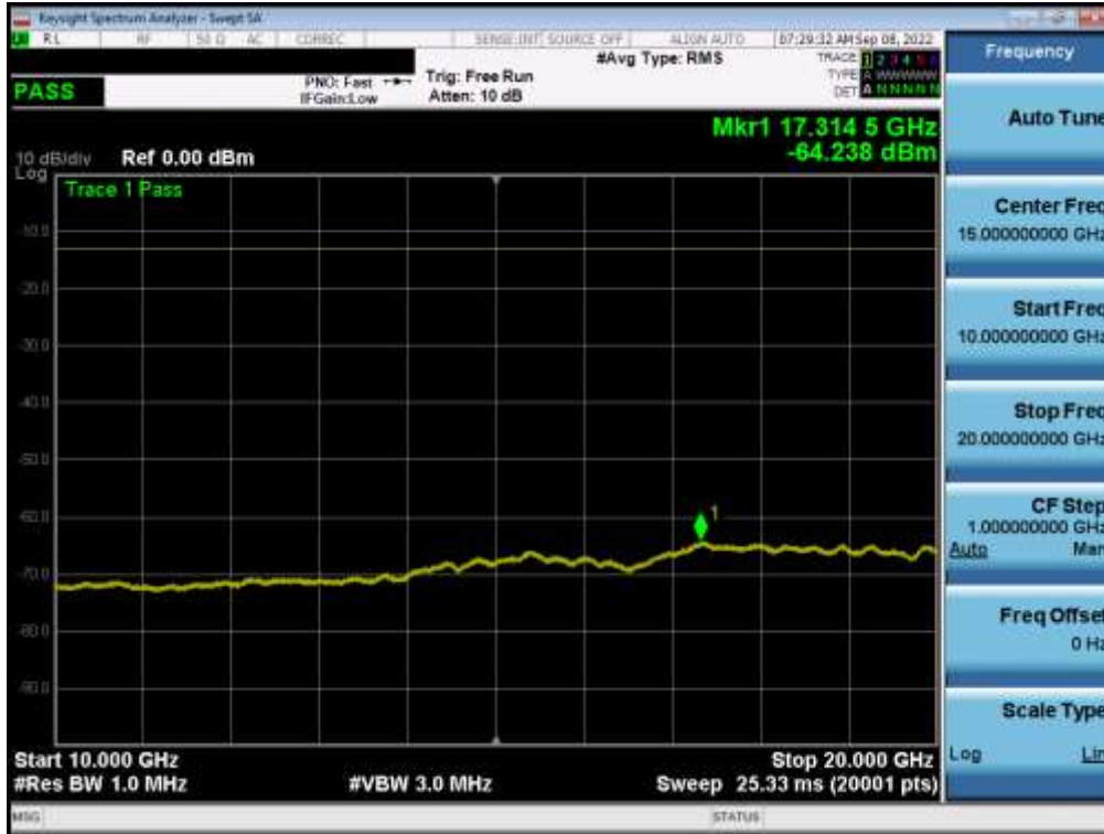
Plot 7-17. Conducted Spurious Plot (LTE Band 2 - 20MHz QPSK - 1RB - Low Channel)
