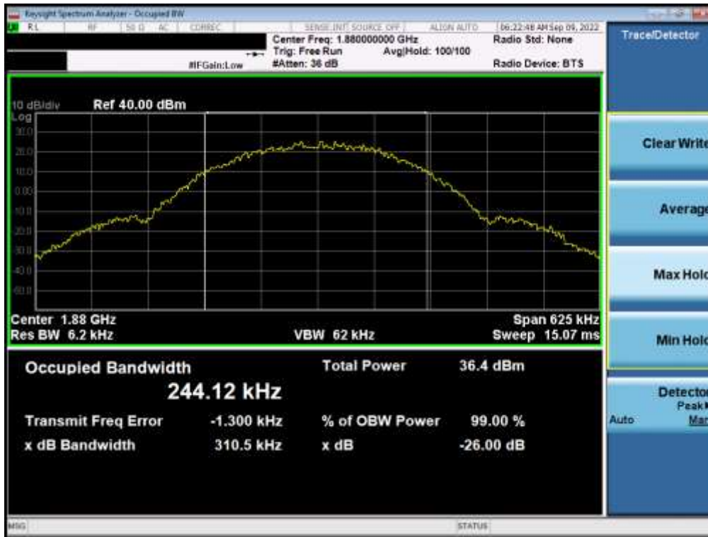
Plot 7-13. Occupied Bandwidth Plot (GPRS, Ch. 661)
