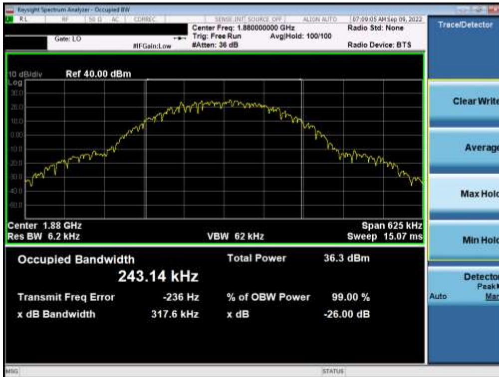
Plot 7-14. Occupied Bandwidth Plot (EDGE, Ch. 661)
