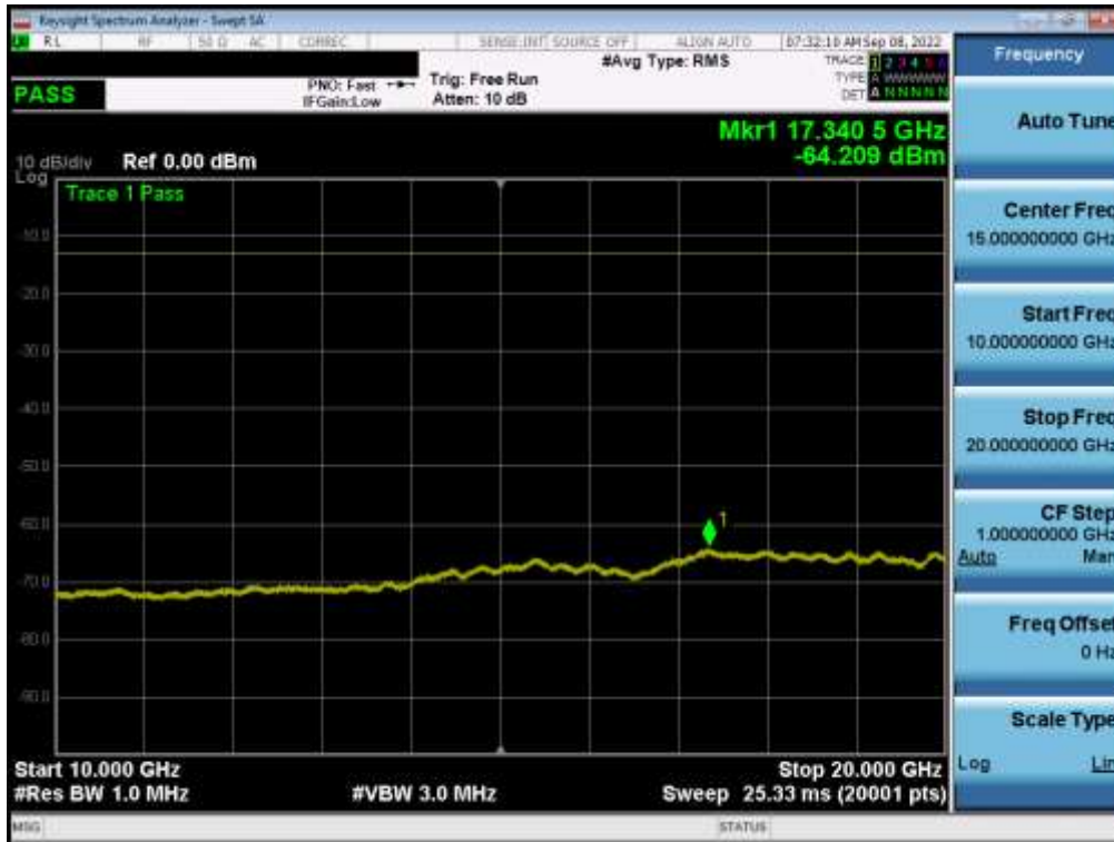
Plot 7-20. Conducted Spurious Plot (LTE Band 2 - 20MHz QPSK - 1RB - Mid Channel)
