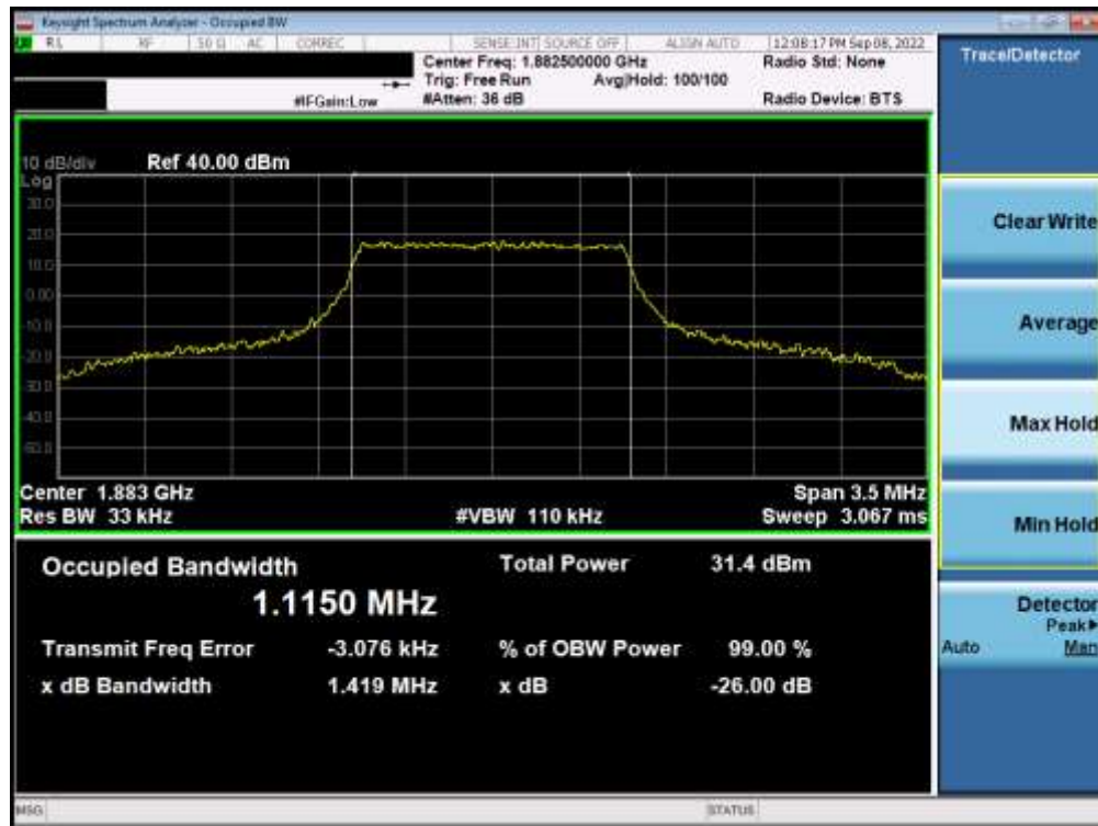
Plot 7-12. Occupied Bandwidth Plot (LTE Band 2 - 1.4MHz 16-QAM - Full RB)
