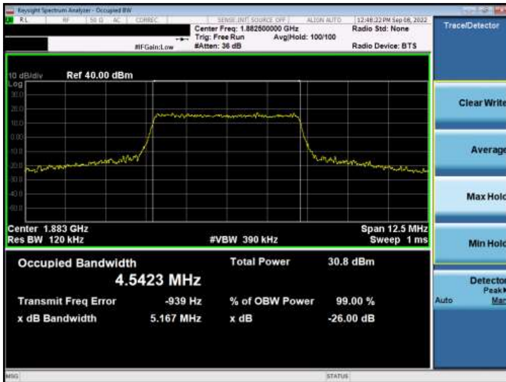
Plot 7-8. Occupied Bandwidth Plot (LTE Band 2 - 5MHz 16-QAM - Full RB)
