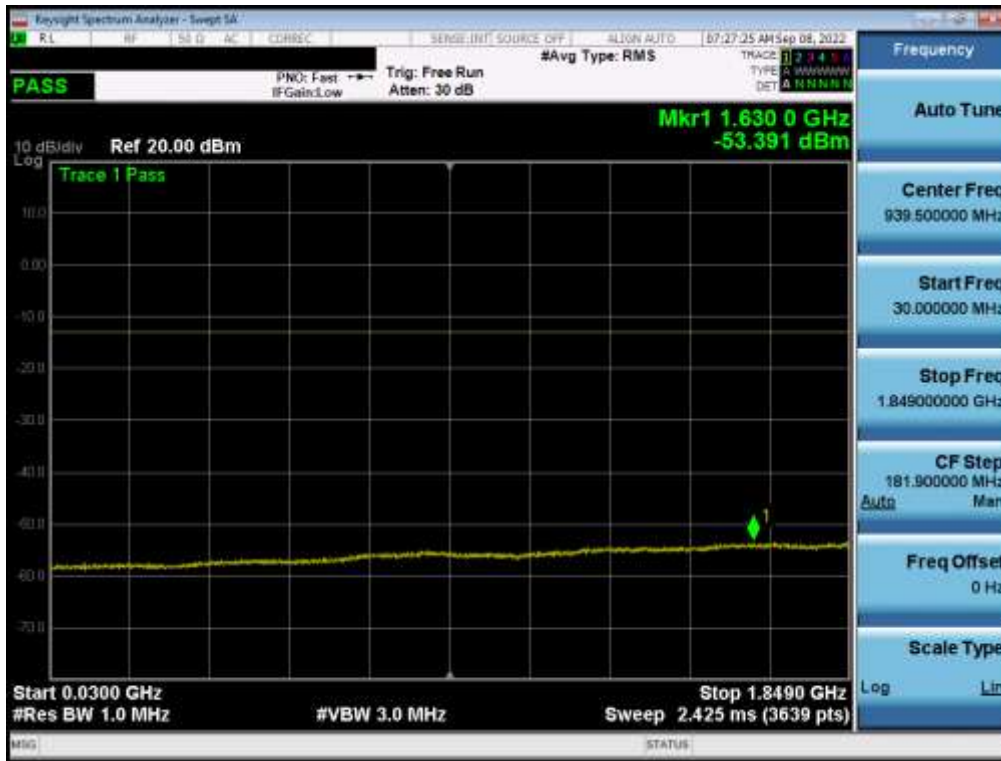
Plot 7-15. Conducted Spurious Plot (LTE Band 2 - 20MHz QPSK - 1RB - Low Channel)
