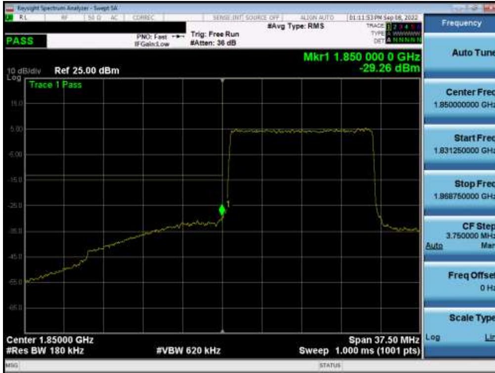
Plot 7-37. Lower Band Edge Plot (LTE Band 2 - 15MHz QPSK – Full RB)
