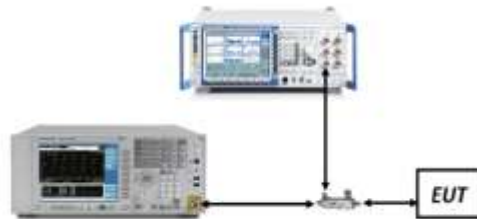
Figure 7-4. Test Instrument & Measurement Setup
