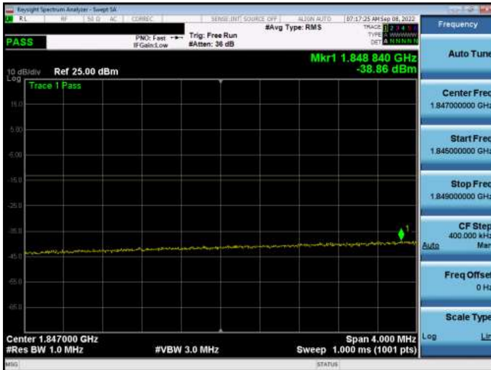
Plot 7-34. Extended Lower Band Edge Plot (LTE Band 2 - 20MHz QPSK – Full RB)
