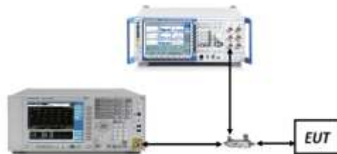
Figure 7-2. Test Instrument & Measurement Setup
