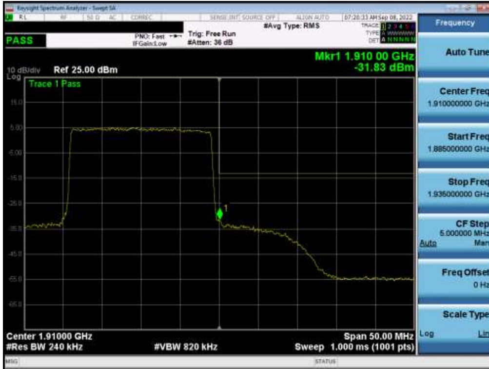
Plot 7-35. Upper Band Edge Plot (LTE Band 2 - 20MHz QPSK – Full RB)
