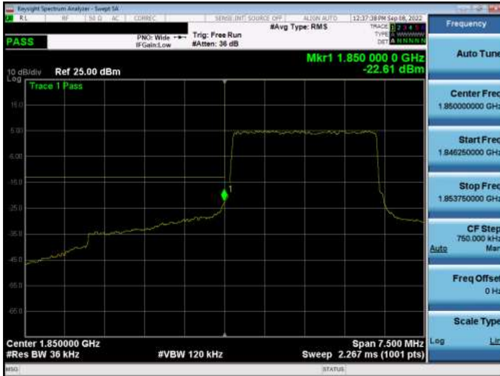
Plot 7-49. Lower Band Edge Plot (LTE Band 2 - 3MHz QPSK – Full RB)
