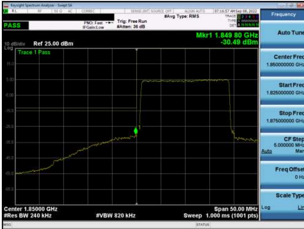
Plot 7-33. Lower Band Edge Plot (LTE Band 2 - 20MHz QPSK – Full RB)
