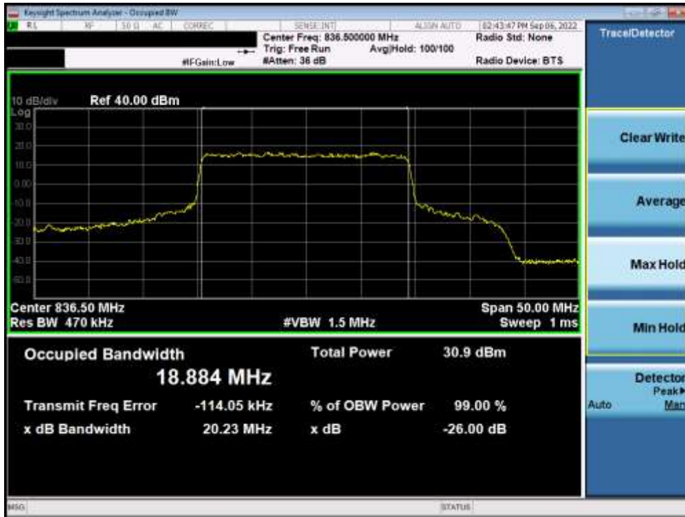
Plot 7-12. Occupied Bandwidth Plot (NR Band n5 - 20MHz QPSK - Full RB)
