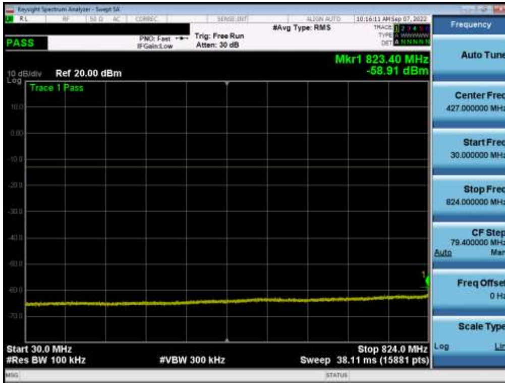
Plot 7-59. Conducted Spurious Plot (WCDMA Ch. 4233)
