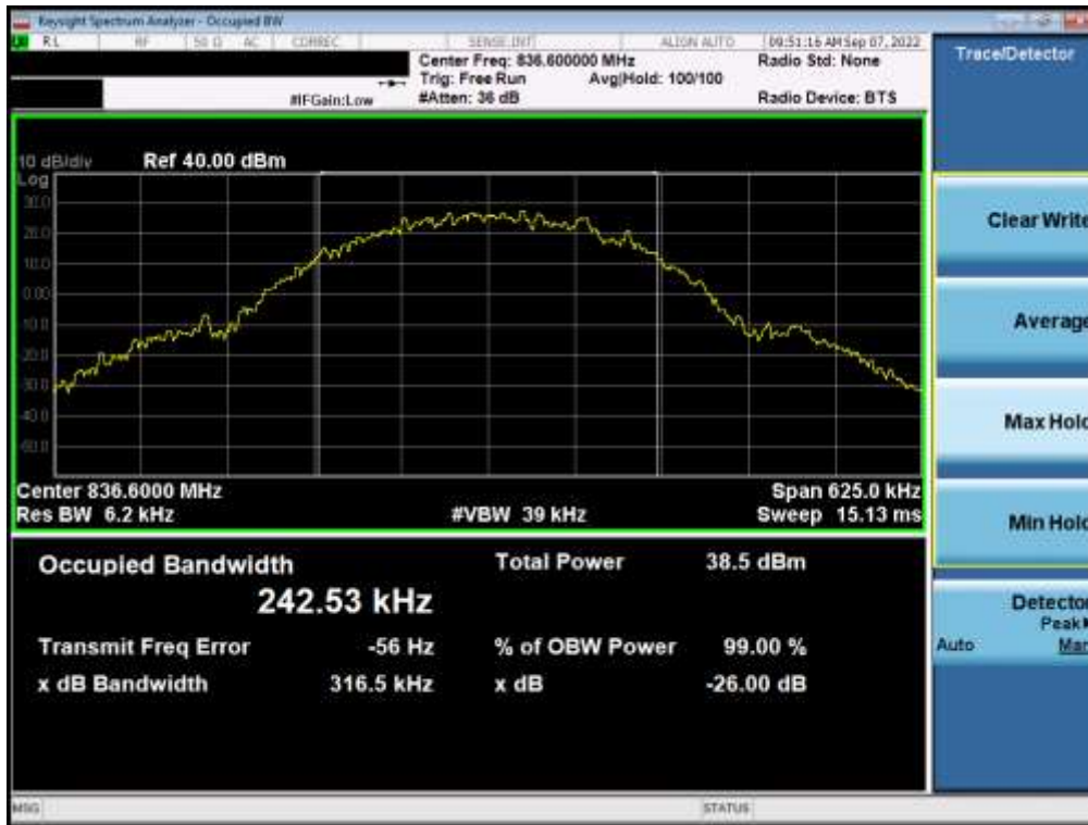
Plot 7-23. Occupied Bandwidth Plot (GPRS, Ch. 190)
