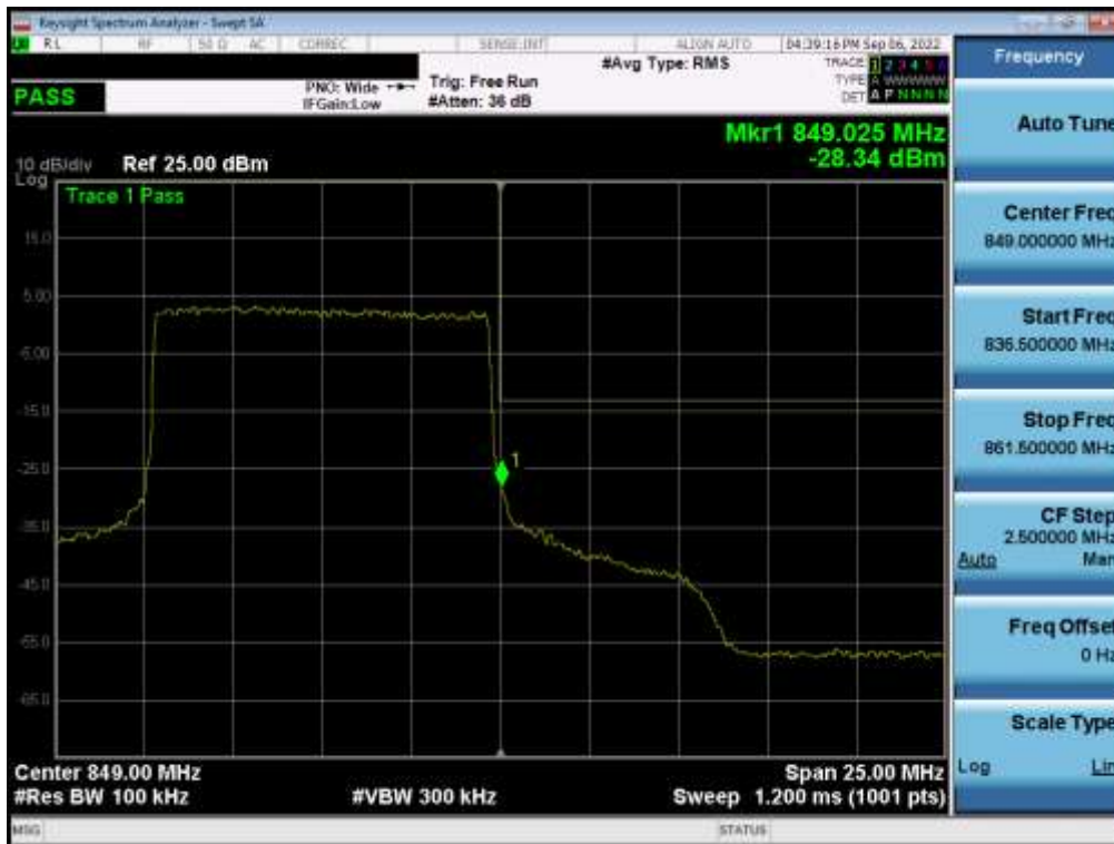
Plot 7-77. Upper Band Edge Plot (NR Band n5 – 10.0MHz - Full RB)
