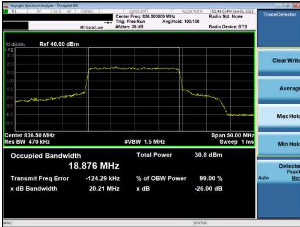
Plot 7-13. Occupied Bandwidth Plot (NR Band n5 - 20MHz 16-QAM - Full RB)
