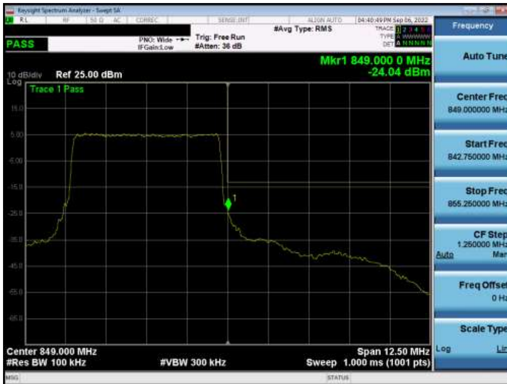
Plot 7-79. Upper Band Edge Plot (NR Band n5 – 5.0MHz - Full RB)
