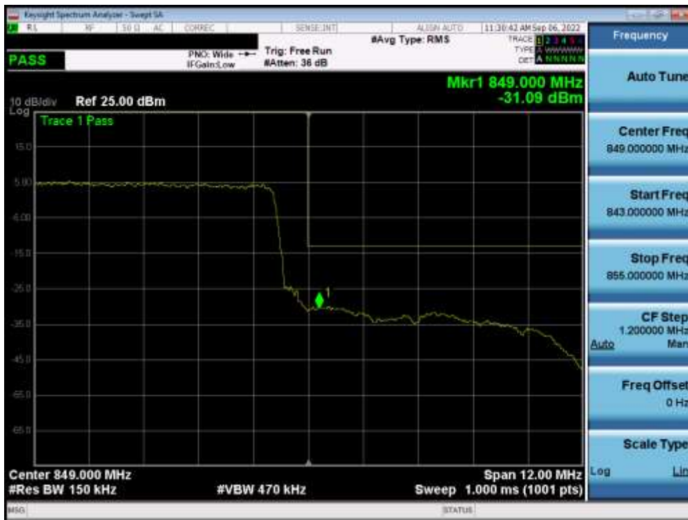
Plot 7-63. Upper Band Edge Plot (LTE Band 26 - 15MHz QPSK – Full RB)
