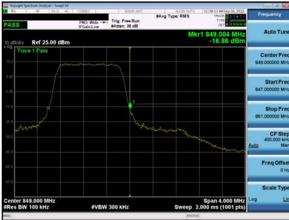
Plot 7-71. Upper Band Edge Plot (LTE Band 26/5 – 1.4MHz QPSK – Full RB)
