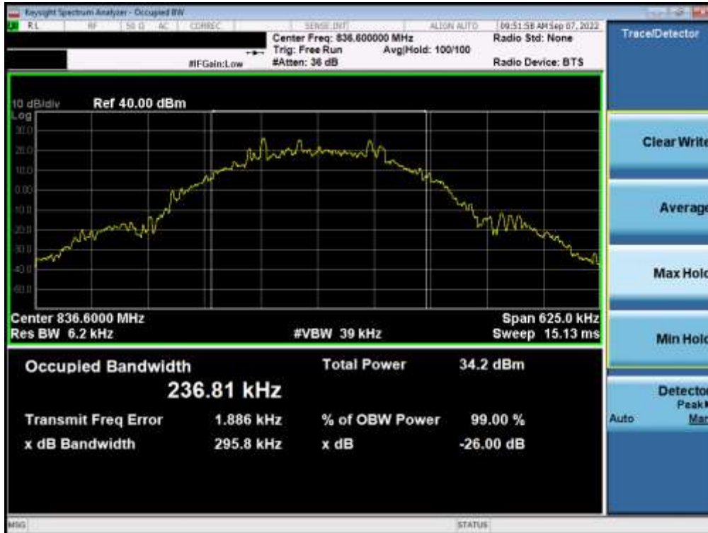
Plot 7-24. Occupied Bandwidth Plot (EDGE, Ch. 190)
