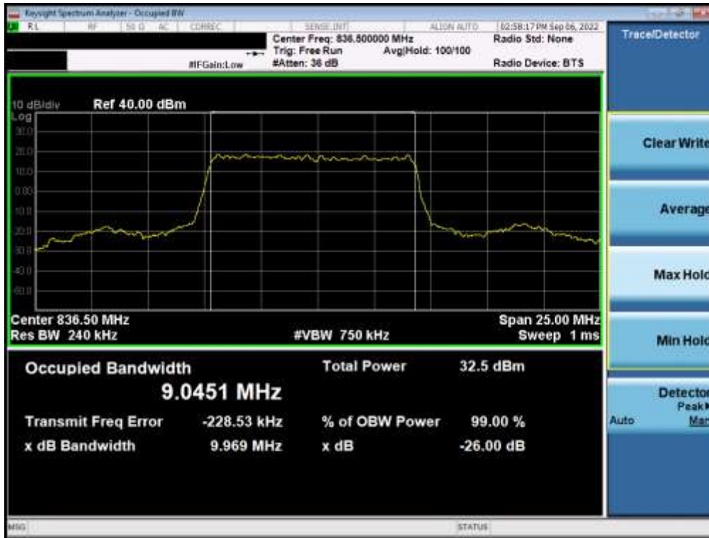
Plot 7-17. Occupied Bandwidth Plot (NR Band n5 - 10MHz \pi/2 BPSK - Full RB)
