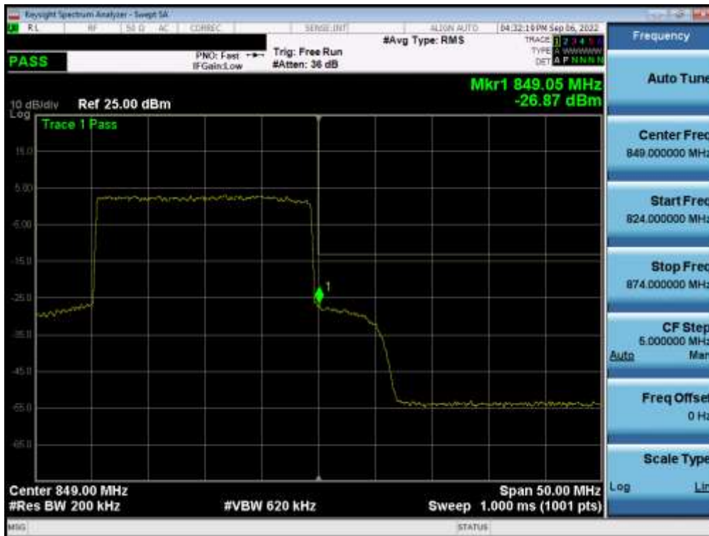
Plot 7-73. Upper Band Edge Plot (NR Band n5 – 20.0MHz - Full RB)
