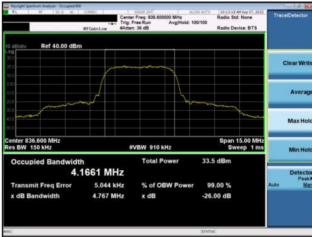
Plot 7-25. Occupied Bandwidth Plot (WCDMA, Ch. 4183)
