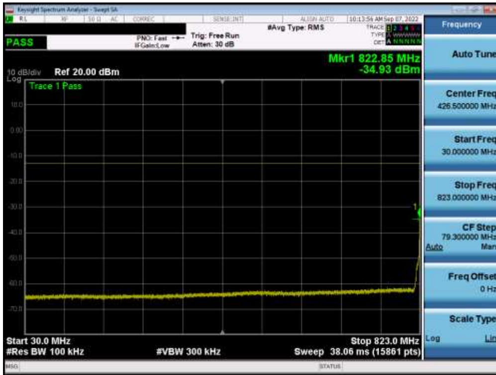
Plot 7-53. Conducted Spurious Plot (WCDMA Ch. 4132)
