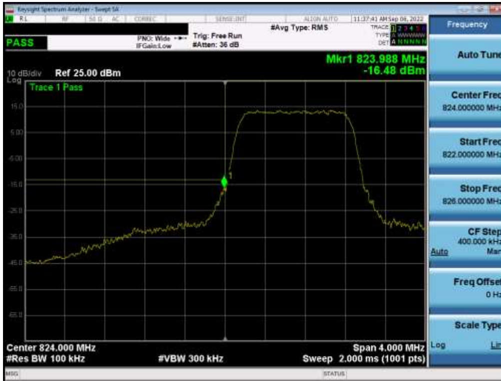
Plot 7-70. Lower Band Edge Plot (LTE Band 26/5 – 1.4MHz QPSK – Full RB)
