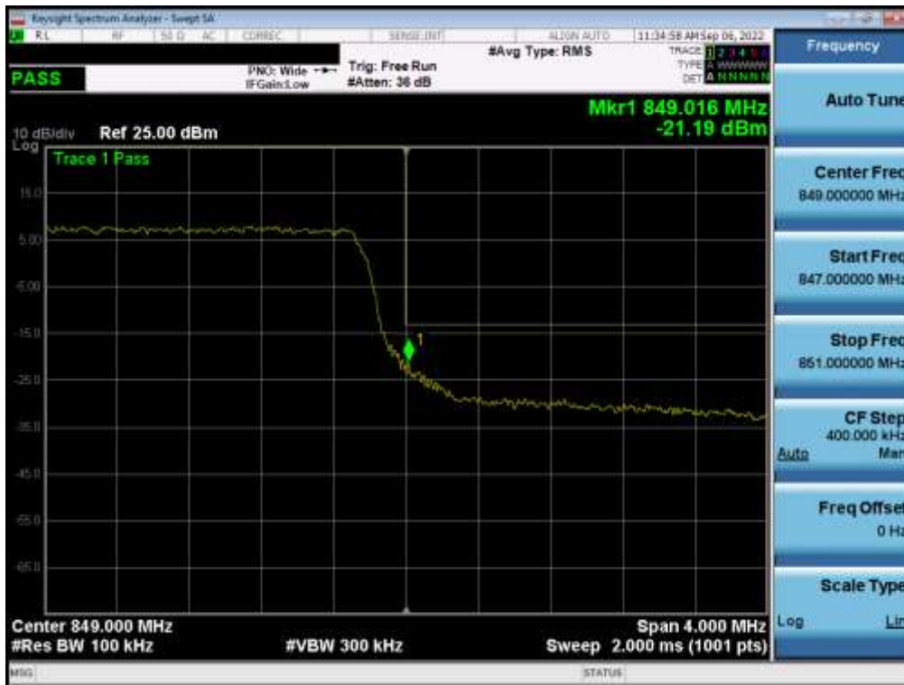
Plot 7-67. Upper Band Edge Plot (LTE Band 26/5 - 5MHz QPSK – Full RB)
