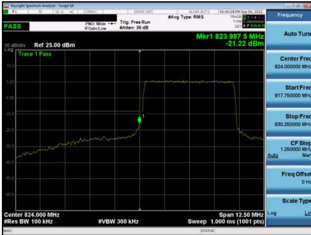
Plot 7-78. Lower Band Edge Plot (NR Band n5 – 5.0MHz - Full RB)
