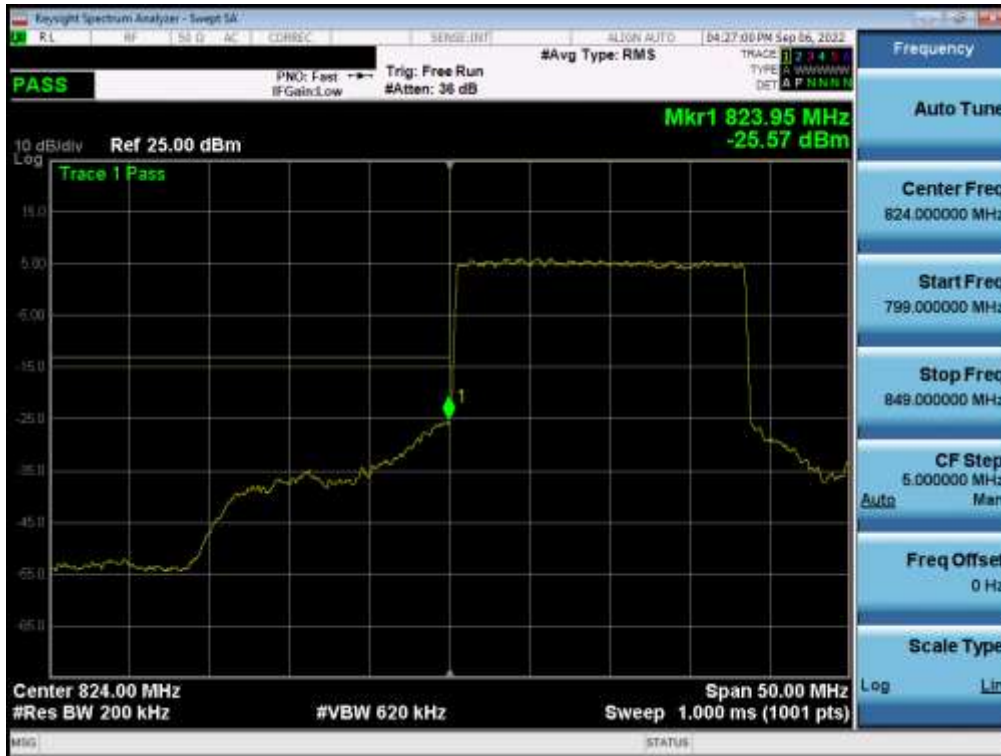
Plot 7-72. Lower Band Edge Plot (NR Band n5 – 20.0MHz - Full RB)
