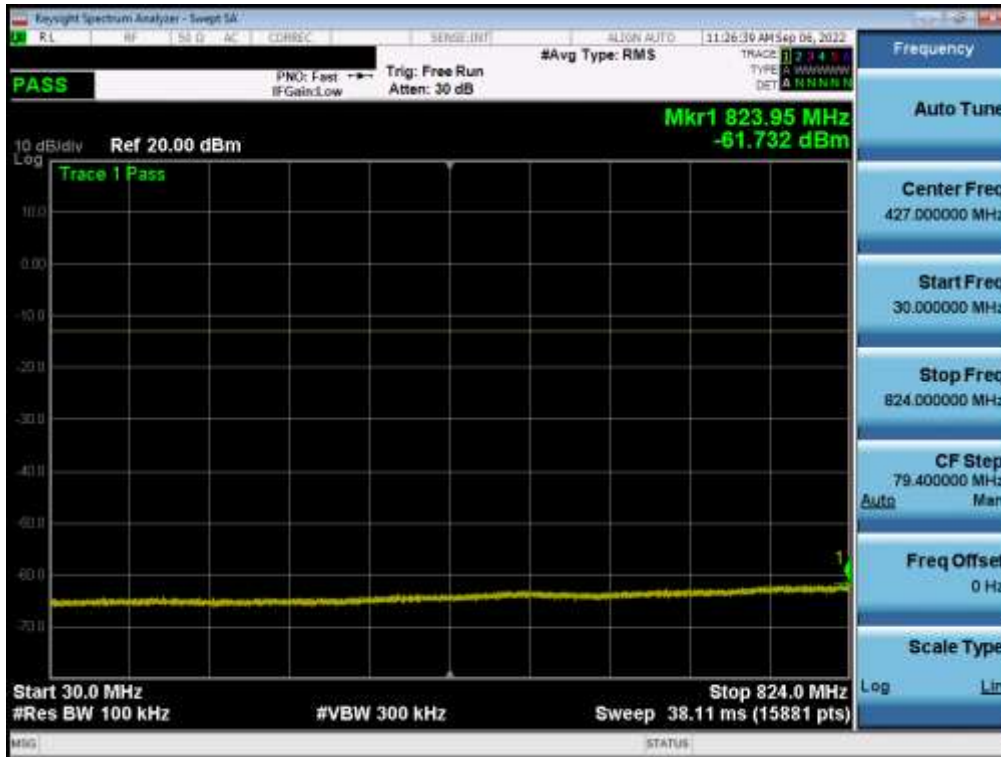
Plot 7-32. Conducted Spurious Plot (LTE Band 26/5 - 10MHz QPSK - 1 RB - High Channel)
