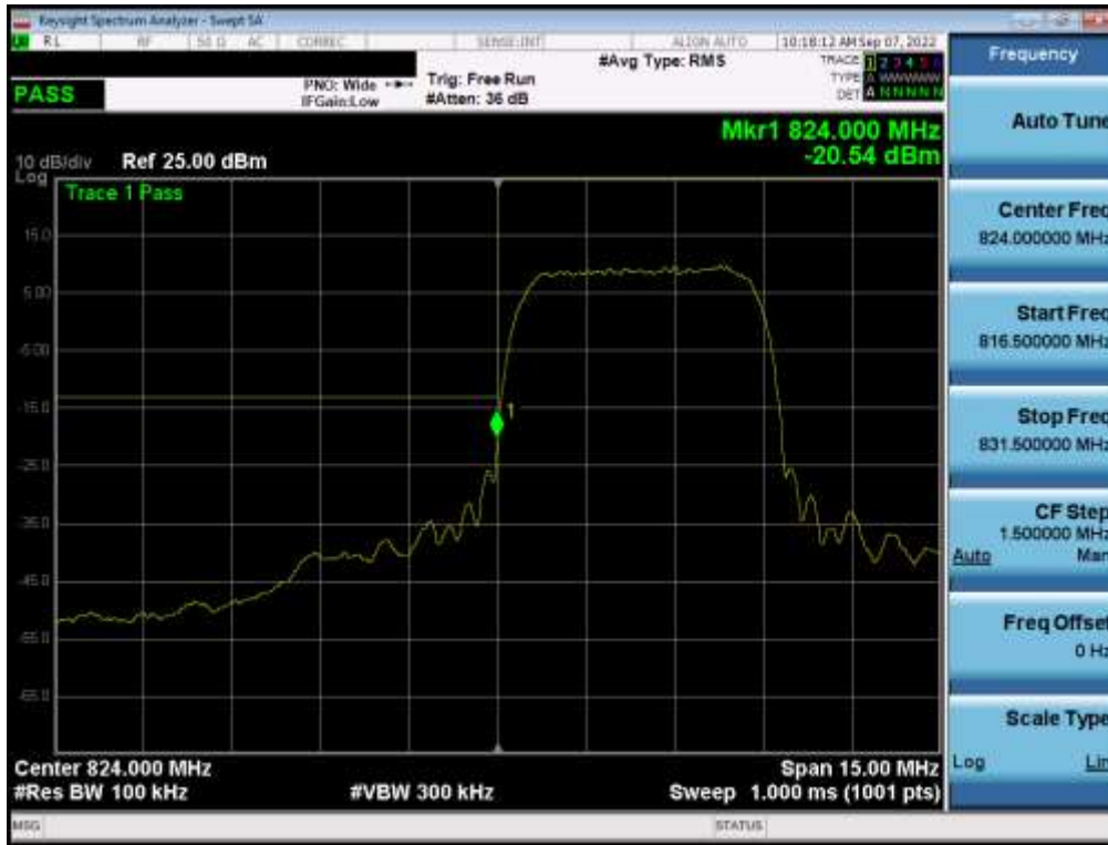
Plot 7-82. Lower Band Edge Plot (WCDMA Cell – Ch. 4132)
