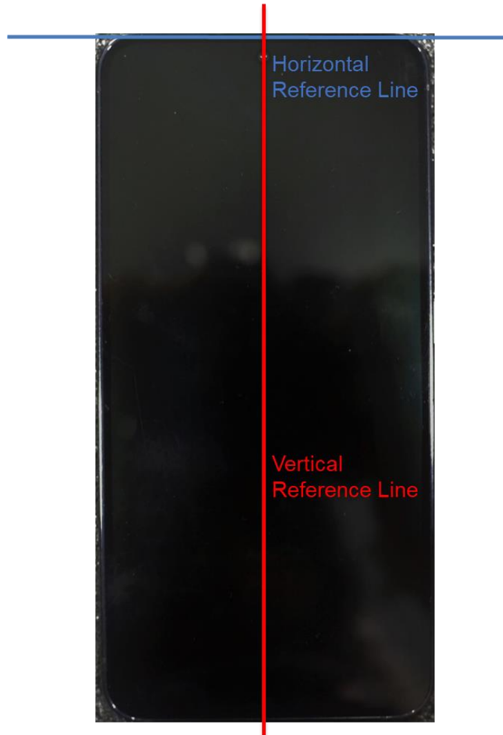
SAR Test Setup Photo 18 – Reference Lines
