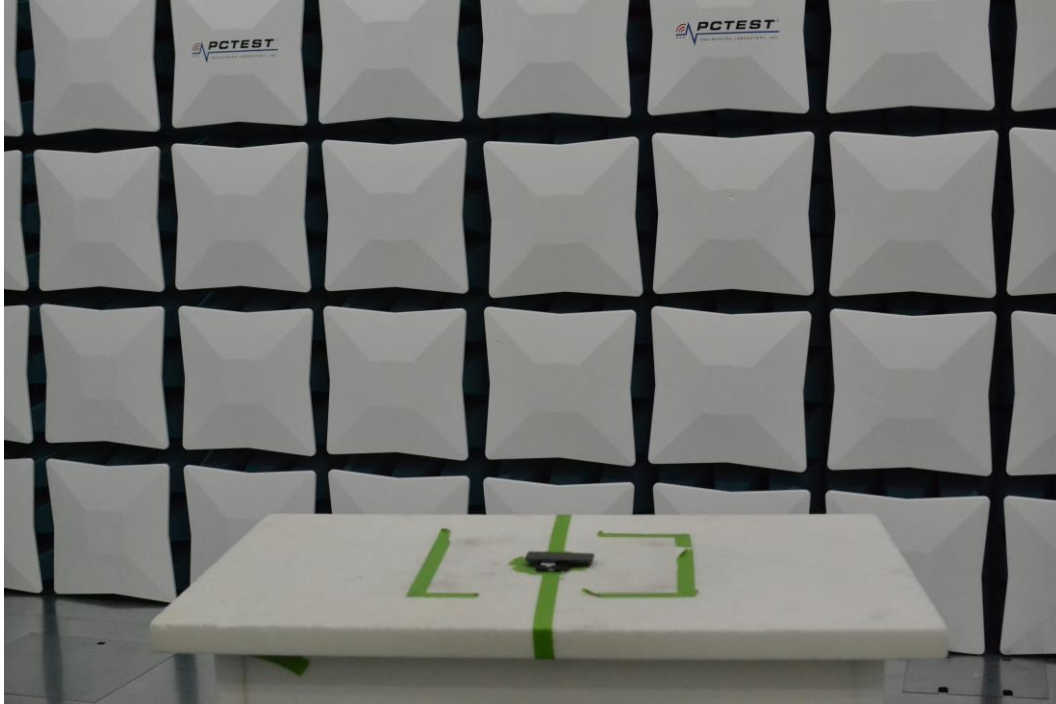
Figure 25. Test Setup – WPT Position – 30Hz-1GHz
