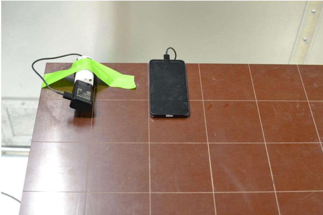
Figure 2. Test Setup – ACLC– <30MHz
