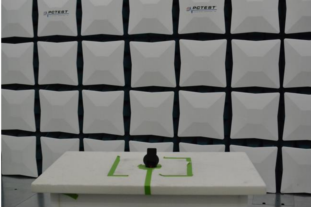
Figure 21. Test Setup – WCP Position – 30MHz-1GHz
