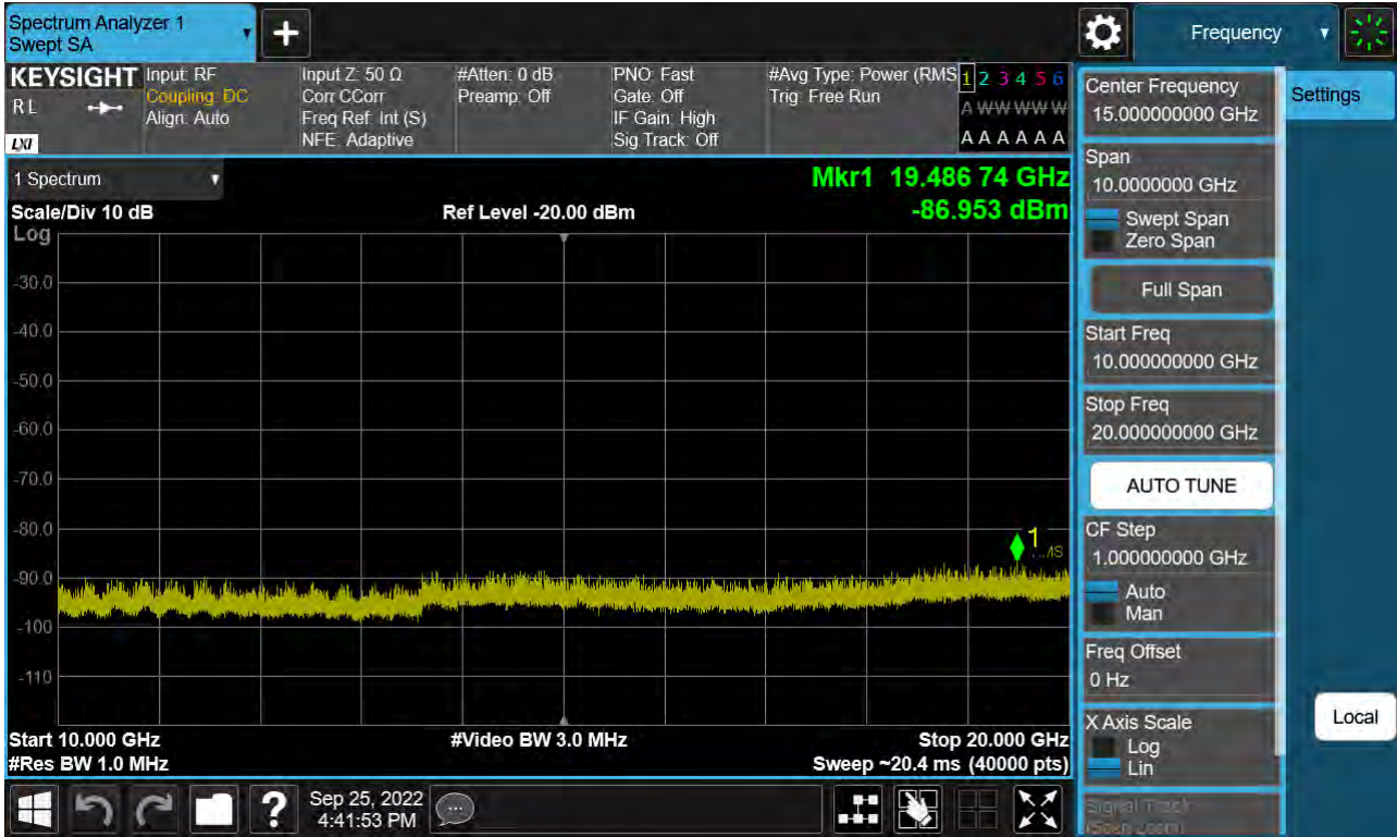
Sub6 n66. Conducted Spurious Plot_2 (343000ch_10 MHz_BPSK_RB 1_1)
