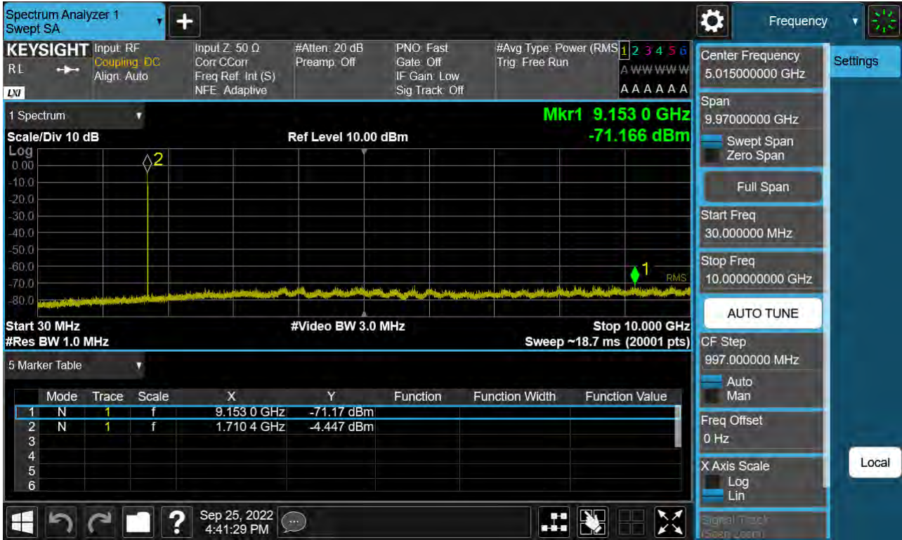
Sub6 n66. Conducted Spurious Plot_1 (343000ch_10 MHz_BPSK_RB 1_1)
