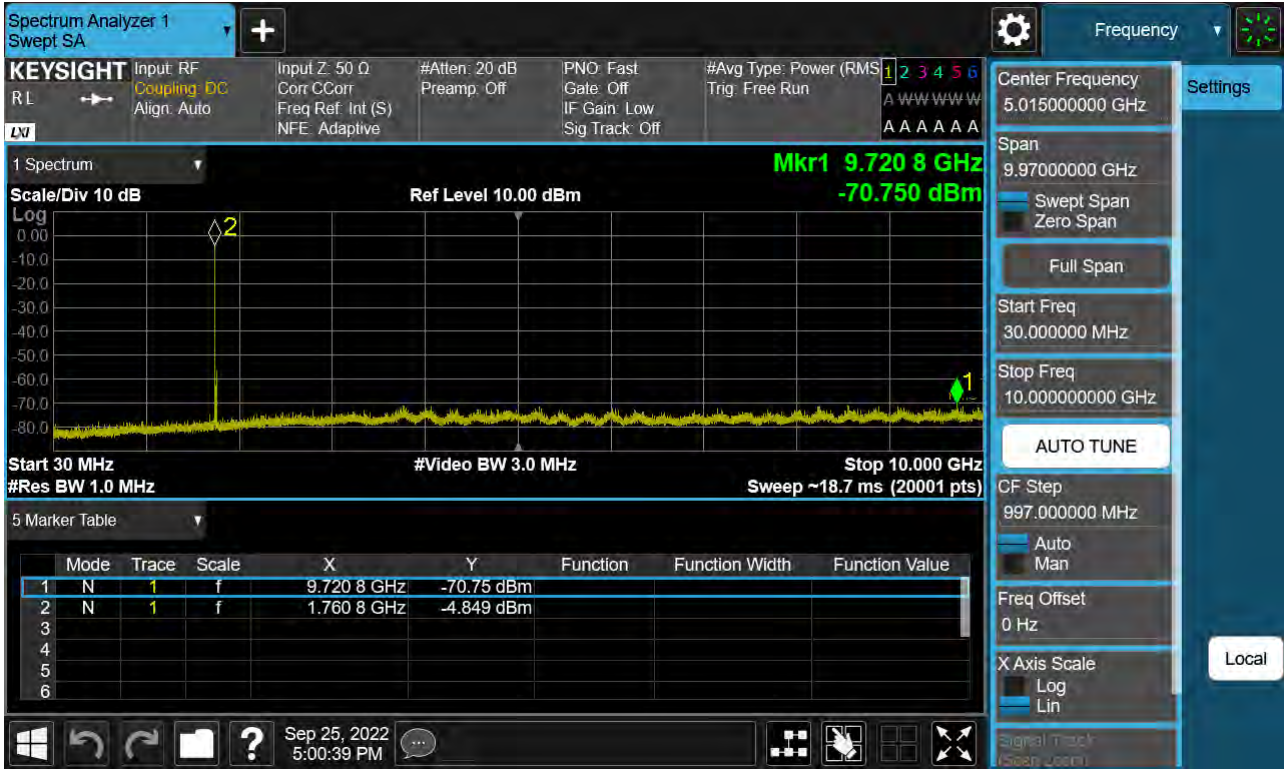
Sub6 n66. Conducted Spurious Plot_1 (354000ch_20 MHz_BPSK_ RB 1_1)
