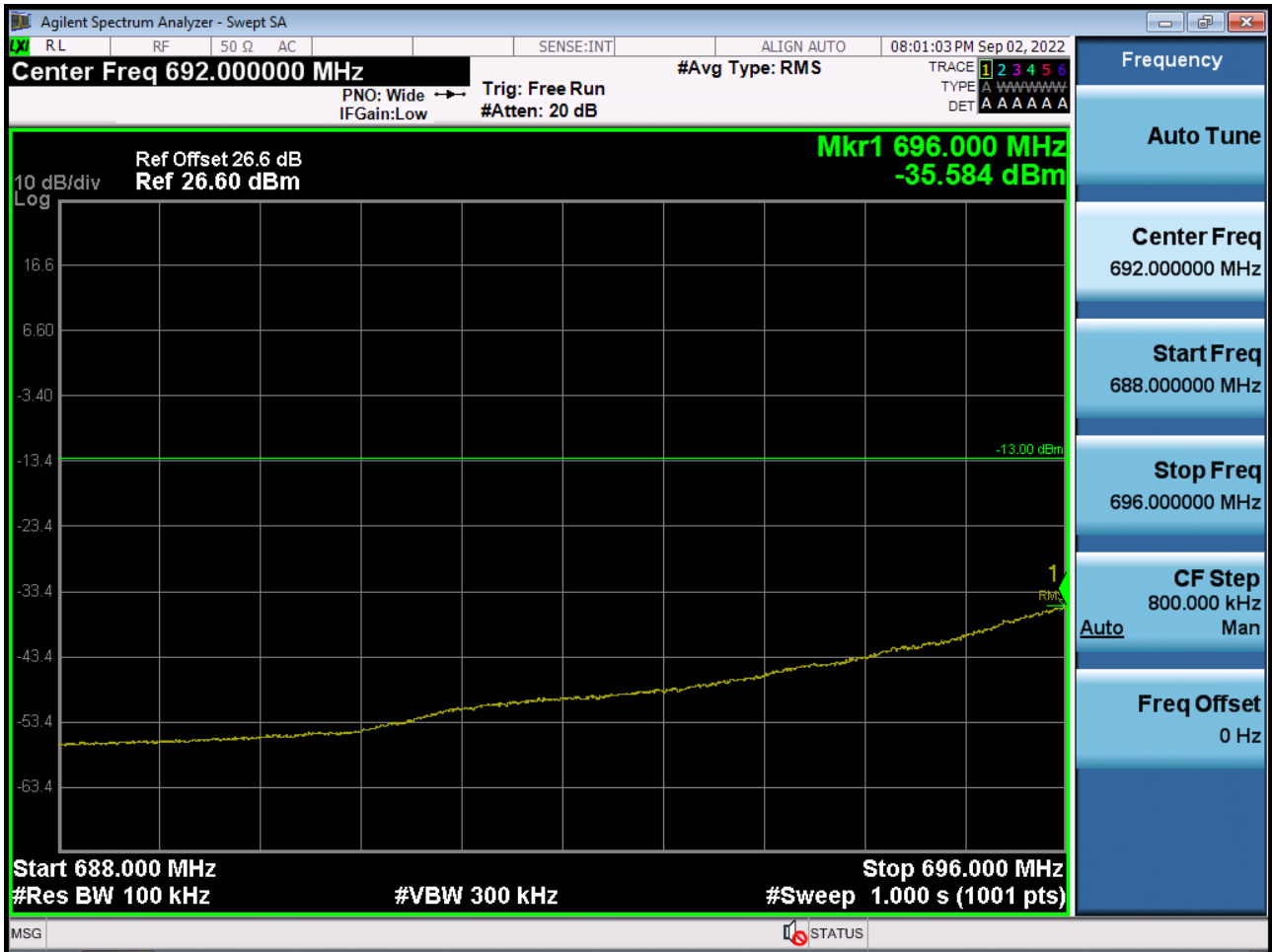
BAND 12/17. Lower Extended Band Edge Plot (5 M BW Ch.23035 QPSK_RB25_0)
