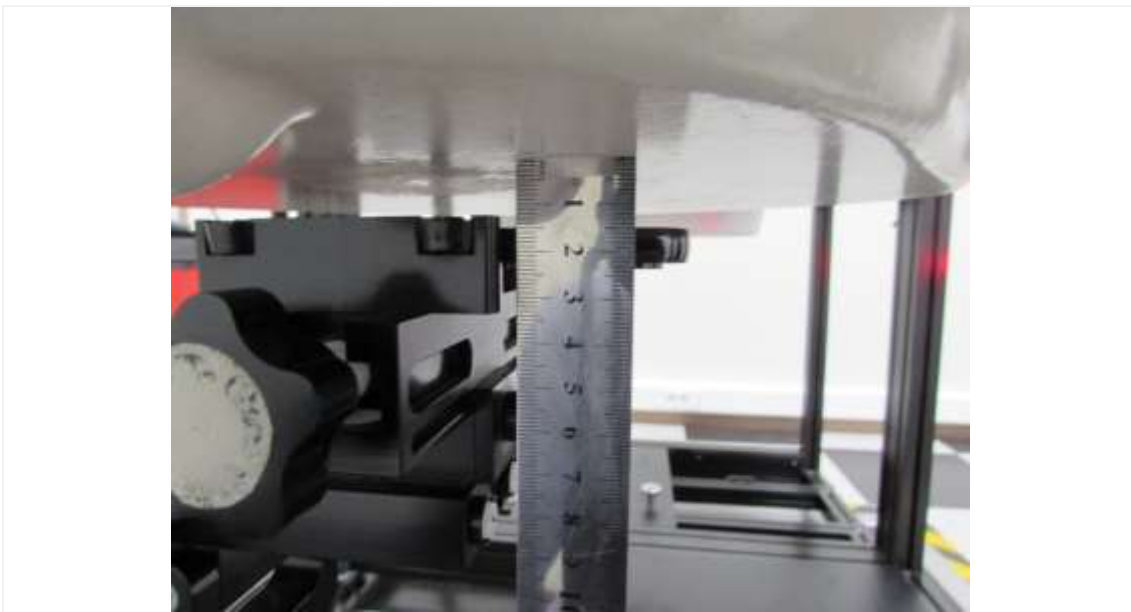
Distance of 15 mm from the EUT
