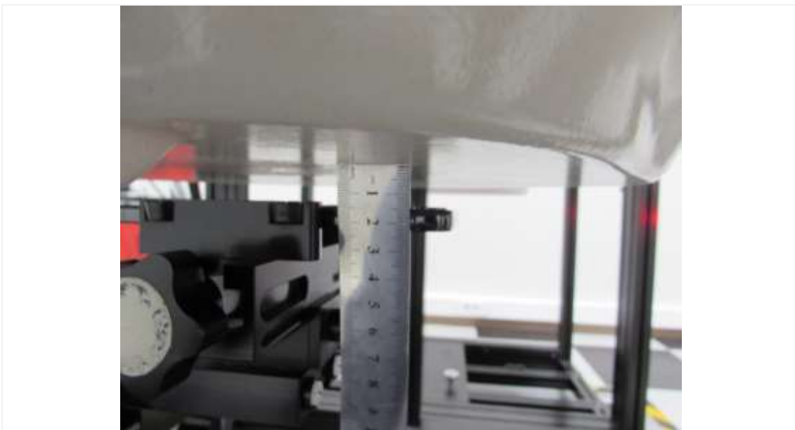
Distance of 15 mm from the EUT
