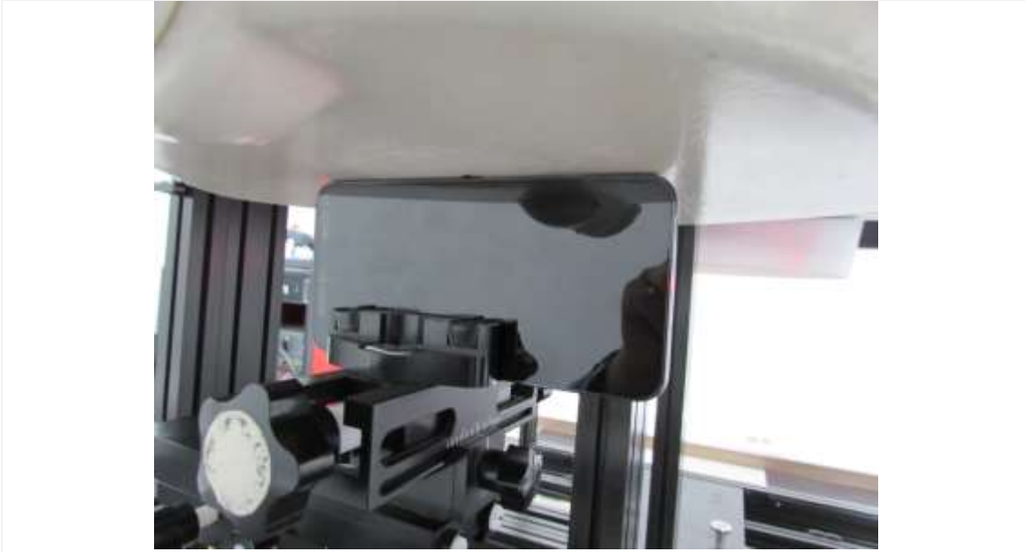
Distance of 0 mm from the EUT
