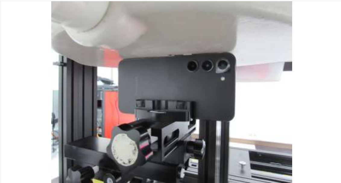
Distance of 0 mm from the EUT
