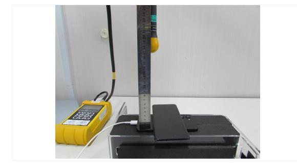
Top + TA : 20 cm (The distance between the DUT and the center of the probe is 15 cm.)
