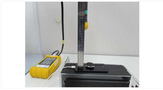
**Top + TA : 20 cm** (The distance between the DUT and the center of the probe is 20 cm.)
