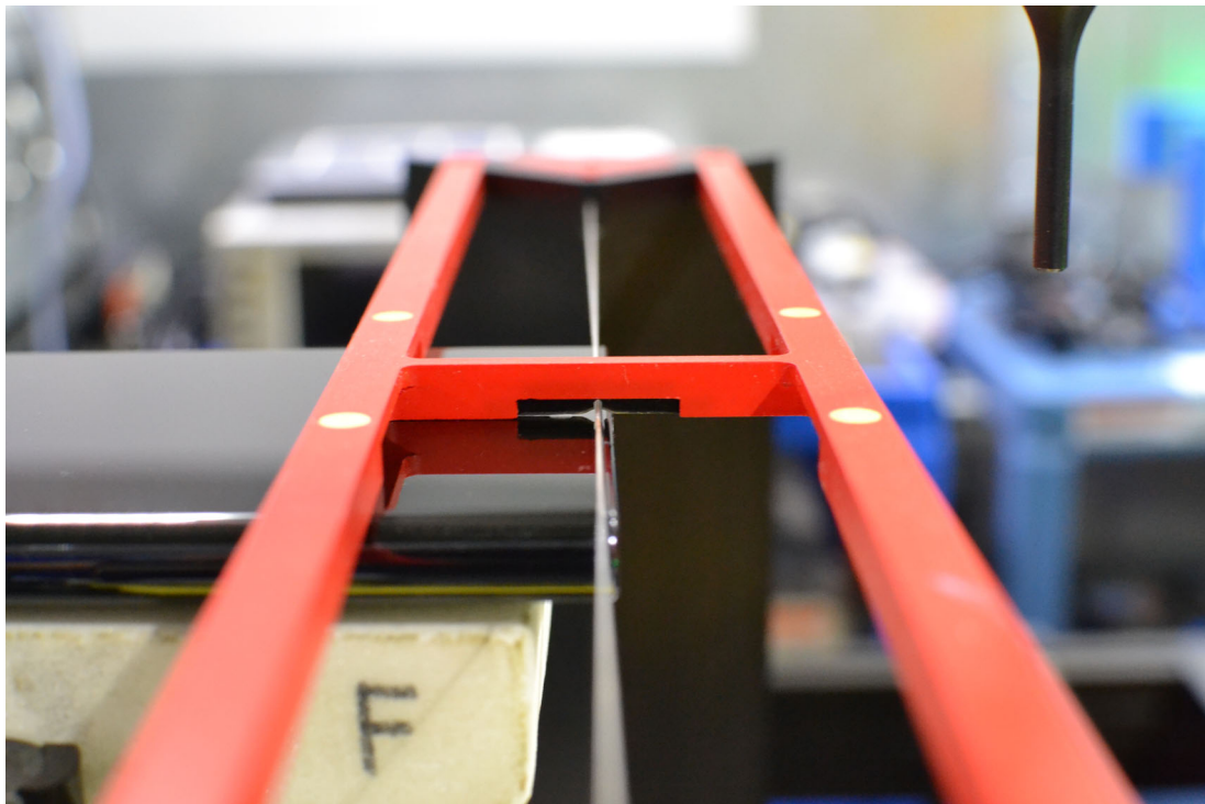
Figure 17-2 HAC Phantom Plane Alignment
