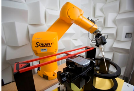
Figure 4-3 SPEAG Robotic System
