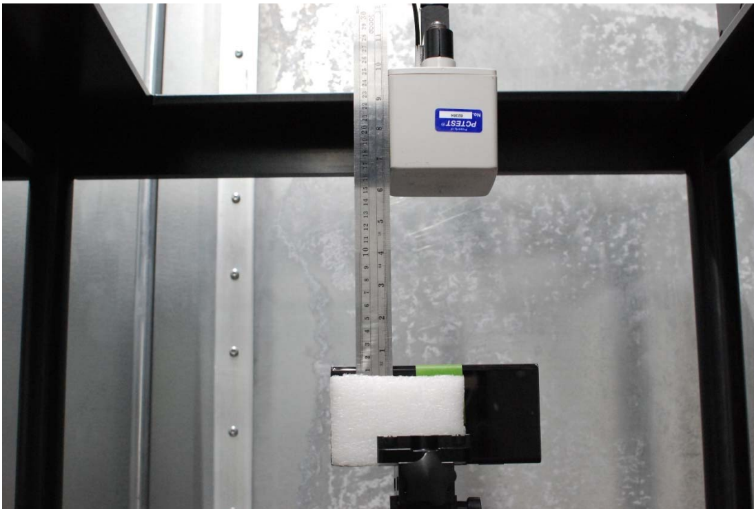
Test Setup Photo 24 H-field, Left edge, 15cm
