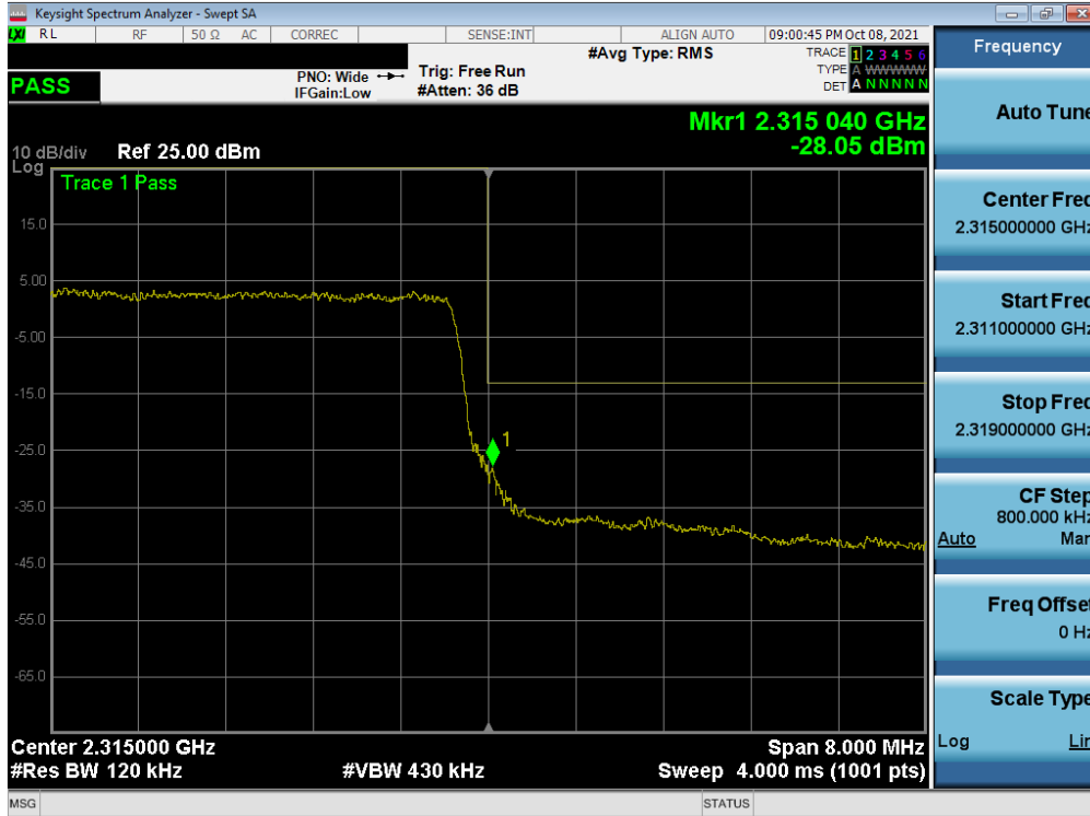
Plot 7-249. Upper Band Edge Plot (NR Band n30 - 10MHz CP-OFDM-QPSK – Full RB - Ant A)
