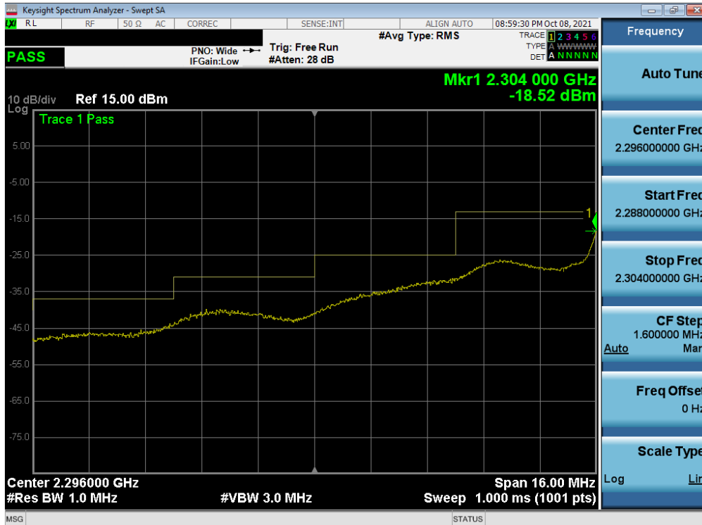
Plot 7-248. Extended Lower Band Edge Plot (NR Band n30 - 10MHz CP-OFDM-QPSK – Full RB - Ant A)
