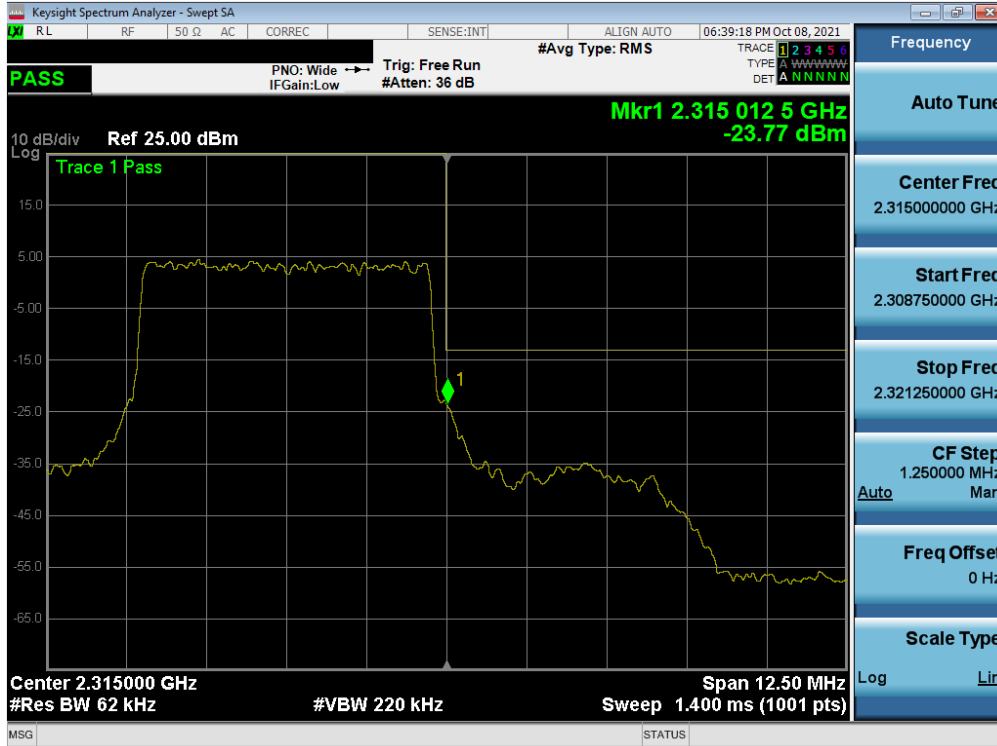
Plot 7-261. Upper Band Edge Plot (NR Band n30 - 5MHz CP-OFDM-QPSK – Full RB - Ant J)
