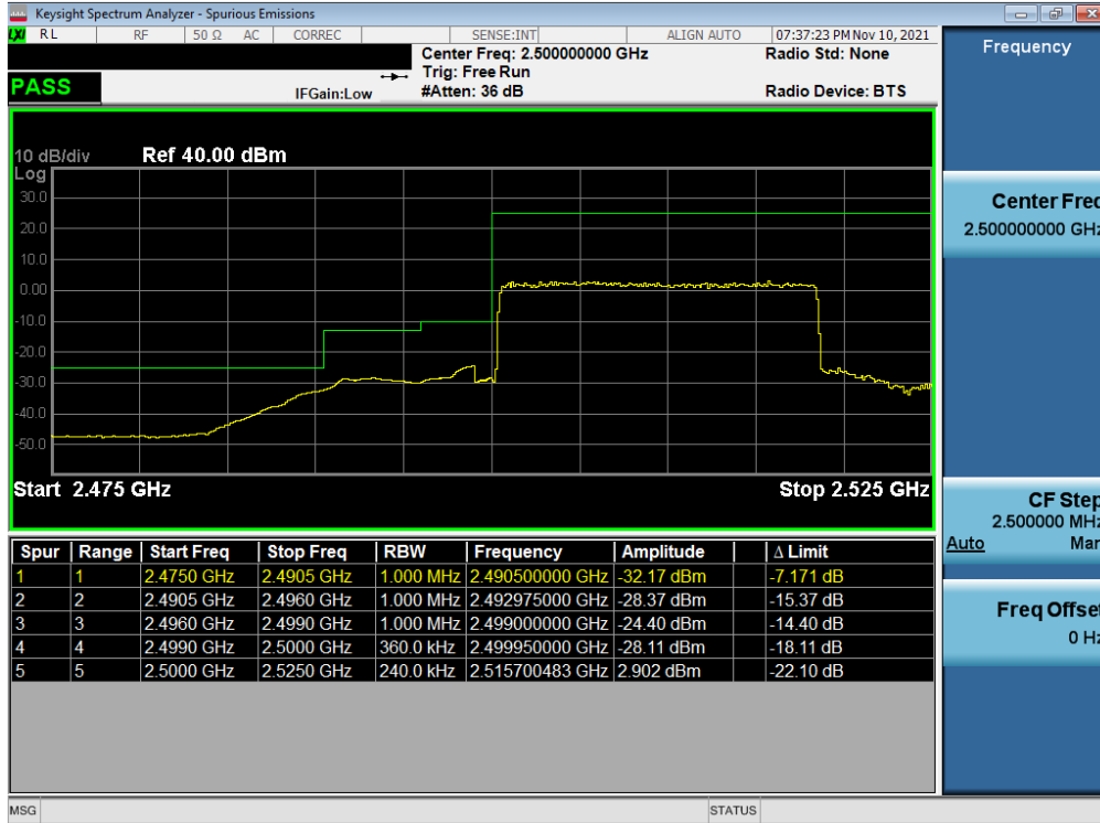
Plot 7-269. Lower Band Edge Plot (NR Band n7 - 20MHz CP-OFDM-QPSK – Full RB - Ant B)
