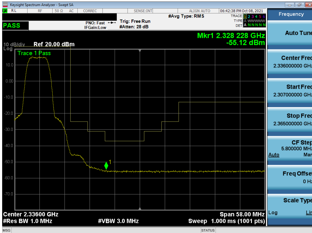
Plot 7-262. Extended Upper Band Edge Plot (NR Band n30 - 5MHz CP-OFDM-QPSK – Full RB - Ant J)
