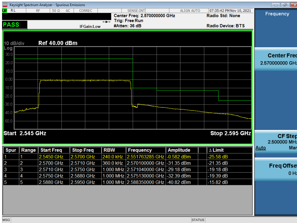
Plot 7-264. Upper Band Edge Plot (NR Band n7 - 40MHz CP-OFDM-QPSK – Full RB - Ant B)
