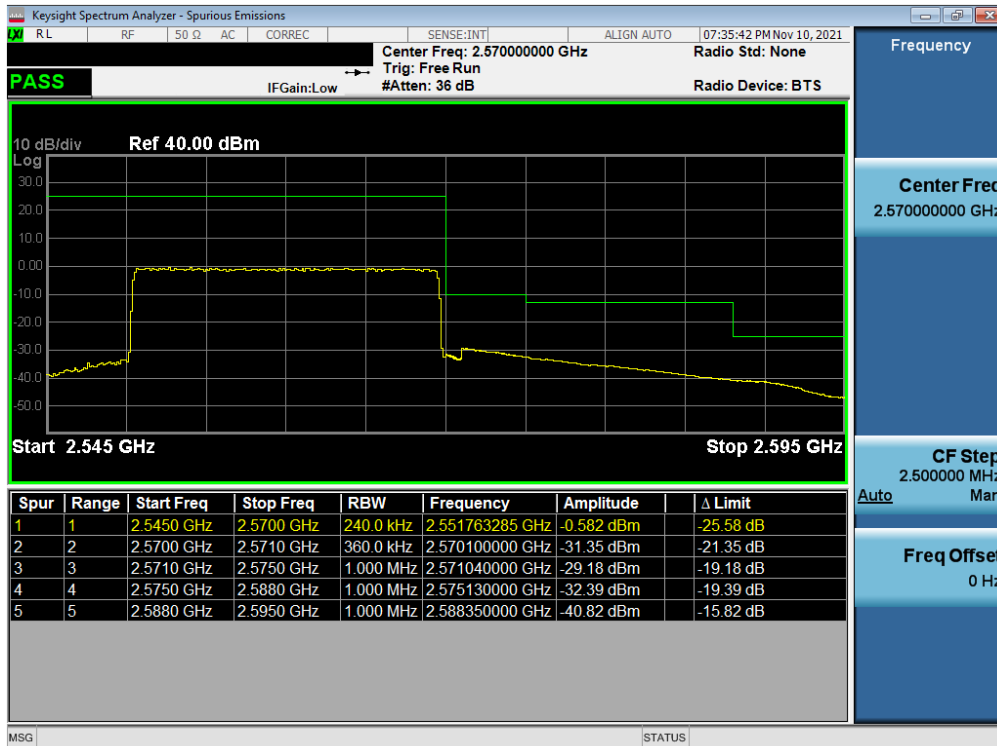
Plot 7-270. Upper Band Edge Plot (NR Band n7 - 20MHz CP-OFDM-QPSK – Full RB - Ant B)
