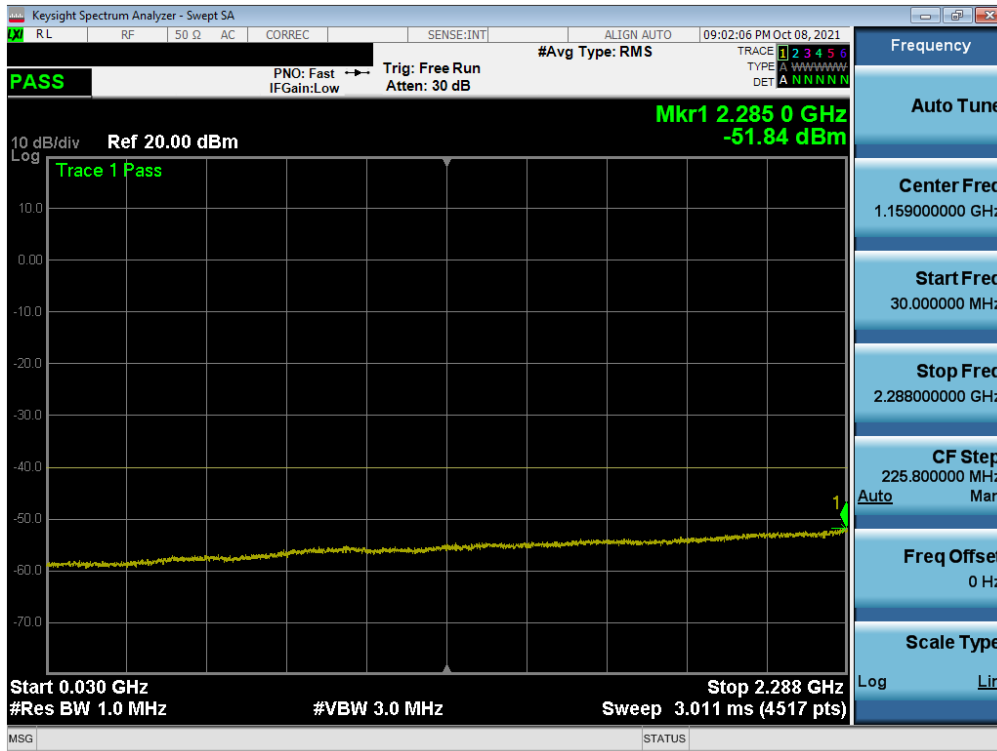
Plot 7-129. Conducted Spurious Plot (NR Band n30 - 10MHz QPSK - RB Size 1, RB Offset 0 – Ant J)
