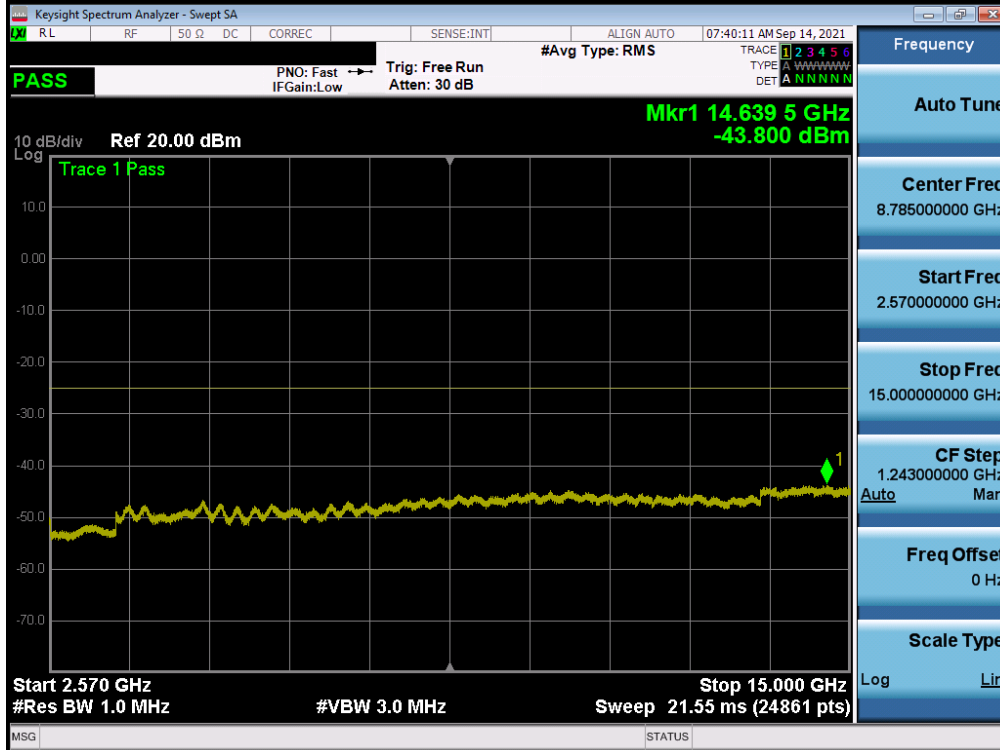
Plot 7-104. Conducted Spurious Plot (LTE Band 7 - 20MHz QPSK - RB Size 1, RB Offset 0 - Mid Channel)
