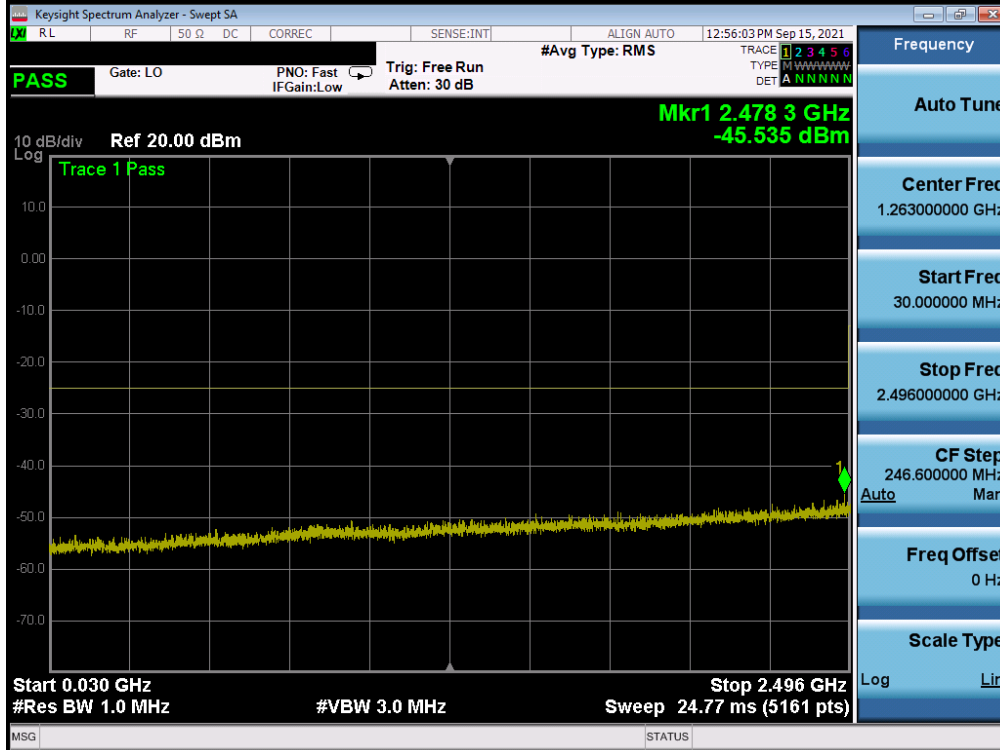
Plot 7-187. Conducted Spurious Plot (ULCA LTE B41(PC2) - 20MHz QPSK - RB Size 1, RB Offset 0 - High Channel)
