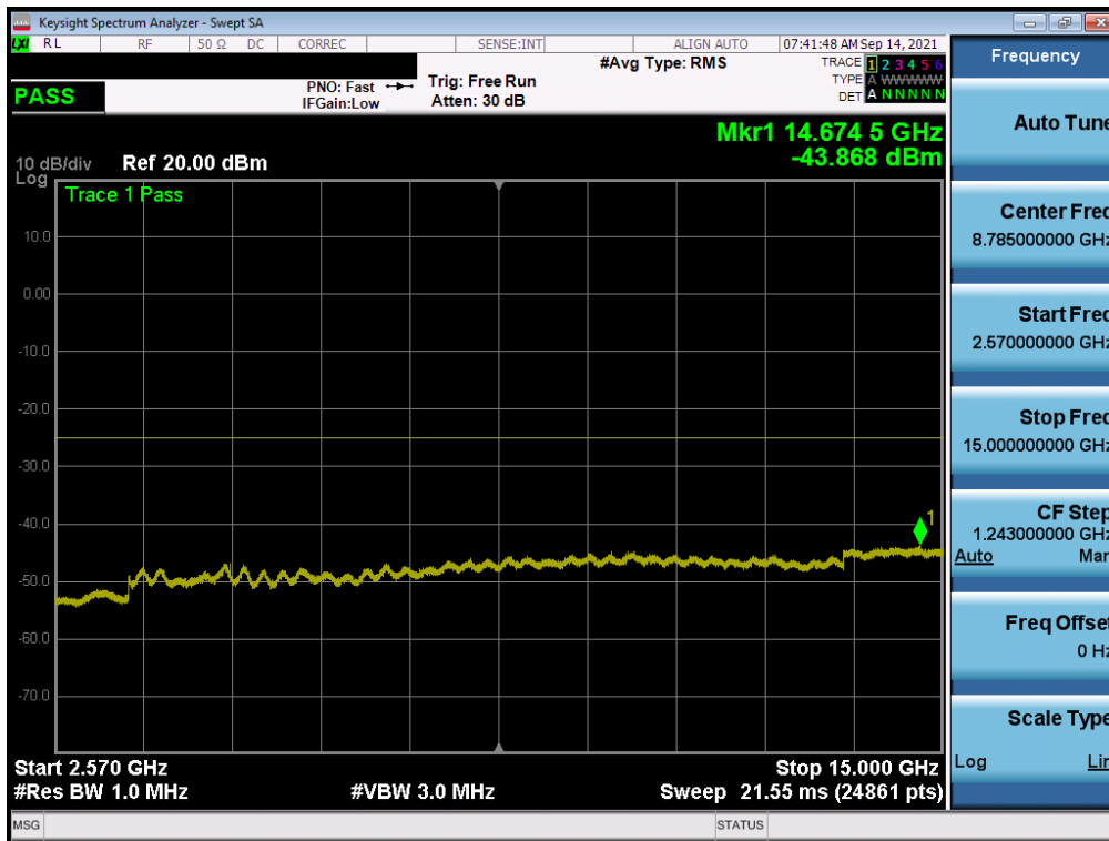
Plot 7-101. Conducted Spurious Plot (LTE Band 7 - 20MHz QPSK - RB Size 1, RB Offset 0 - Low Channel)
