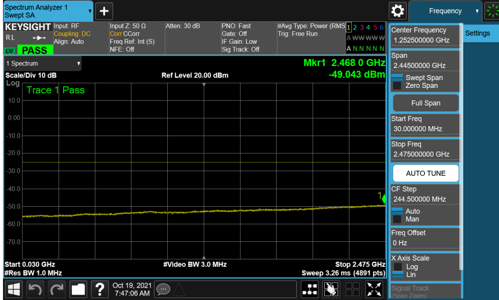
Plot 7-138. Conducted Spurious Plot (NR Band n7 - 40MHz QPSK - RB Size 1, RB Offset 0 - High Channel - Ant B)
