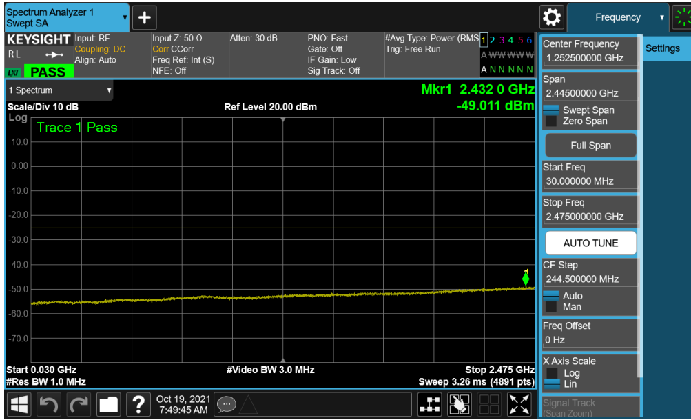
Plot 7-132. Conducted Spurious Plot (NR Band n7 - 40MHz QPSK - RB Size 1, RB Offset 0 - Low Channel - Ant B)
