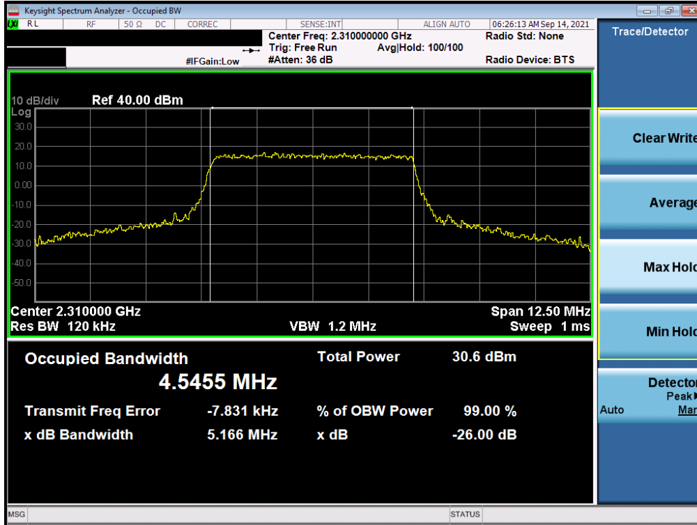
Plot 7-11. Occupied Bandwidth Plot (LTE Band 30 - 5MHz QPSK - Full RB)
