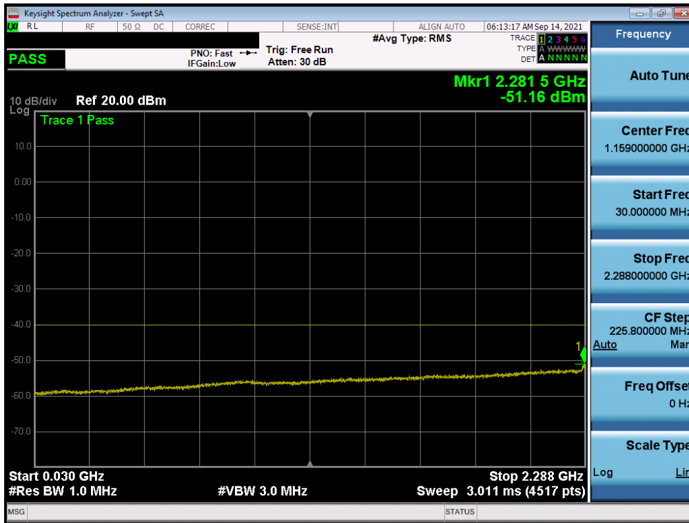
Plot 7-97. Conducted Spurious Plot (LTE Band 30 - 10MHz QPSK - RB Size 1, RB Offset 0)
