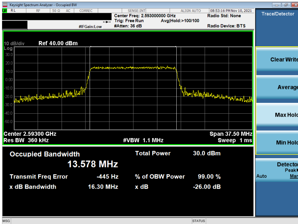
Plot 7-32. Occupied Bandwidth Plot (LTE Band 41(PC3)/38 - 15MHz 16-QAM - Full RB)
