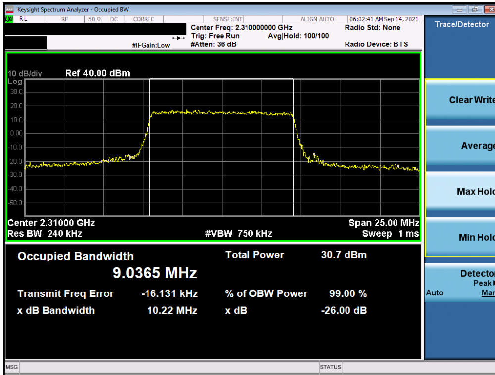
Plot 7-9. Occupied Bandwidth Plot (LTE Band 30 - 10MHz QPSK - Full RB)
