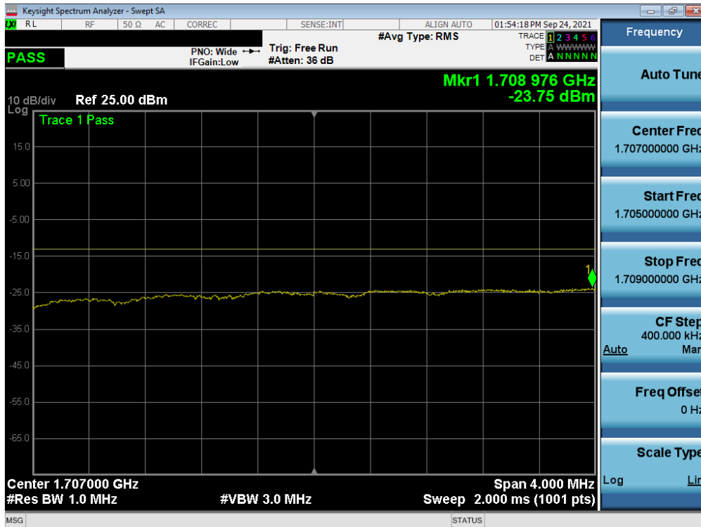
Plot 7-227. Lower Extended Band Edge Plot (NR Band n66 - 40.0MHz - Full RB)
