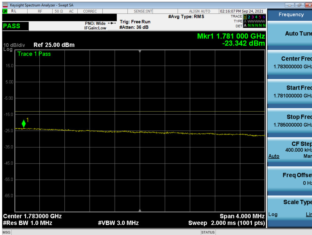
Plot 7-233. Upper Extended Band Edge Plot (NR Band n66 - 30.0MHz - Full RB)
