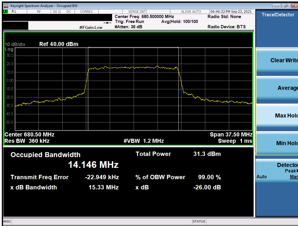
Plot 7-21. Occupied Bandwidth Plot (NR Band n71 - 15MHz DFT-s-OFDM BPSK - Full RB)
