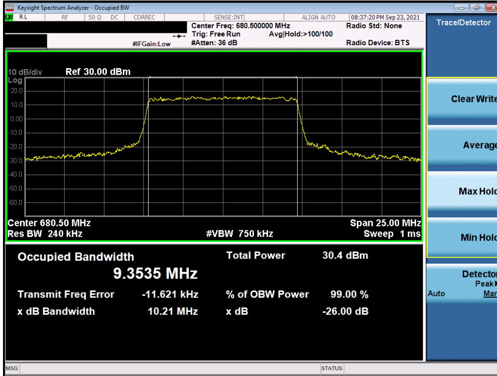
Plot 7-24. Occupied Bandwidth Plot (NR Band n71 - 10MHz DFT-s-OFDM BPSK - Full RB)
