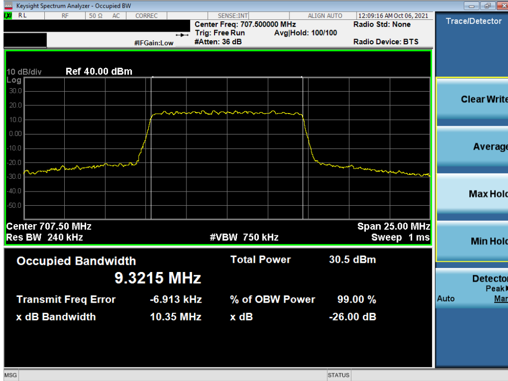
Plot 7-34. Occupied Bandwidth Plot (NR Band n12 - 10MHz CP-OFDM QPSK - Full RB)
