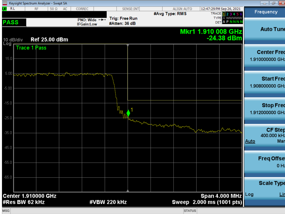
Plot 7-140. Upper Band Edge Plot (NR Band n2 – 5MHz QPSK – Full RB)
