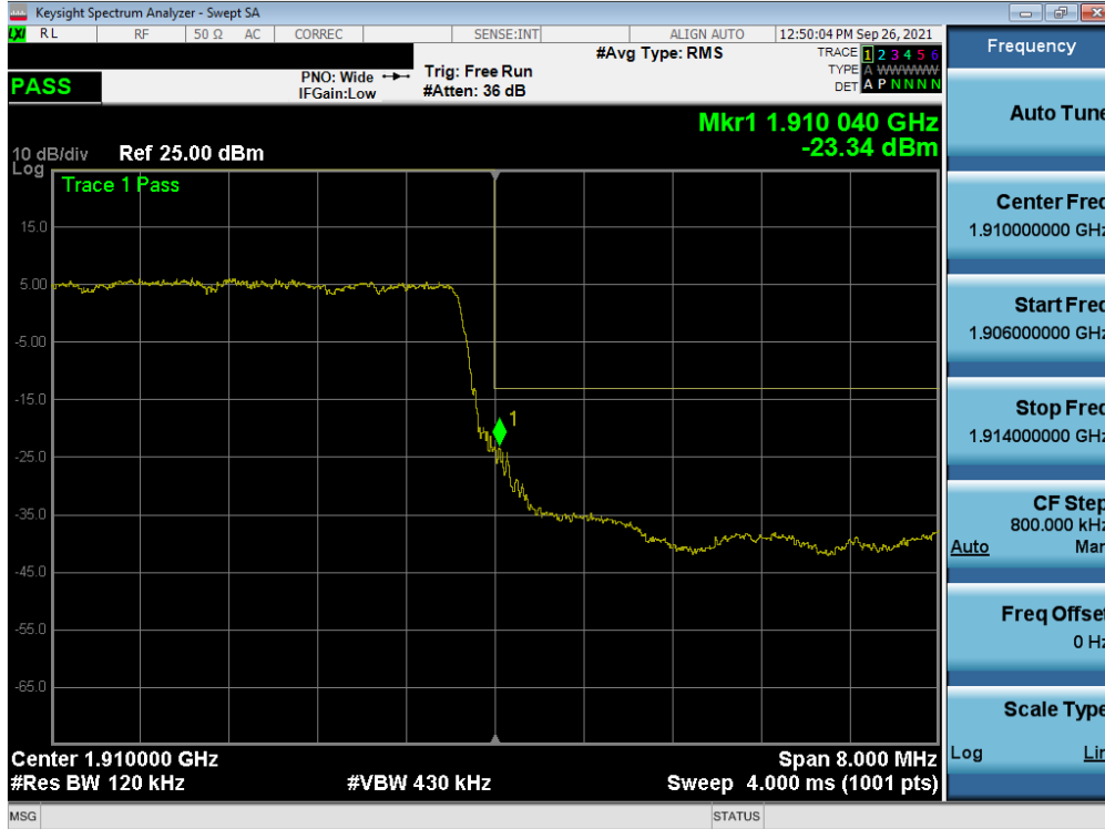
Plot 7-134. Upper Band Edge Plot (NR Band n2 - 10MHz QPSK – Full RB)
