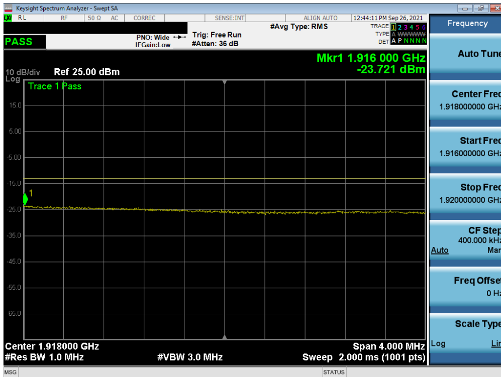
Plot 7-131. Extended Upper Band Edge Plot (NR Band n25 - 15MHz QPSK – Full RB)
