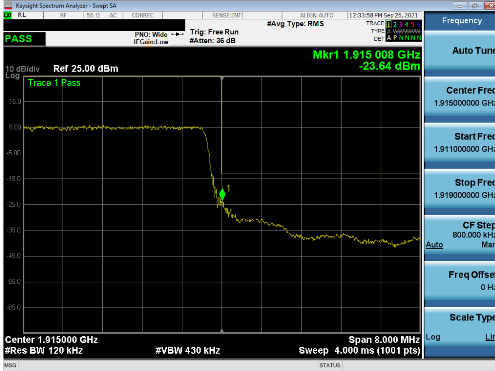
Plot 7-136. Upper Band Edge Plot (NR Band n25 - 10MHz QPSK – Full RB)
