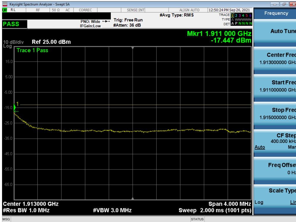
Plot 7-135. Extended Upper Band Edge Plot (NR Band n2 - 10MHz QPSK – Full RB)
