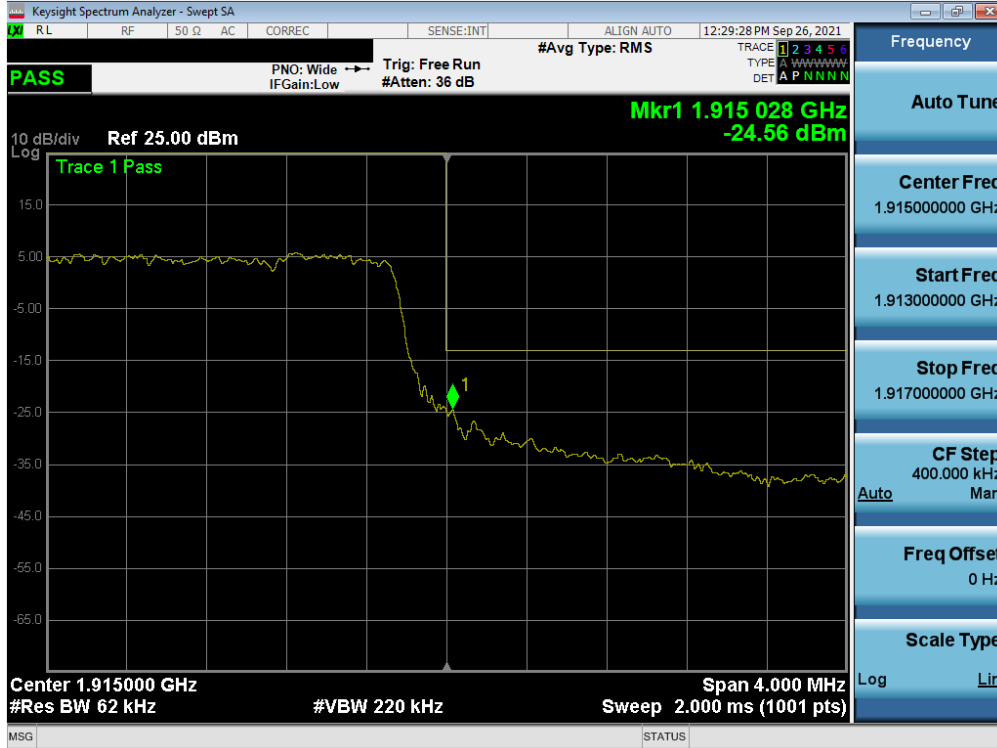
Plot 7-142. Upper Band Edge Plot (NR Band n25 – 5MHz QPSK – Full RB)
