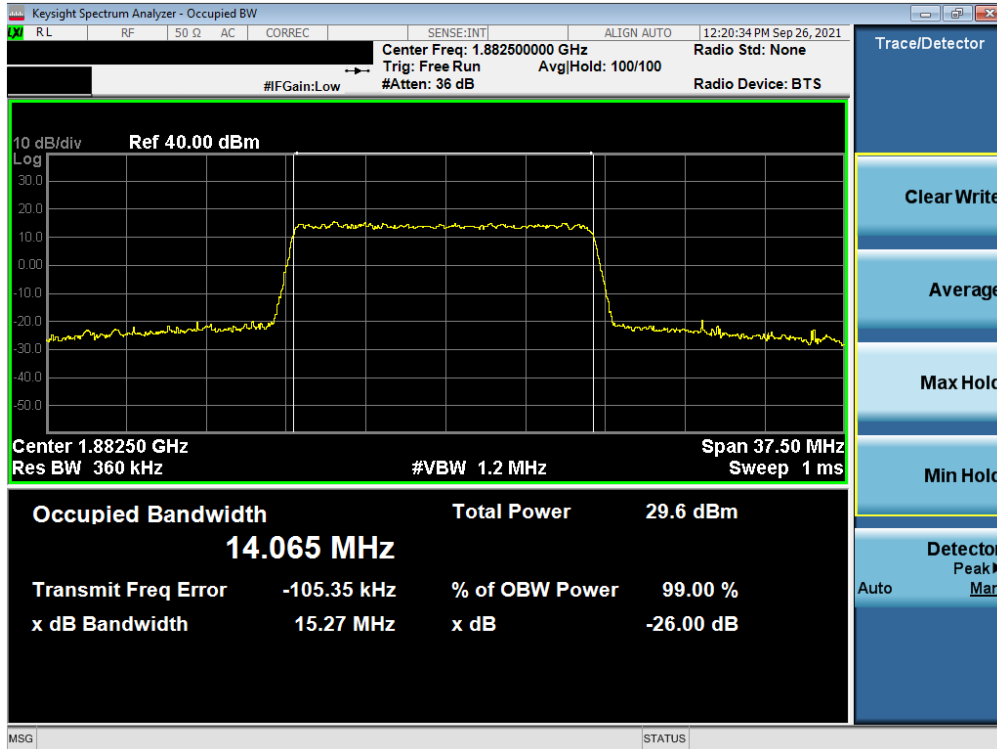
Plot 7-27. Occupied Bandwidth Plot (NR Band n25/2 - 15.0MHz CP-OFDM QPSK - Full RB)
