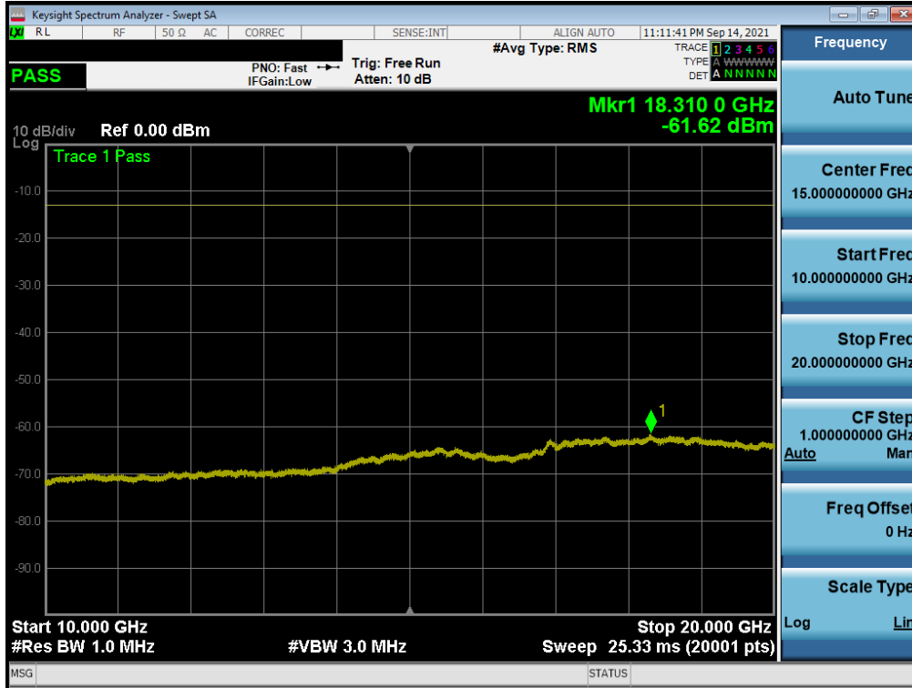
Plot 7-73. Conducted Spurious Plot (WCDMA Ch. 9538)
