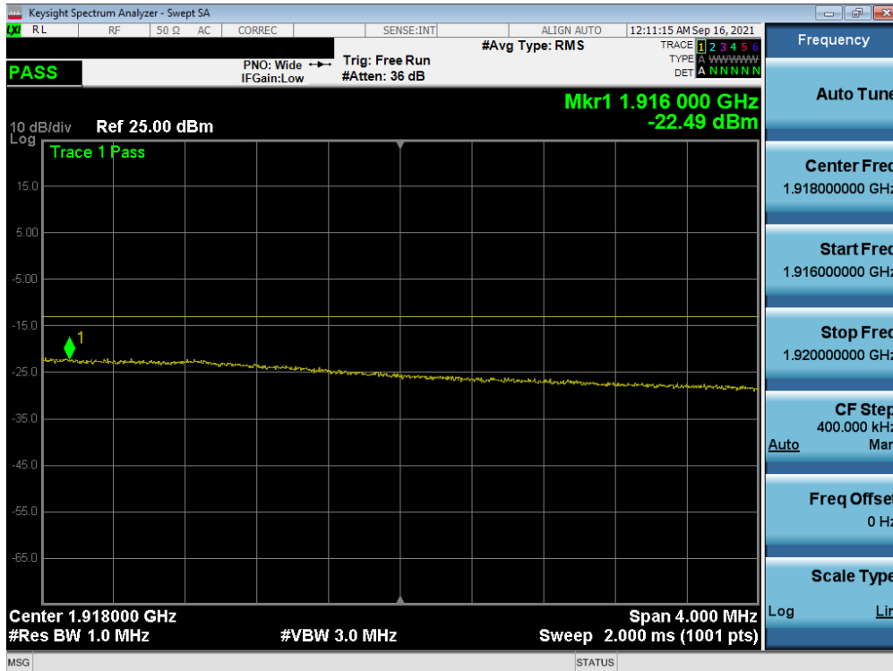
Plot 7-83. Extended Upper Band Edge Plot (LTE Band 25 - 15MHz QPSK – Full RB)
