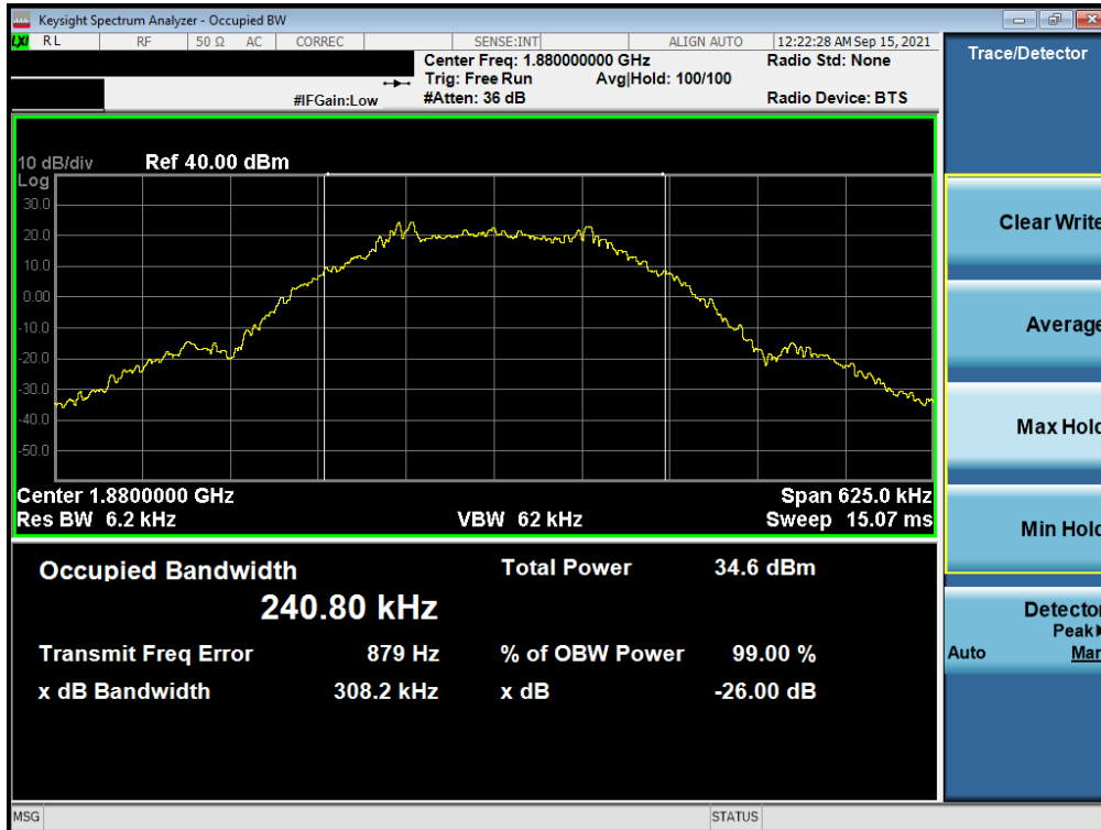
Plot 7-36. Occupied Bandwidth Plot (EDGE, Ch. 661)
