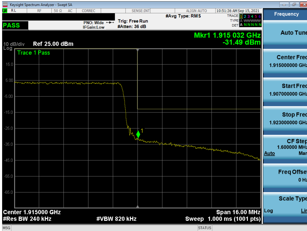
Plot 7-77. Upper Band Edge Plot (LTE Band 25 - 20MHz QPSK – Full RB)
