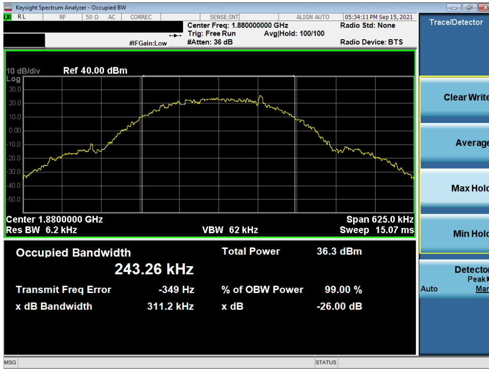
Plot 7-35. Occupied Bandwidth Plot (GPRS, Ch. 661)
