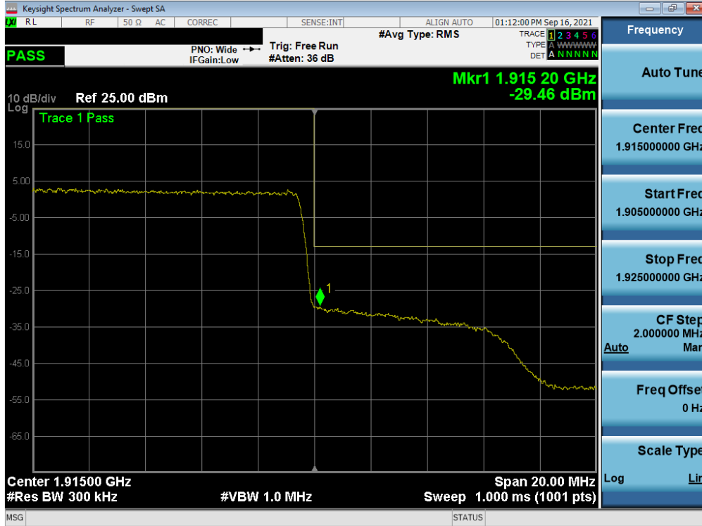
Plot 7-118. Upper Band Edge Plot (NR Band n25 - 25MHz QPSK – Full RB)
