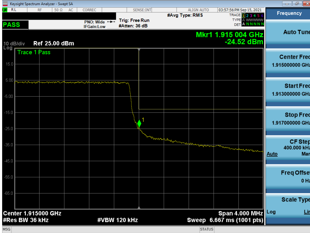
Plot 7-100. Upper Band Edge Plot (LTE Band 25 - 3MHz QPSK – Full RB)
