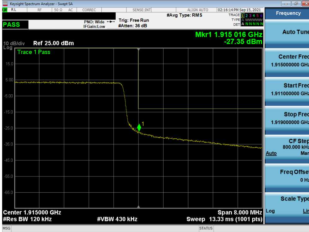
Plot 7-88. Upper Band Edge Plot (LTE Band 25 - 10MHz QPSK – Full RB)
