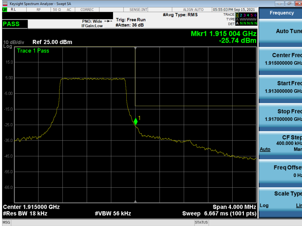
Plot 7-106. Upper Band Edge Plot (LTE Band 25 – 1.4MHz QPSK – Full RB)
