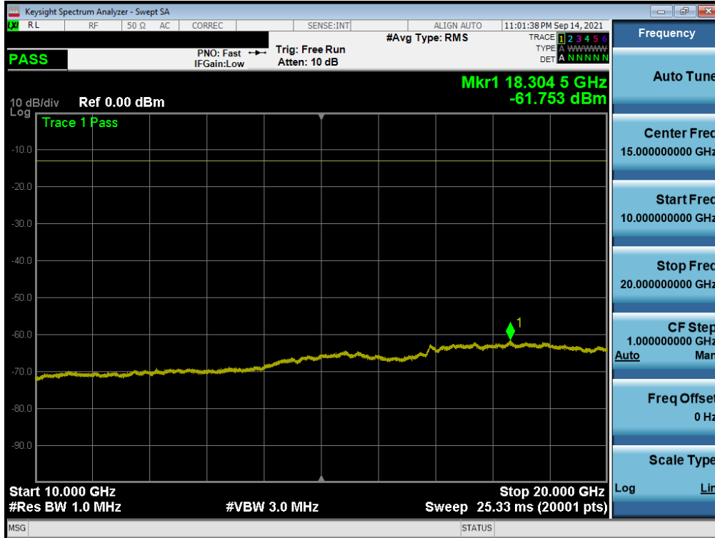
Plot 7-67. Conducted Spurious Plot (WCDMA Ch. 9262)
