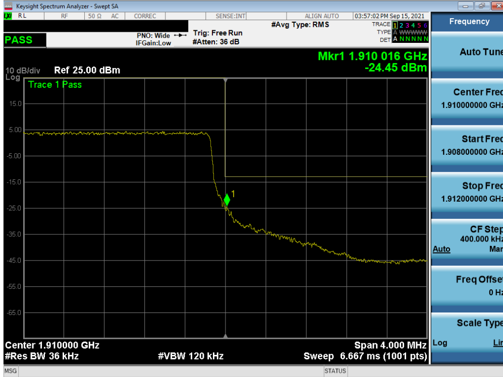
Plot 7-98. Upper Band Edge Plot (LTE Band 2 - 3MHz QPSK – Full RB)
