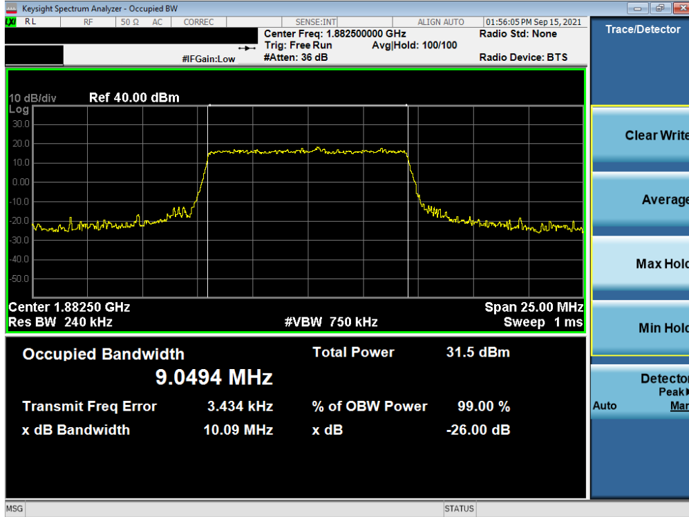
Plot 7-6. Occupied Bandwidth Plot (LTE Band 25/2 - 10MHz QPSK - Full RB)
