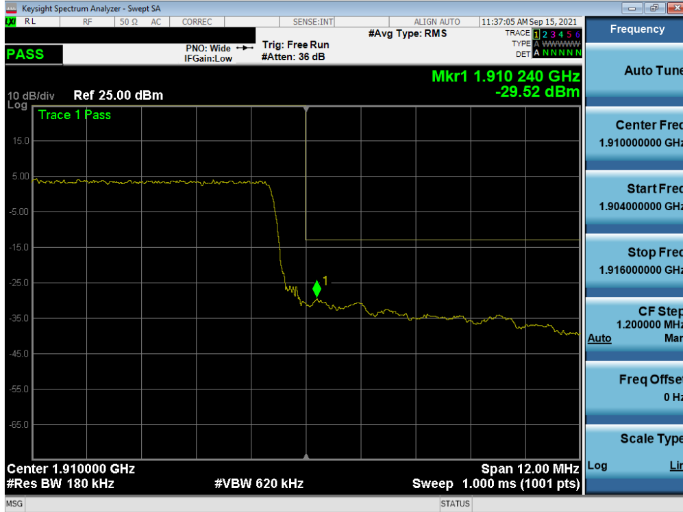
Plot 7-80. Upper Band Edge Plot (LTE Band 2 - 15MHz QPSK – Full RB)
