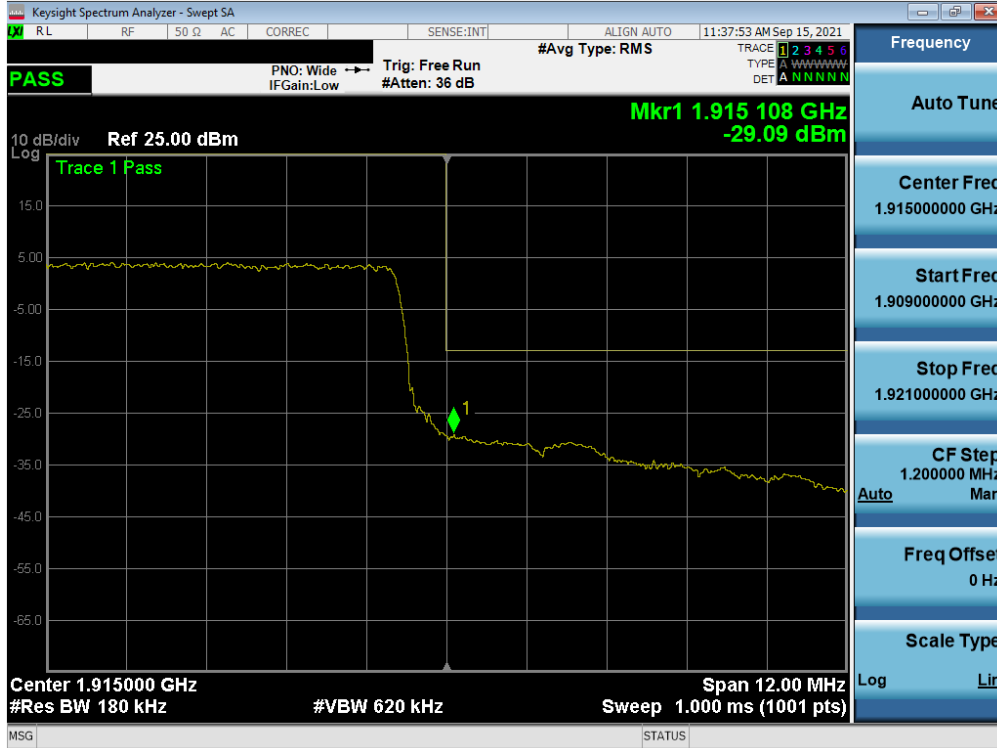
Plot 7-82. Upper Band Edge Plot (LTE Band 25 - 15MHz QPSK – Full RB)
