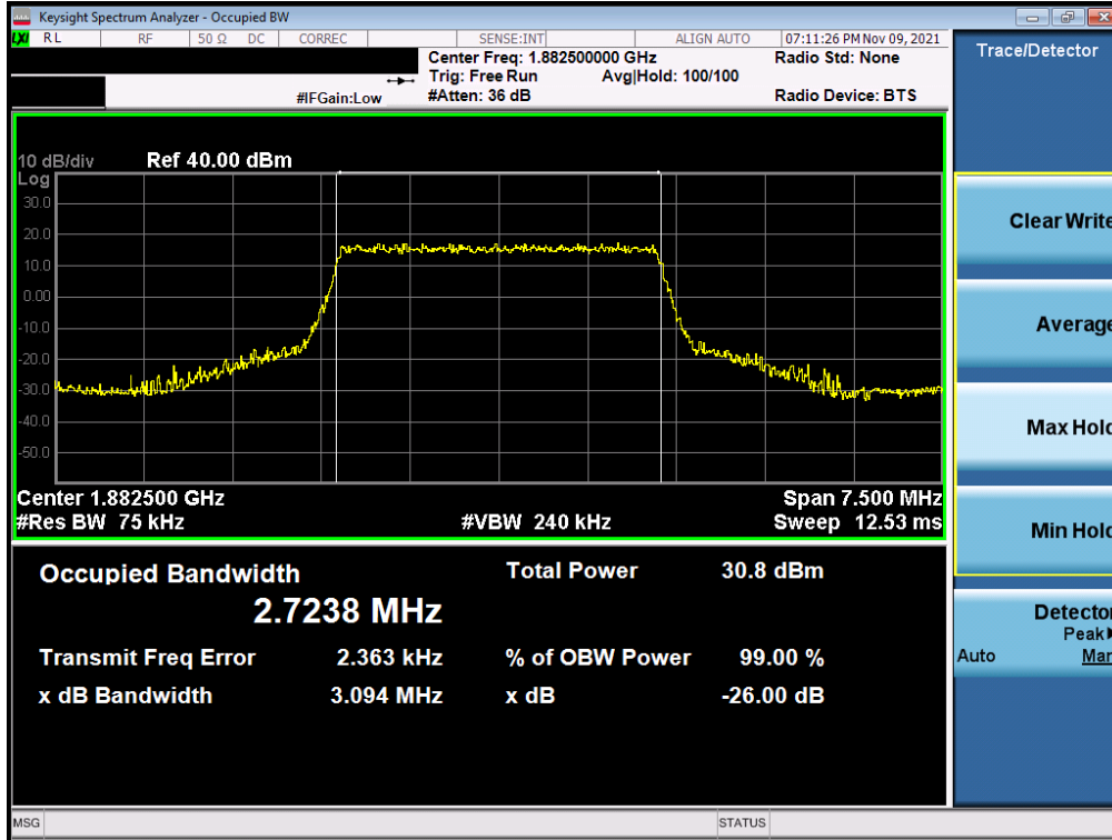
Plot 7-10. Occupied Bandwidth Plot (LTE Band 25/2 - 3MHz QPSK - Full RB)
