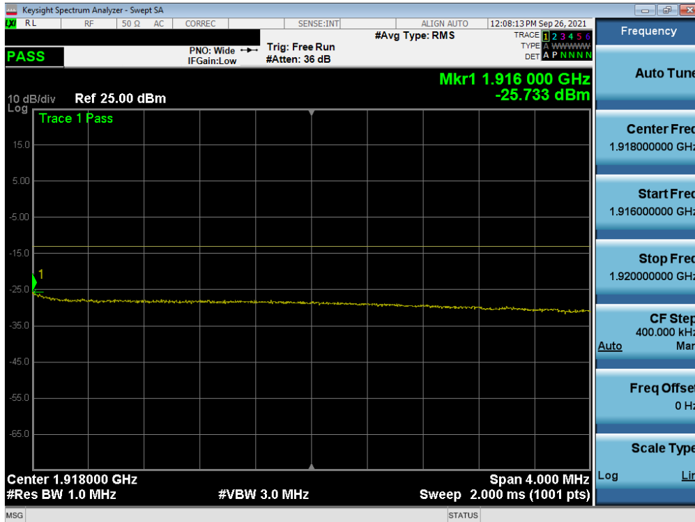
Plot 7-125. Extended Upper Band Edge Plot (NR Band n25 - 20MHz QPSK – Full RB)
