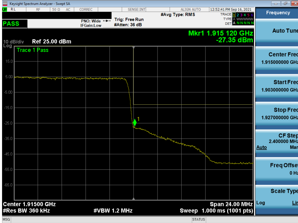
Plot 7-114. Upper Band Edge Plot (NR Band n25 - 30MHz QPSK – Full RB)
