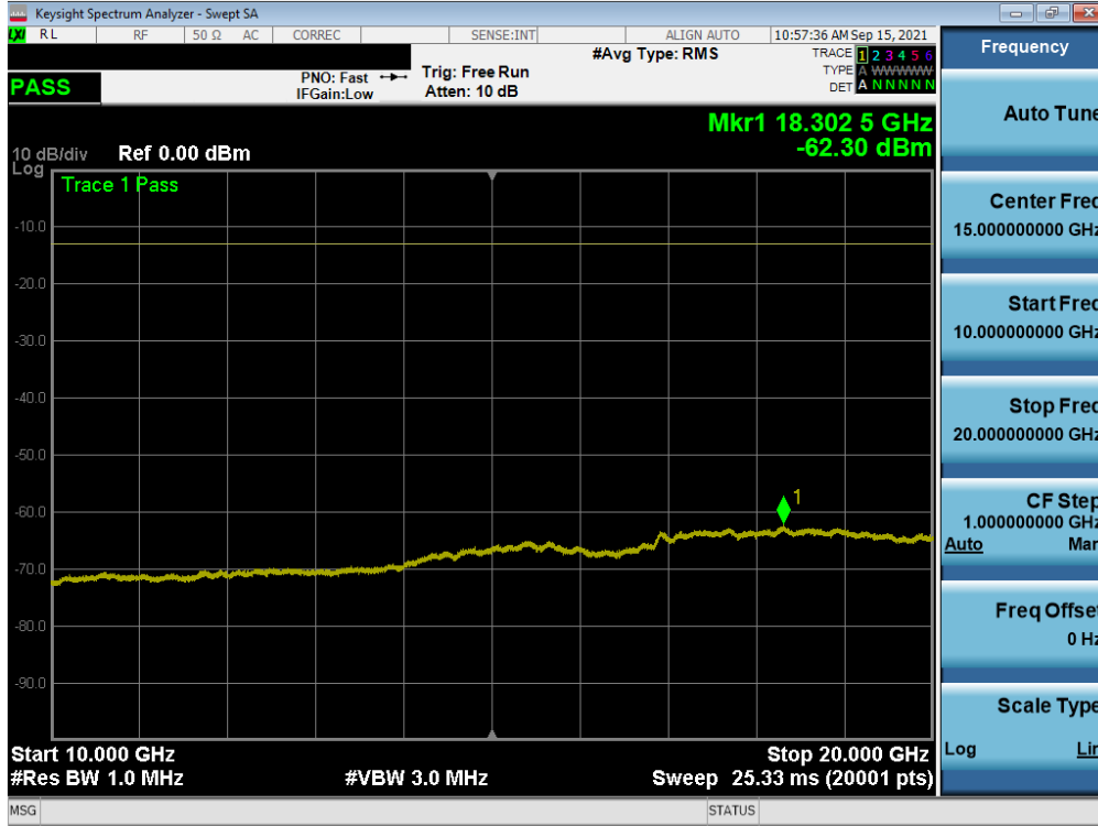
Plot 7-40. Conducted Spurious Plot (LTE Band 25/2 - 20MHz QPSK - 1RB - Low Channel)
