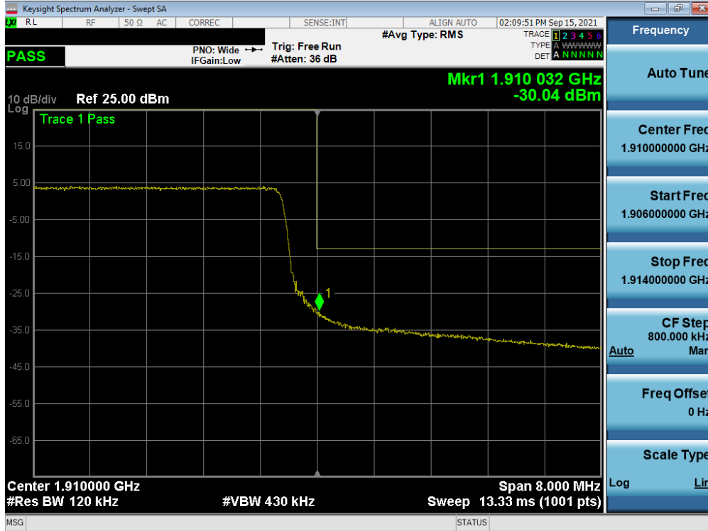
Plot 7-86. Upper Band Edge Plot (LTE Band 2 - 10MHz QPSK – Full RB)
