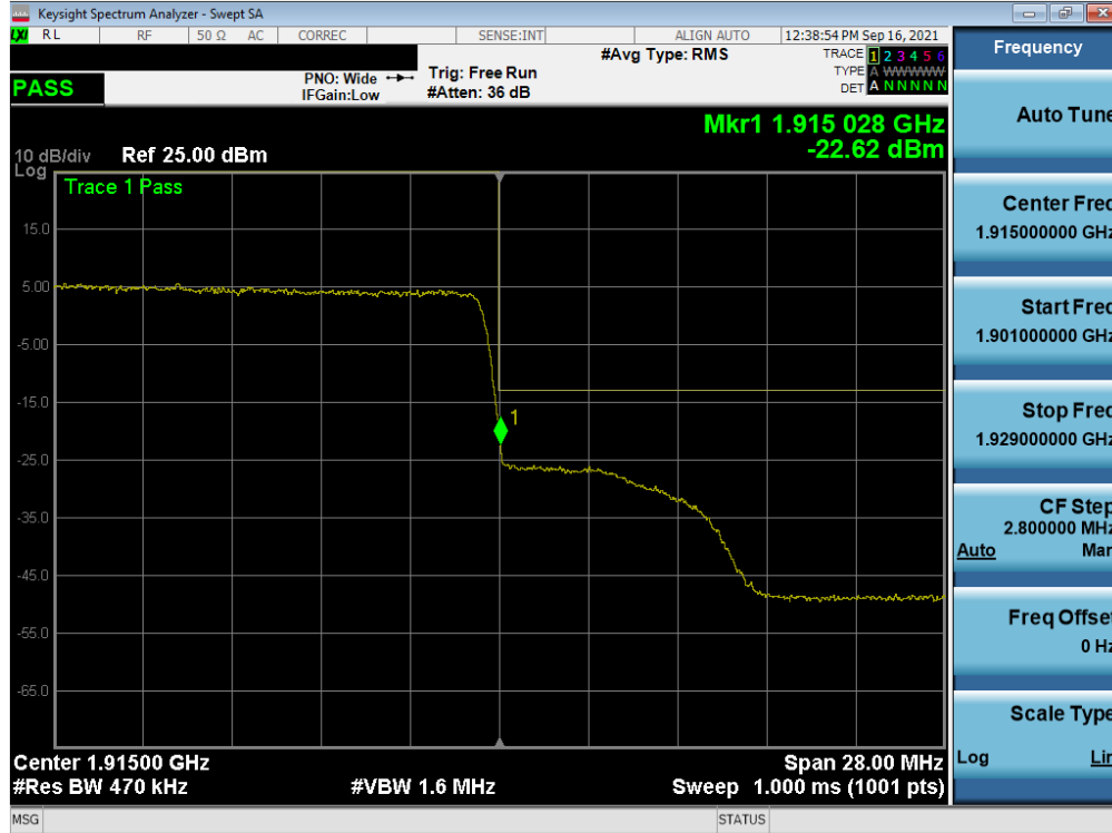
Plot 7-110. Upper Band Edge Plot (NR Band n25 - 40MHz QPSK – Full RB)
