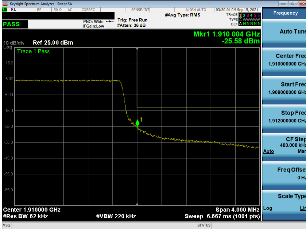
Plot 7-92. Upper Band Edge Plot (LTE Band 2 - 5MHz QPSK – Full RB)
