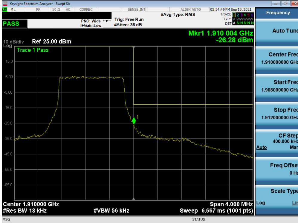
Plot 7-104. Upper Band Edge Plot (LTE Band 2 – 1.4MHz QPSK – Full RB)
