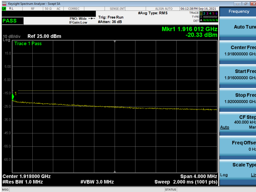
Plot 7-89. Extended Upper Band Edge Plot (LTE Band 25 - 10MHz QPSK – Full RB)
