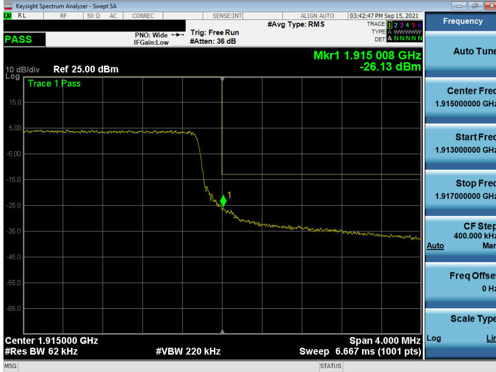
Plot 7-94. Upper Band Edge Plot (LTE Band 25 - 5MHz QPSK – Full RB)
