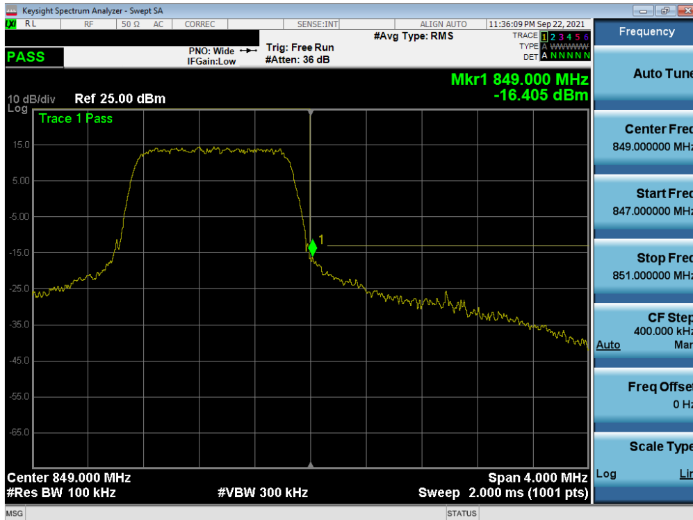
Plot 7-71. Upper Band Edge Plot (LTE Band 26/5 – 1.4MHz QPSK – Full RB)
