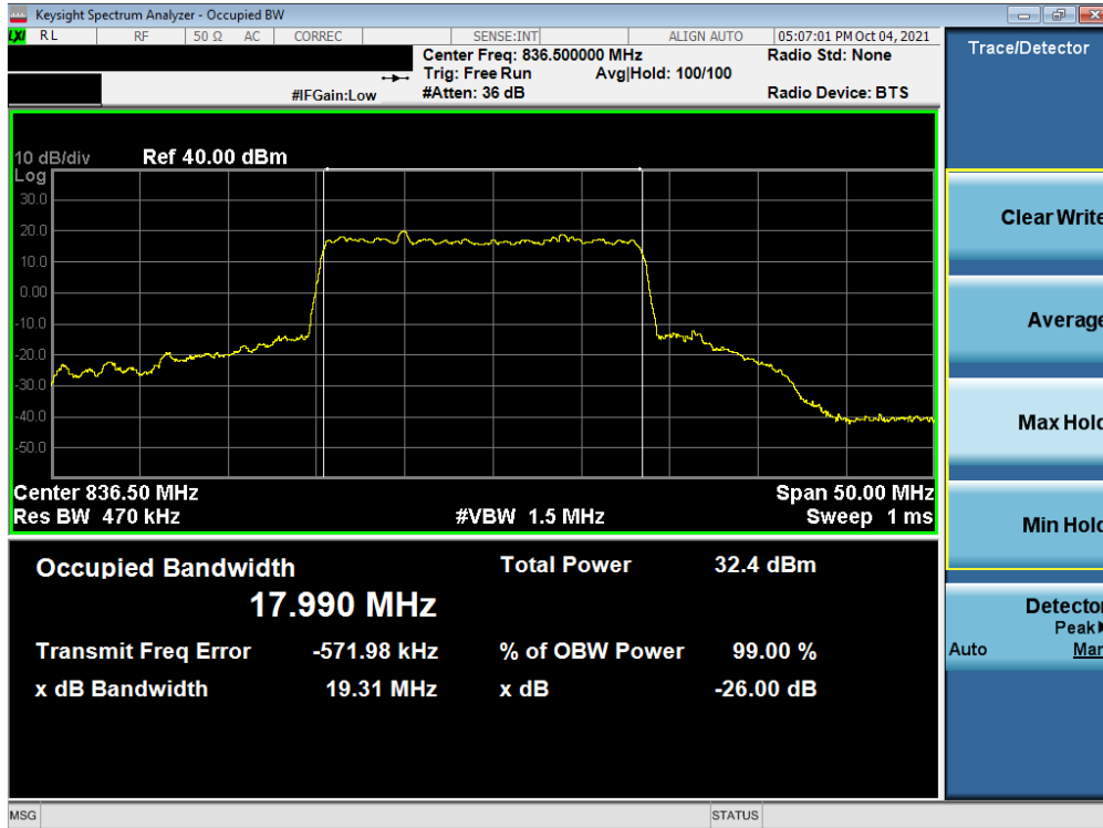
Plot 7-11. Occupied Bandwidth Plot (NR Band n5 - 20MHz \pi/2 BPSK - Full RB)
