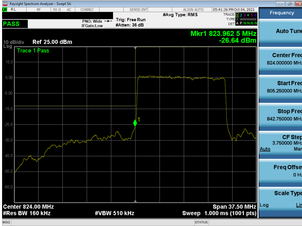
Plot 7-74. Lower Band Edge Plot (NR Band n5 – 15.0MHz - Full RB)
