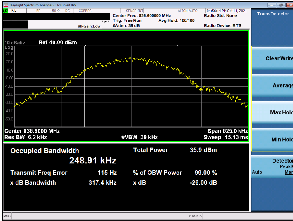
Plot 7-23. Occupied Bandwidth Plot (GPRS, Ch. 190)
