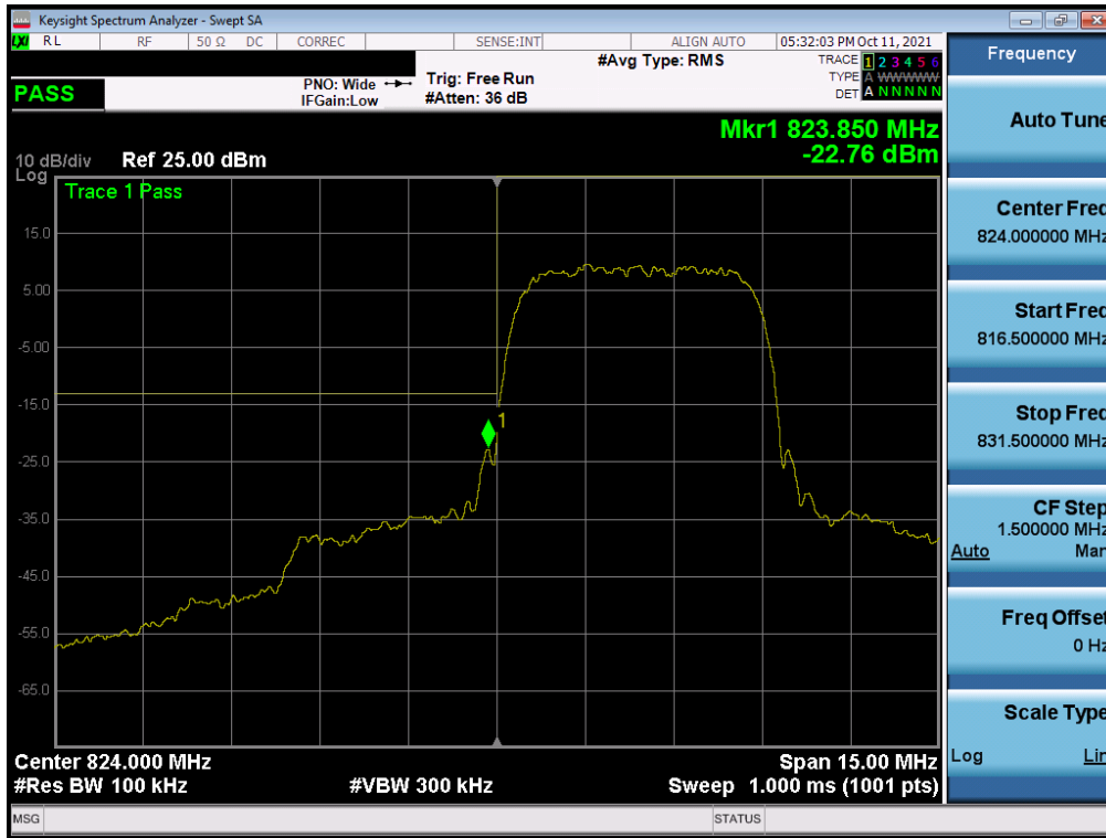
Plot 7-82. Lower Band Edge Plot (WCDMA Cell – Ch. 4132)
