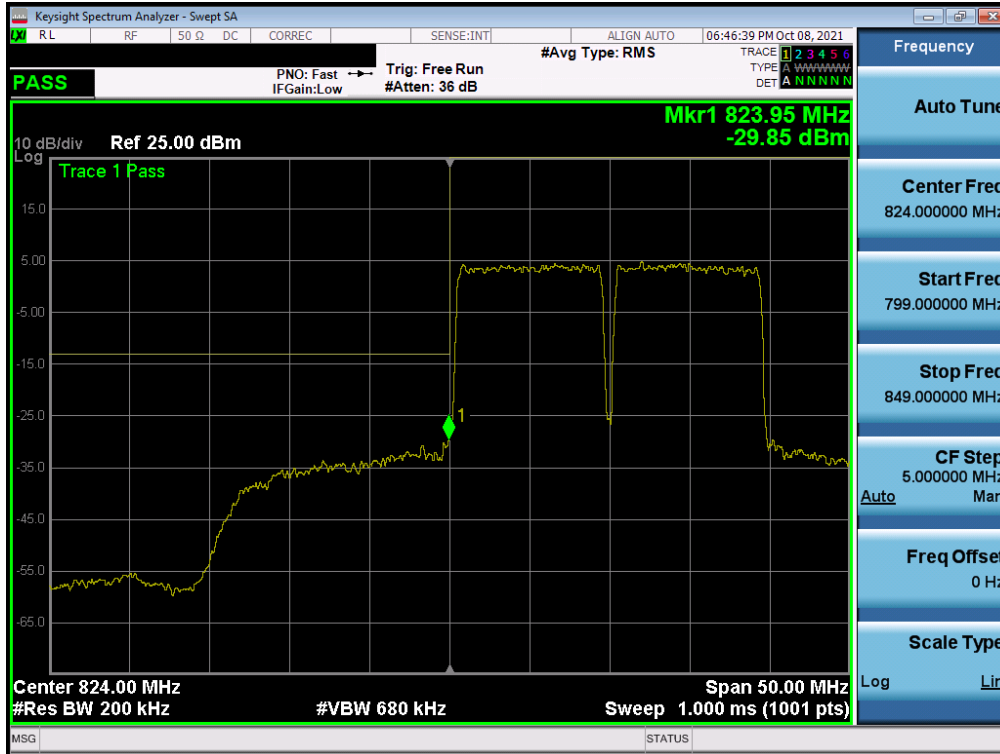
Plot 7-93. Lower Band Edge Plot (Band 5 QPSK – PCC: 10MHz SCC: 10MHz – Full RB)
