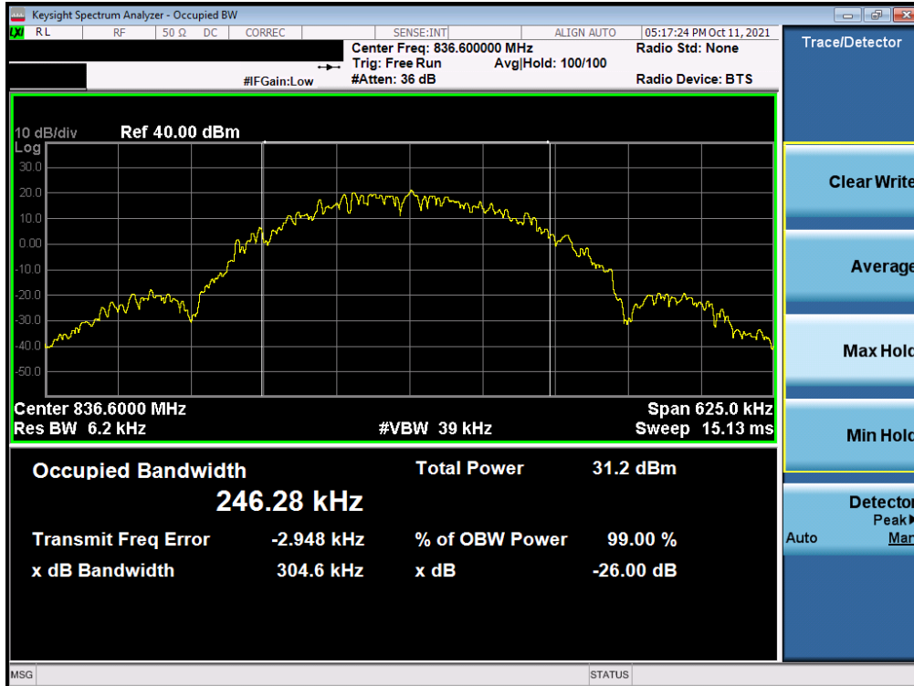
Plot 7-24. Occupied Bandwidth Plot (EDGE, Ch. 190)
