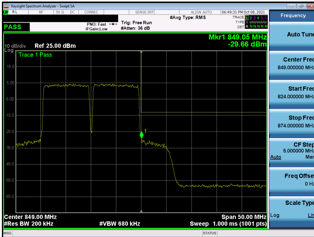
Plot 7-94. Upper Band Edge Plot (Band 5 QPSK – PCC: 10MHz SCC: 10MHz – Full RB)
