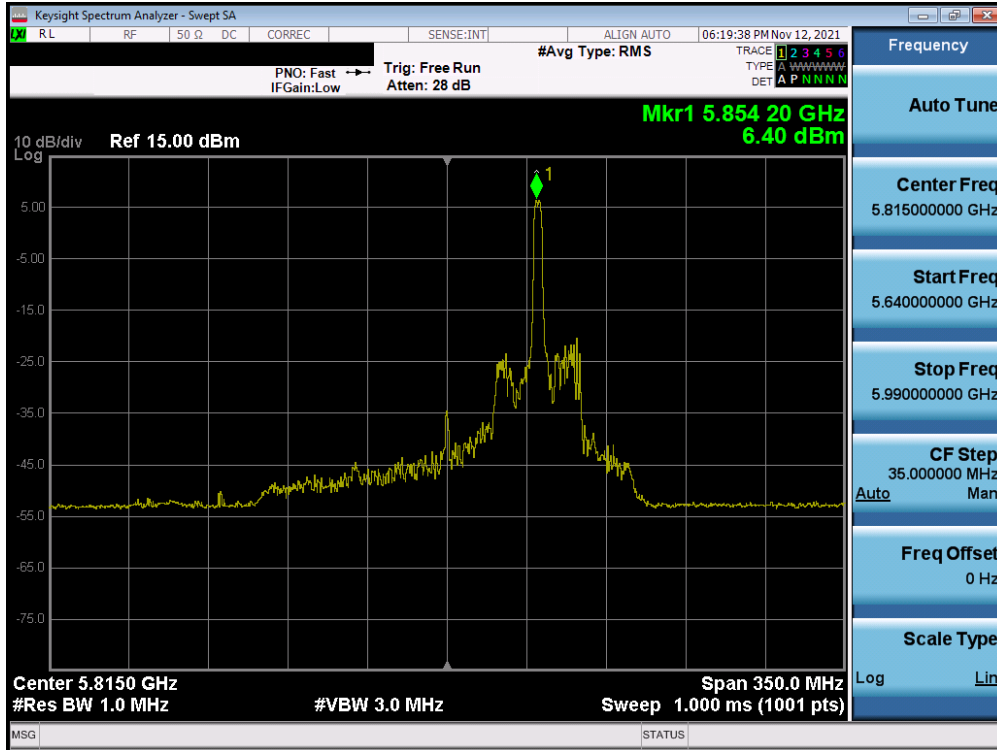
Plot 7-273. Power Spectral Density Plot MIMO ANT2 (160MHz BW U 802.11ax – 26 Tones (UNII Band 3/4) – Ch. 163)
