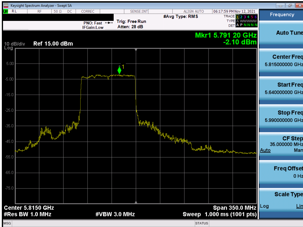
Plot 7-311. Power Spectral Density Plot MIMO ANT2 (160MHz BW L 802.11ax – 996 Tones (UNII Band 3/4) – Ch. 163)
