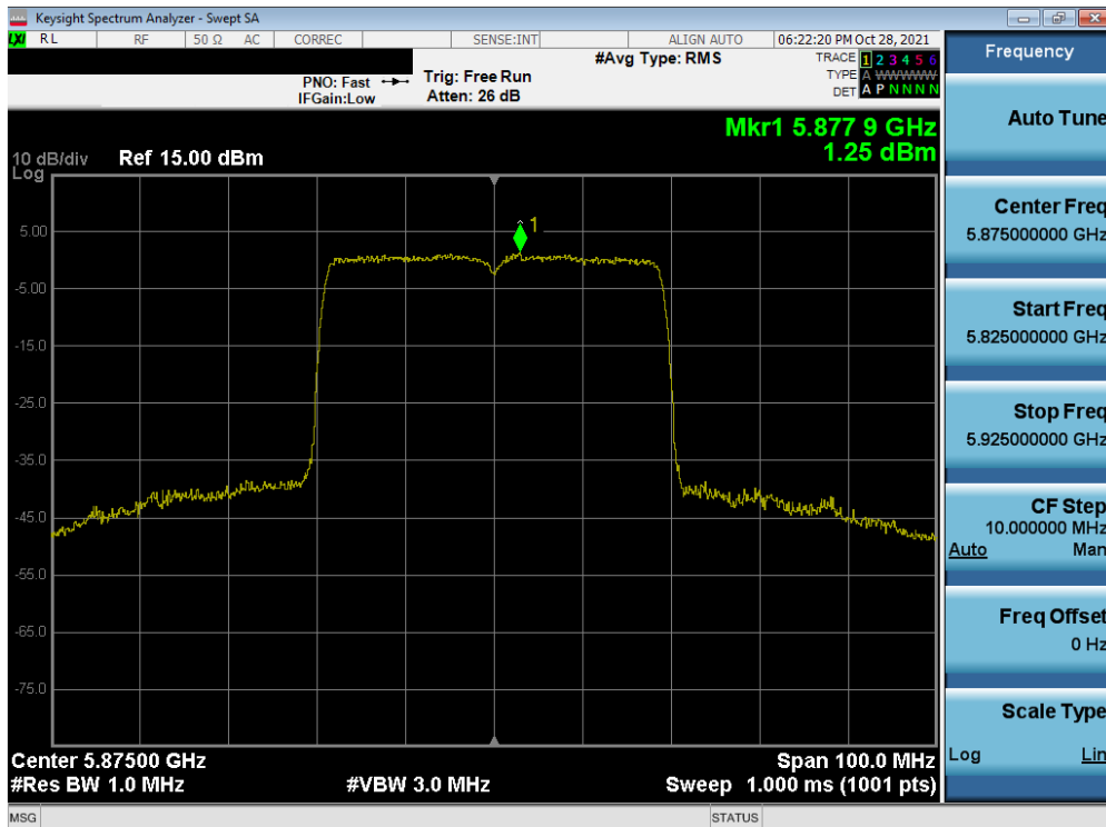
Plot 7-309. Power Spectral Density Plot MIMO ANT2 (40MHz BW 802.11ax – 484 Tones (UNII Band 3) – Ch. 175)
