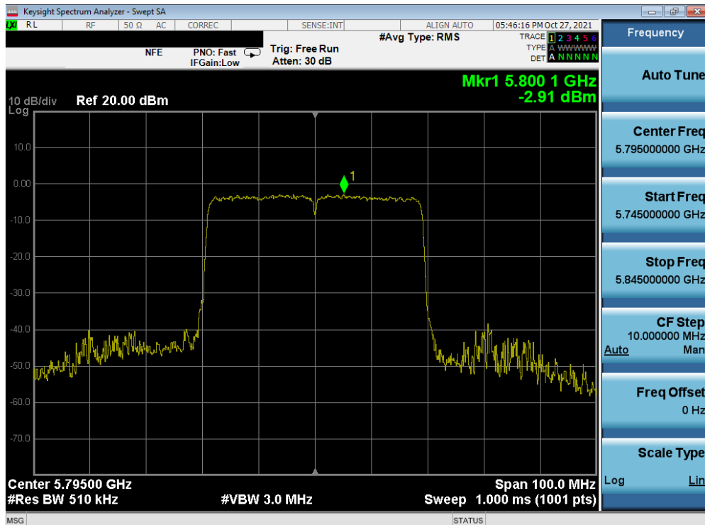
Plot 7-225. Power Spectral Density Plot MIMO ANT1 (40MHz BW 802.11ax – Full Tones (UNII Band 3) – Ch. 159)
