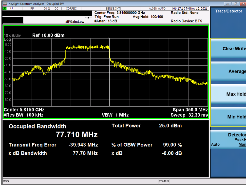
Plot 7-155. 6dB Bandwidth Plot MIMO ANT2 (160MHz BW L 802.11ax – 996 Tones (UNII Band 3/4) – Ch. 163)
