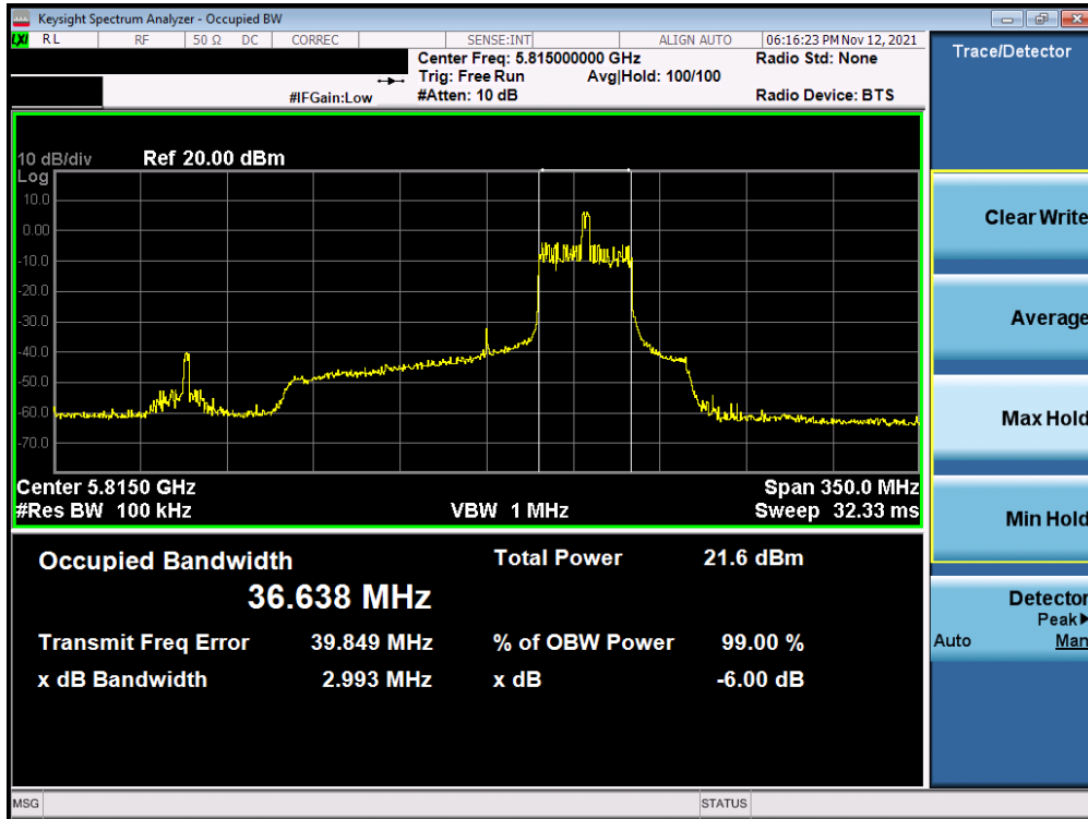
Plot 7-142. 6dB Bandwidth Plot MIMO ANT2 (160MHz BW U 802.11ax – 26 Tones (UNII Band 3/4) – Ch. 163)
