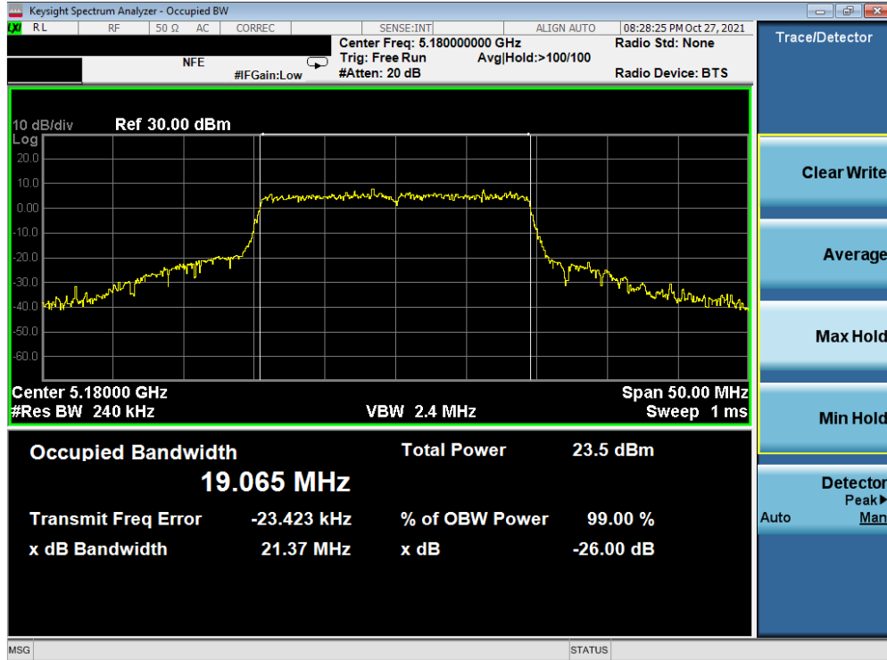
Plot 7-76. 26dB Bandwidth Plot MIMO ANT2 (20MHz BW 802.11ax – 242 Tones (UNII Band 1) – Ch. 36)
