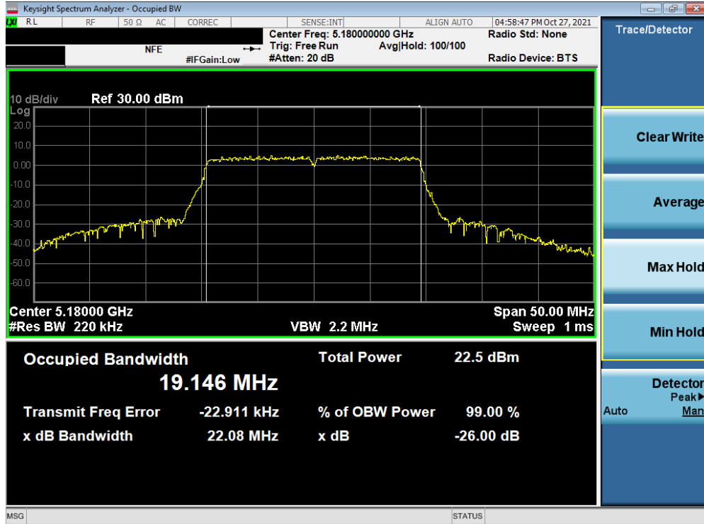
Plot 7-26. 26dB Bandwidth Plot MIMO ANT1 (20MHz BW 802.11ax – 242 Tones (UNII Band 1) – Ch. 36)
