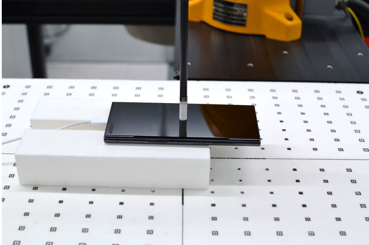
Figure D-4 Near Field Power Density Test Setup Photo – Front Side at 2mm
