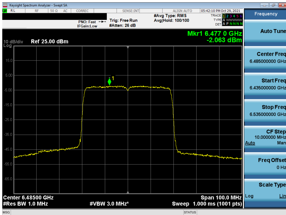
Plot 7-221. Power Spectral Density Plot MIMO ANT1 (40MHz BW 802.11ax (FULL Tones) (UNII Band 6) – Ch. 107)
