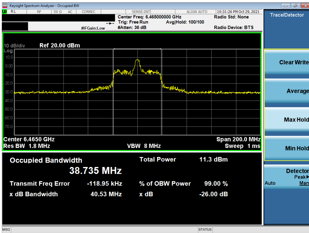
Plot 7-102. 26dB Bandwidth Plot MIMO ANT2 (80MHz BW 802.11ax (26 Tones) (UNII Band 6) – Ch. 103)
