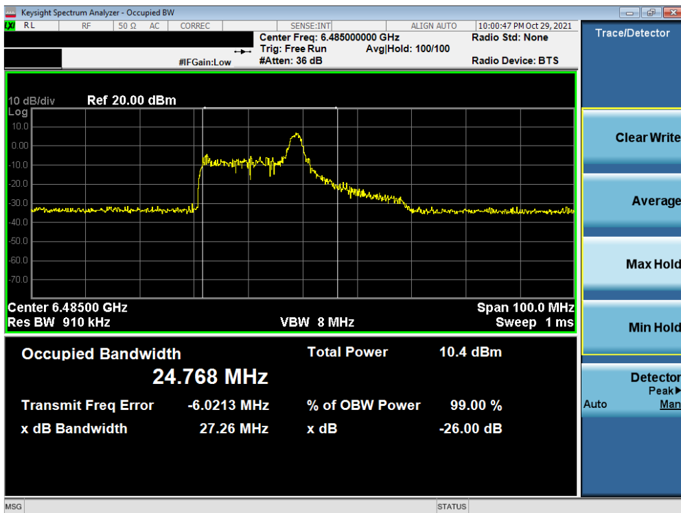
Plot 7-100. 26dB Bandwidth Plot MIMO ANT2 (40MHz BW 802.11ax (26 Tones) (UNII Band 6) – Ch. 107)
