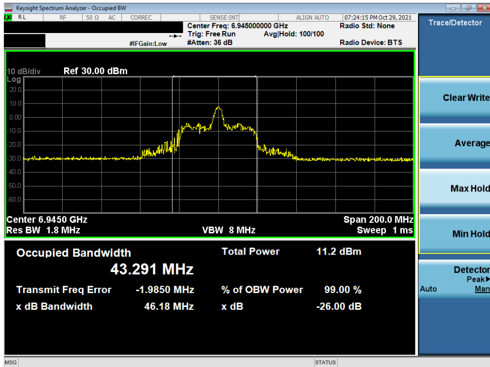
Plot 7-44. 26dB Bandwidth Plot MIMO ANT1 (80MHz BW 802.11ax (26 Tones) (UNII Band 8) – Ch. 199)
