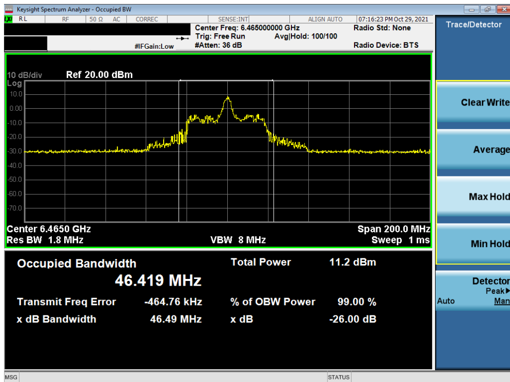
Plot 7-22. 26dB Bandwidth Plot MIMO ANT1 (80MHz BW 802.11ax (26 Tones) (UNII Band 6) – Ch. 103)
