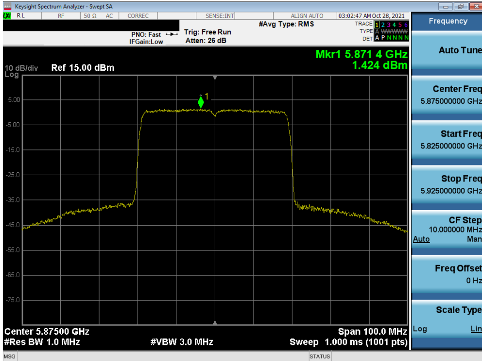
Plot 7-344. Power Spectral Density Plot MIMO ANT2 (40MHz BW 802.11ax (UNII Band 4) – Ch. 175)
