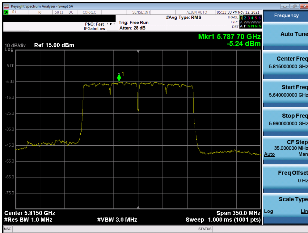
Plot 7-261. Power Spectral Density Plot MIMO ANT1 (160MHz BW 802.11ax (UNII Band 3/4) – Ch. 163)
