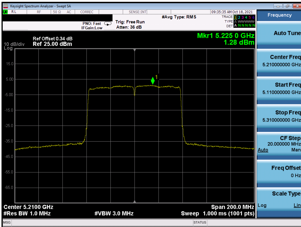
Plot 7-188. Power Spectral Density Plot MIMO ANT1 (80MHz BW 802.11ac (UNII Band 1) – Ch. 42)
