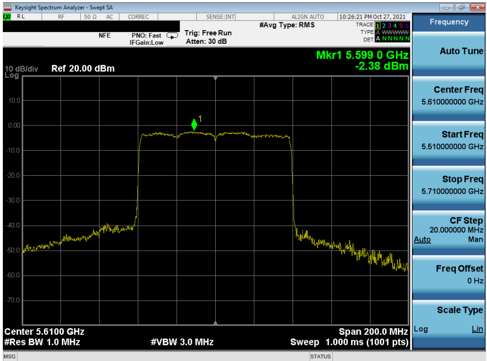
Plot 7-295. Power Spectral Density Plot MIMO ANT2 (80MHz BW 802.11ax – Full Tones (UNII Band 2C) – Ch. 122)
