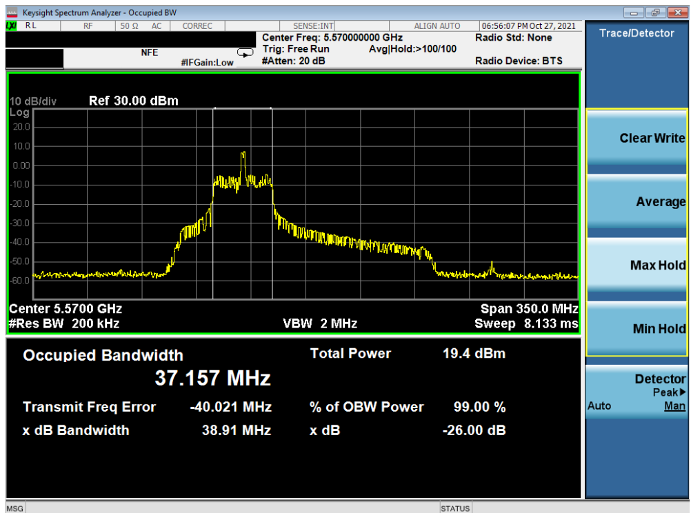
Plot 7-24. 26dB Bandwidth Plot MIMO ANT1 (160MHz BW L 802.11ax – 26 Tones (UNII Band 2C) – Ch. 114)
