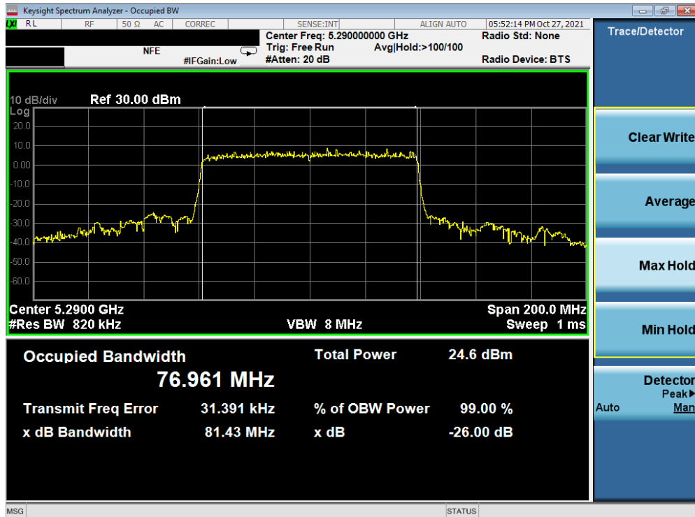
Plot 7-39. 26dB Bandwidth Plot MIMO ANT1 (80MHz BW 802.11ax – 996 Tones (UNII Band 2A) – Ch. 58)
