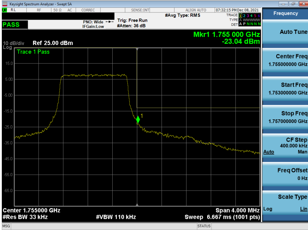
Plot 7-84. Upper Band Edge Plot (LTE Band 4 – 1.4MHz QPSK – Full RB)
