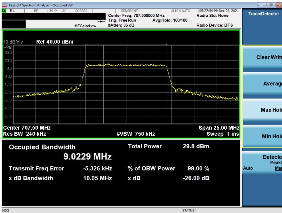
Plot 7-2. Occupied Bandwidth Plot (LTE Band 12 - 10MHz 16-QAM - Full RB)
