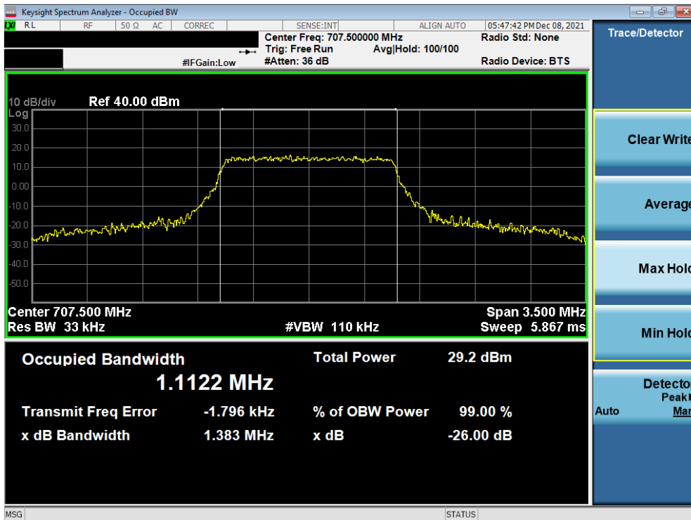
Plot 7-8. Occupied Bandwidth Plot (LTE Band 12 – 1.4MHz 16-QAM - Full RB)
