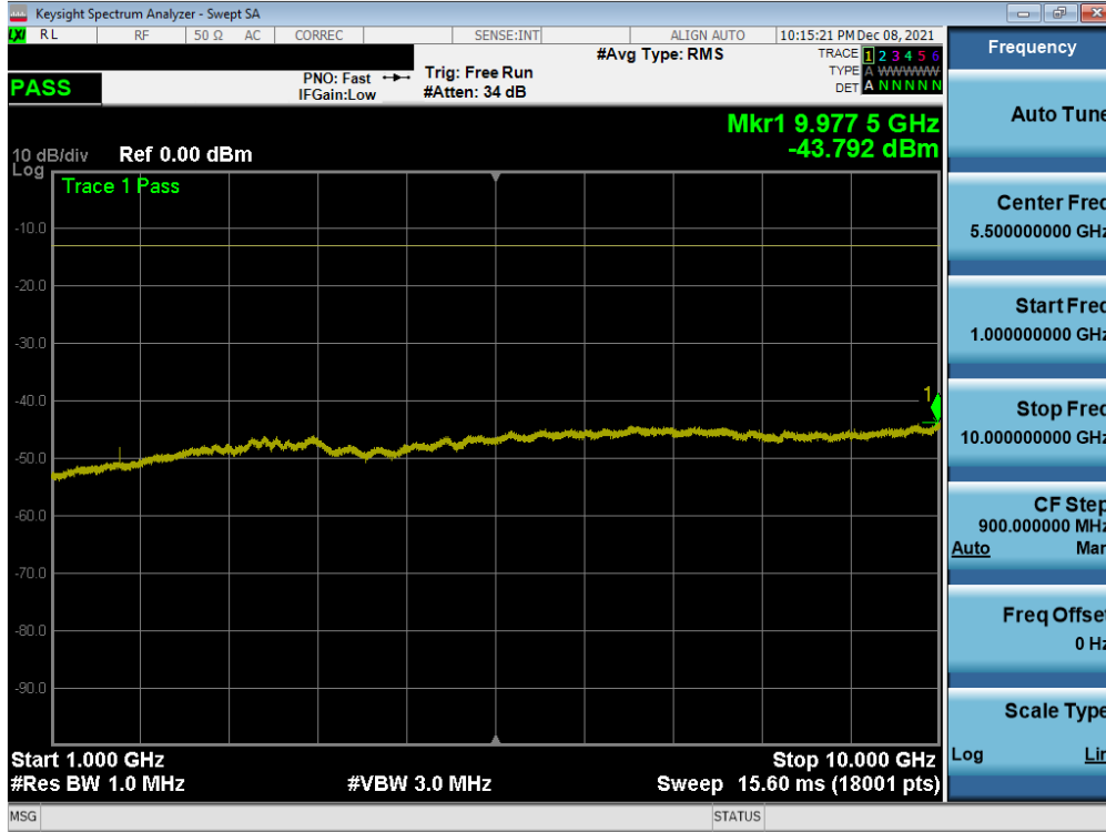
Plot 7-20. Conducted Spurious Plot (LTE Band 5 - 10MHz QPSK - 1 RB - High Channel)
