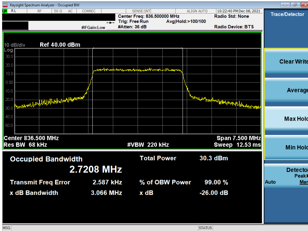
Plot 7-6. Occupied Bandwidth Plot (LTE Band 5 - 3MHz 16-QAM - Full RB)
