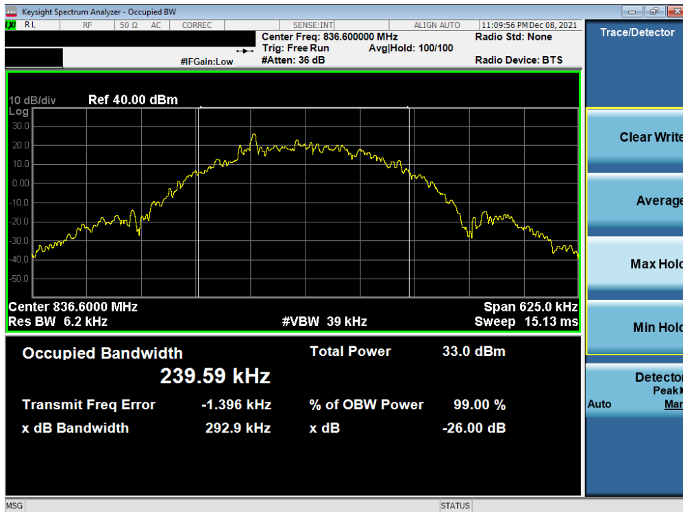
Plot 7-10. Occupied Bandwidth Plot (EDGE, Ch. 190)
