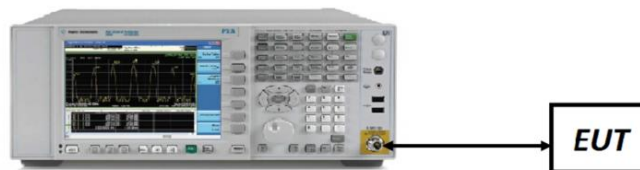
Figure 7-5. Test Instrument & Measurement Setup
