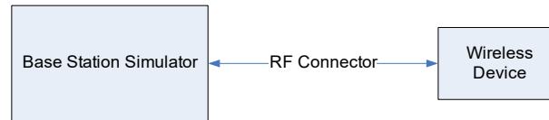
Figure 9-4 Power Measurement Setup – NR FDD
