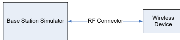
Figure 9-3 Power Measurement Setup
