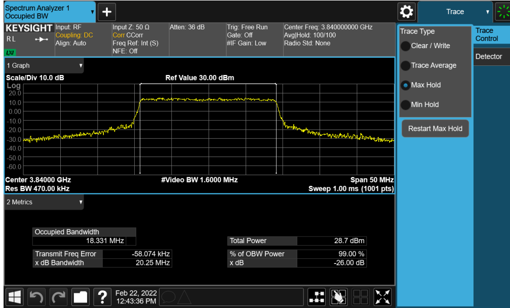
Plot 7-68. Occupied Bandwidth Plot (NR Band n77 - 20MHz 16-QAM - Full RB - ANT F)
