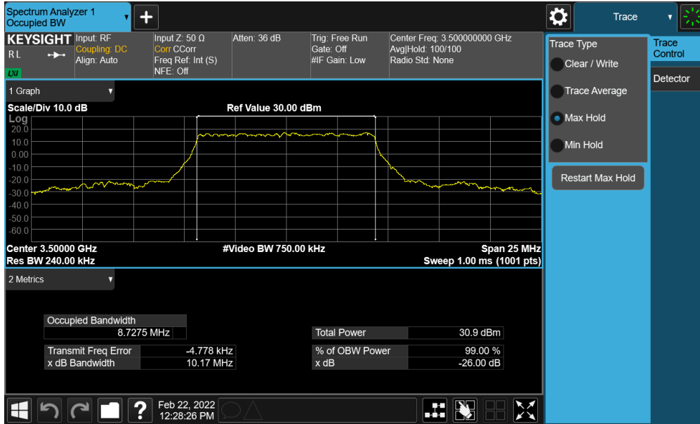
Plot 7-39. Occupied Bandwidth Plot (NR Band n77 (DoD) - 10MHz \pi/2 BPSK - Full RB - ANT F)
