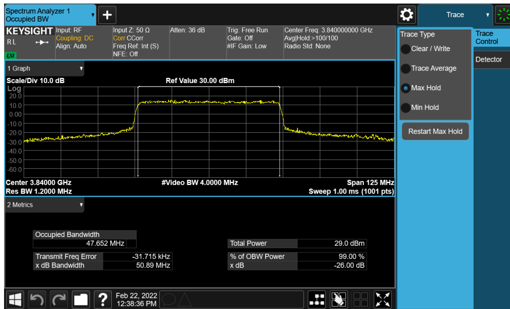
Plot 7-59. Occupied Bandwidth Plot (NR Band n77 - 50MHz 16-QAM - Full RB - ANT F)
