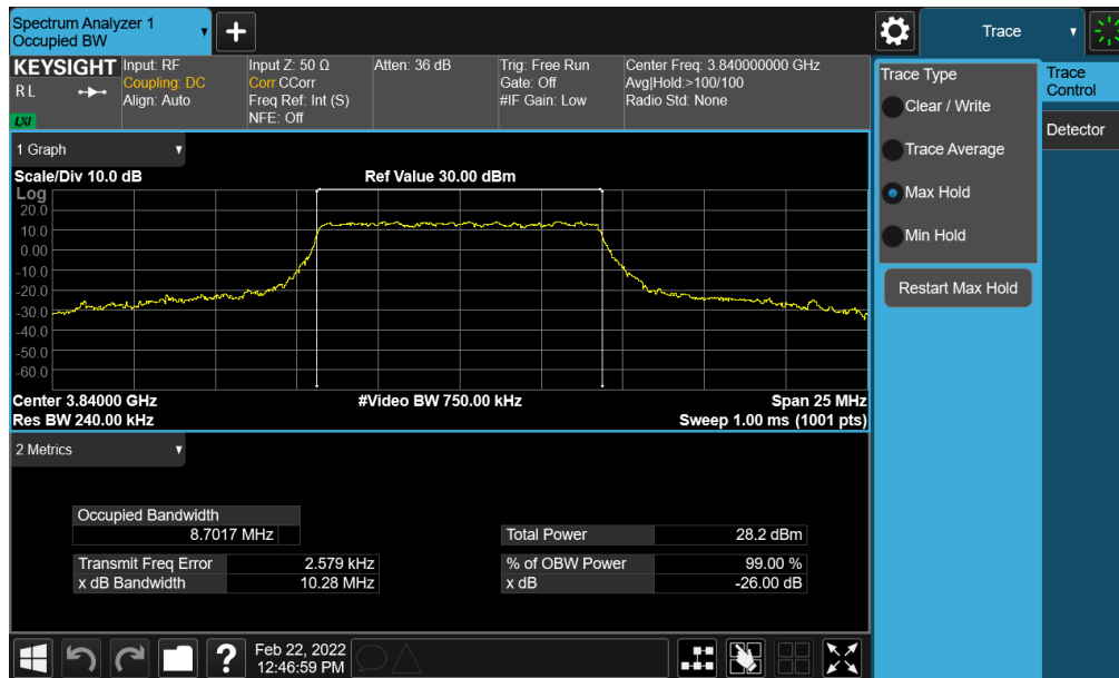
Plot 7-74. Occupied Bandwidth Plot (NR Band n77 - 10MHz 16-QAM - Full RB - ANT F)
