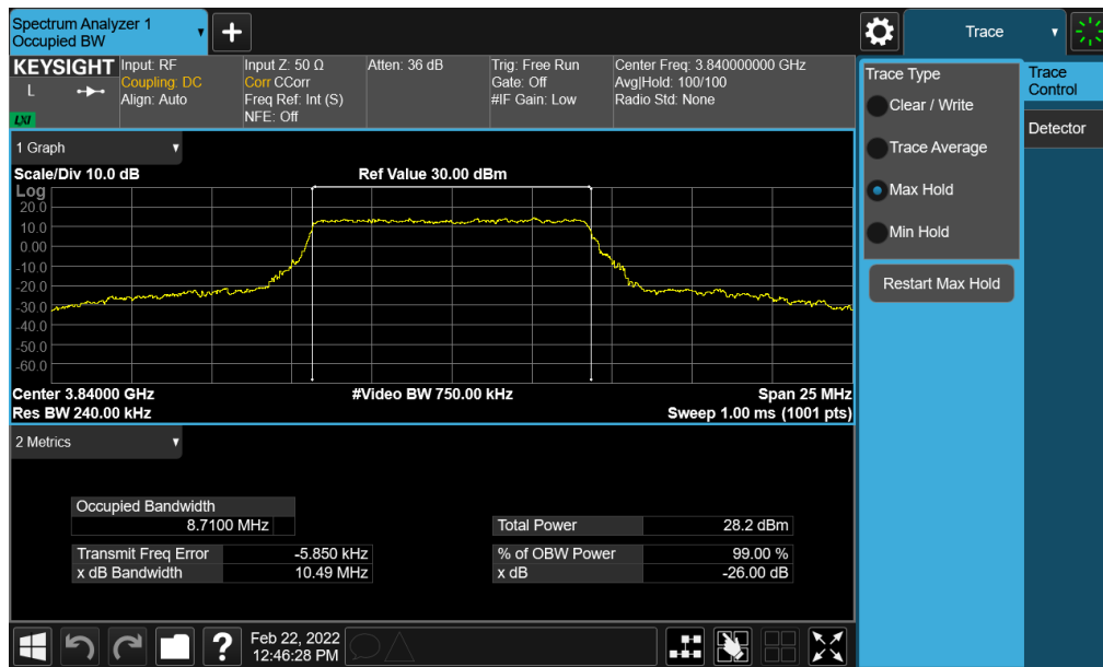
Plot 7-73. Occupied Bandwidth Plot (NR Band n77 - 10MHz QPSK - Full RB - ANT F)
