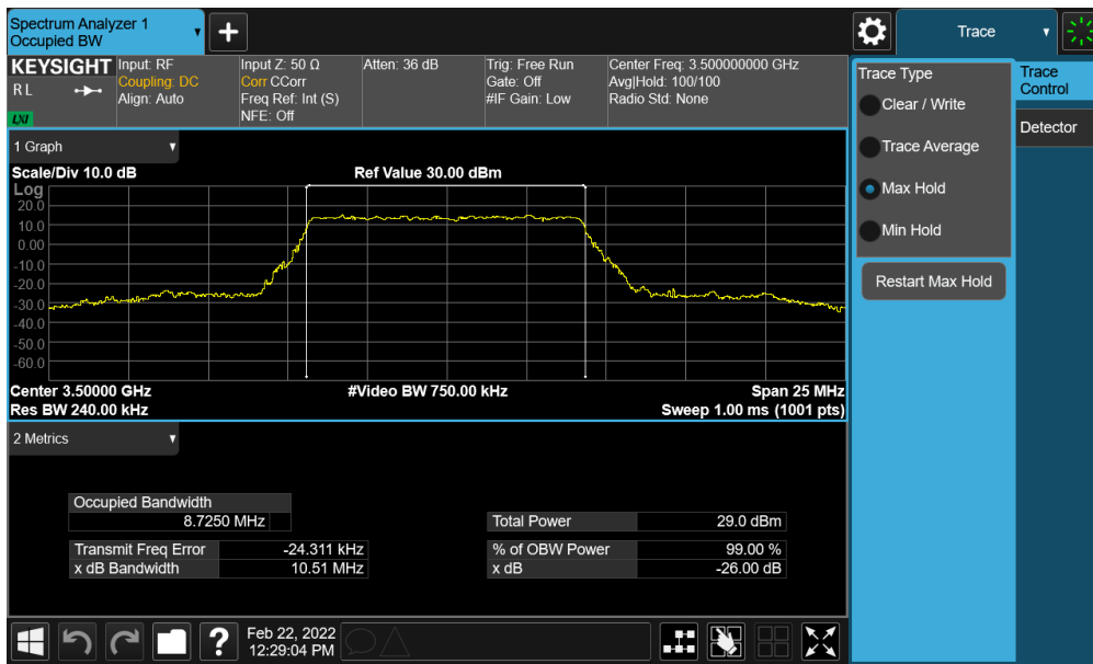
Plot 7-40. Occupied Bandwidth Plot (NR Band n77 (DoD) - 10MHz QPSK - Full RB - ANT F)
