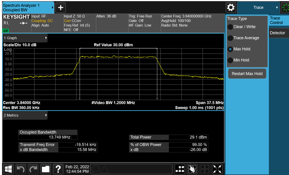
Plot 7-70. Occupied Bandwidth Plot (NR Band n77 - 15MHz QPSK - Full RB - ANT F)
