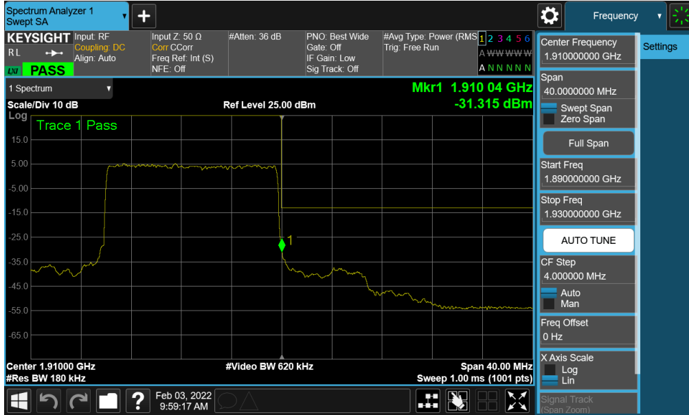
Plot 7-30. Upper Band Edge Plot (NR Band n2 - 15MHz QPSK – Full RB)
