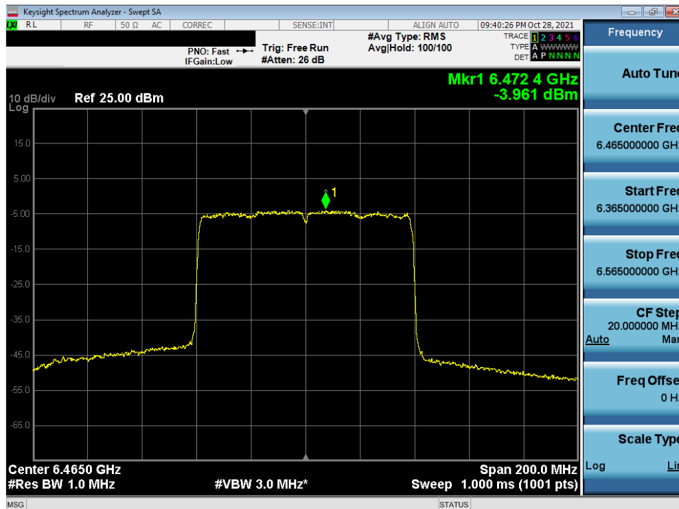
Plot 7-181. Power Spectral Density Measurement Plot MIMO ANT2 (80MHz 802.11ax (UNII Band 6) – Ch. 103)
