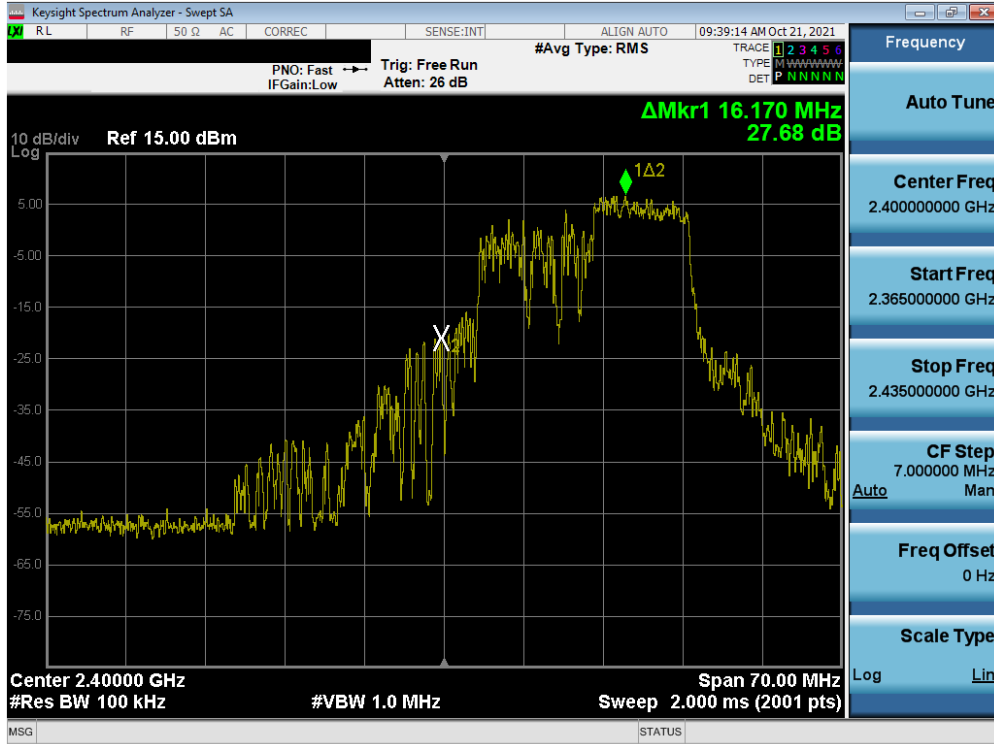
Plot 7-36. Band Edge Plot MIMO ANT2 (802.11ax OFDMA – 106 Tones – Ch. 1)
