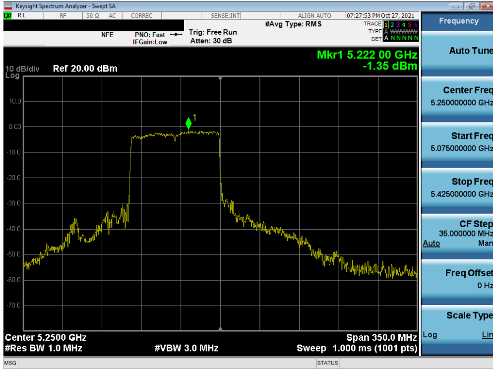
Plot 7-280. Power Spectral Density Plot MIMO ANT2 (160MHz BW L 802.11ax – Full Tones (UNII Band 1/2A) – Ch. 50)
