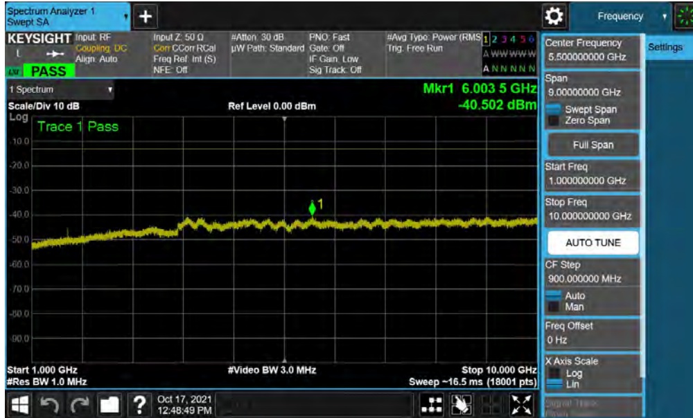
Plot 7-13. Conducted Spurious Plot (LTE Band 26 - 15MHz QPSK - RB Size 1, RB Offset 0)
