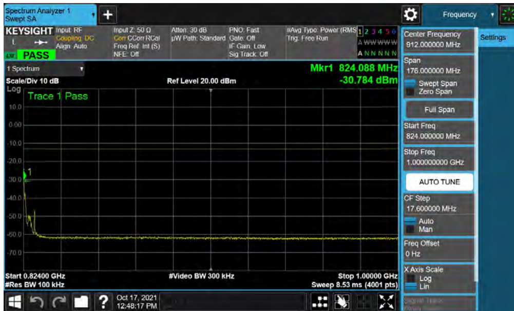
Plot 7-12. Conducted Spurious Plot (LTE Band 26 - 15MHz QPSK - RB Size 1, RB Offset 0)
