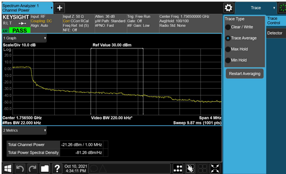
Plot 7-105. Upper Extended Band Edge Plot (LTE Band 4 - 3MHz QPSK – Full RB)
