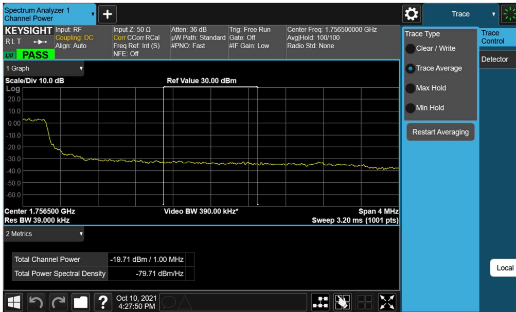
Plot 7-99. Upper Extended Band Edge Plot (LTE Band 4 - 5MHz QPSK – Full RB)
