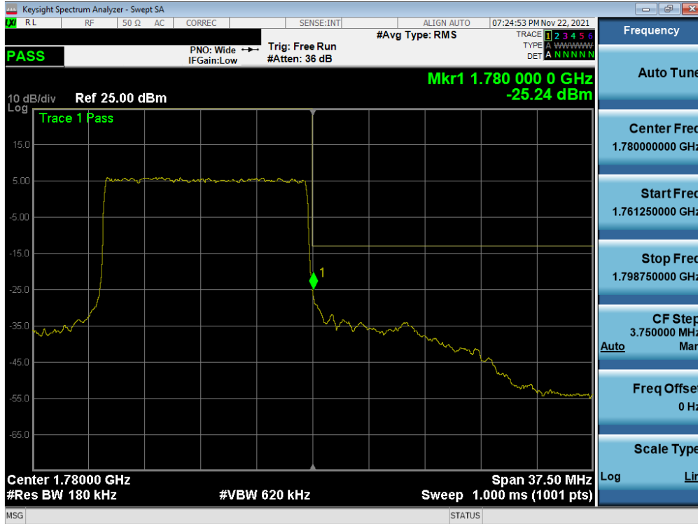
Plot 7-31. Upper Band Edge Plot (NR Band n66 – 15.0MHz - Full RB – ANT A)
