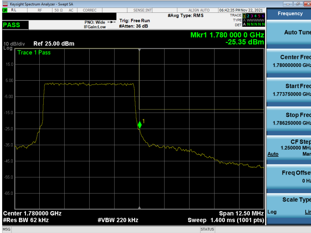
Plot 7-39. Upper Band Edge Plot (NR Band n66 – 5.0MHz - Full RB – ANT A)
