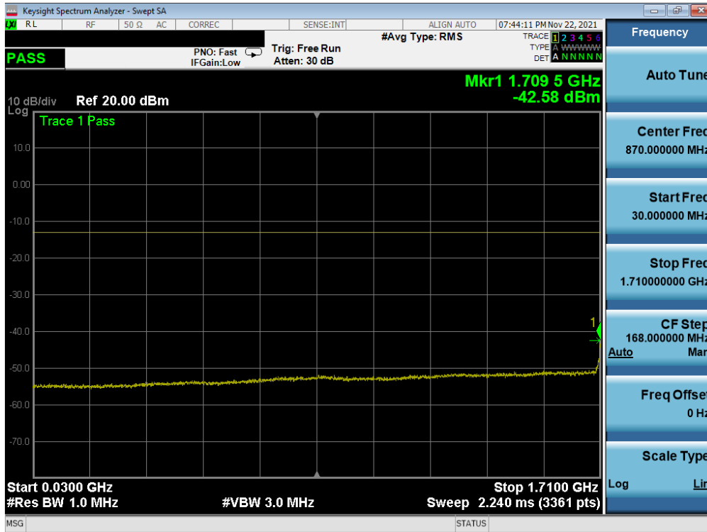
Plot 7-16. Conducted Spurious Plot (NR Band n66 -20MHz - 1 RB - Low Channel – ANT A)
