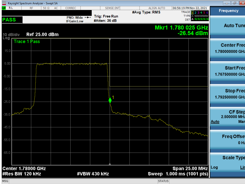
Plot 7-35. Upper Band Edge Plot (NR Band n66 – 10.0MHz - Full RB – ANT A)
