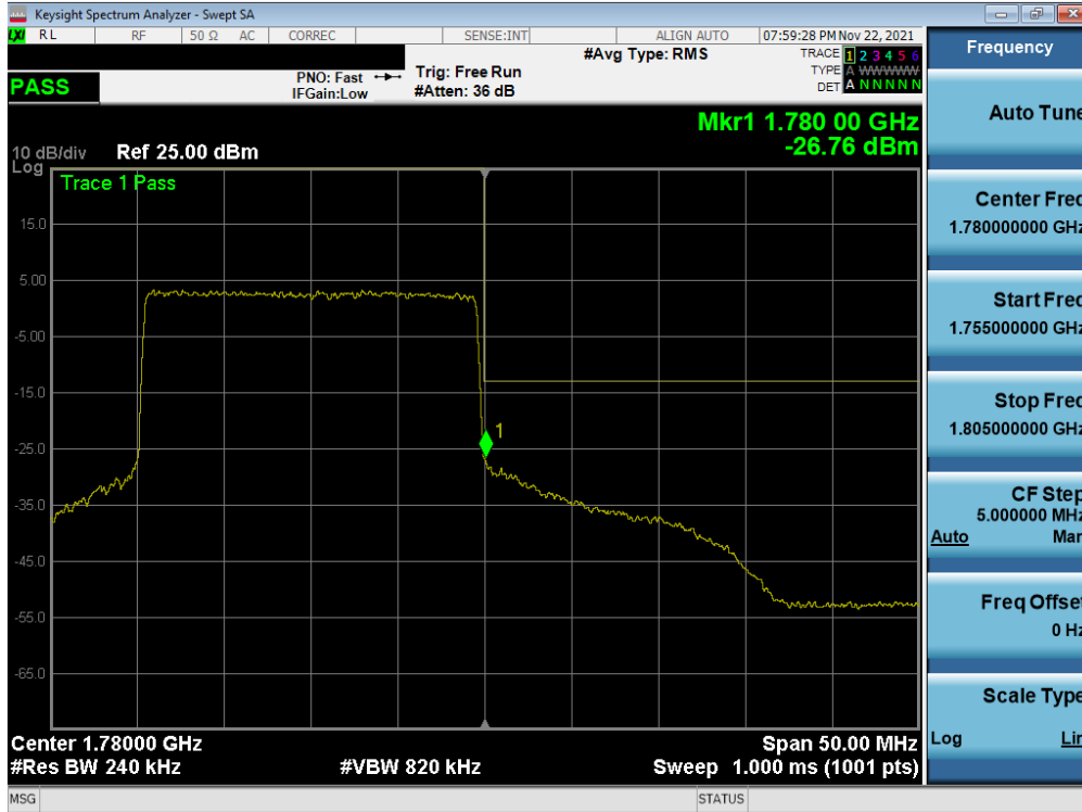
Plot 7-27. Upper Band Edge Plot (NR Band n66 – 20.0MHz - Full RB – ANT A)
