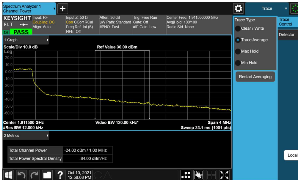
Plot 7-76. Extended Upper Band Edge Plot (LTE Band 2 – 1.4MHz QPSK – Full RB)
