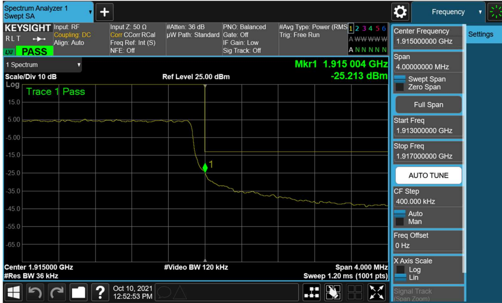
Plot 7-71. Upper Band Edge Plot (LTE Band 25 - 3MHz QPSK – Full RB)
