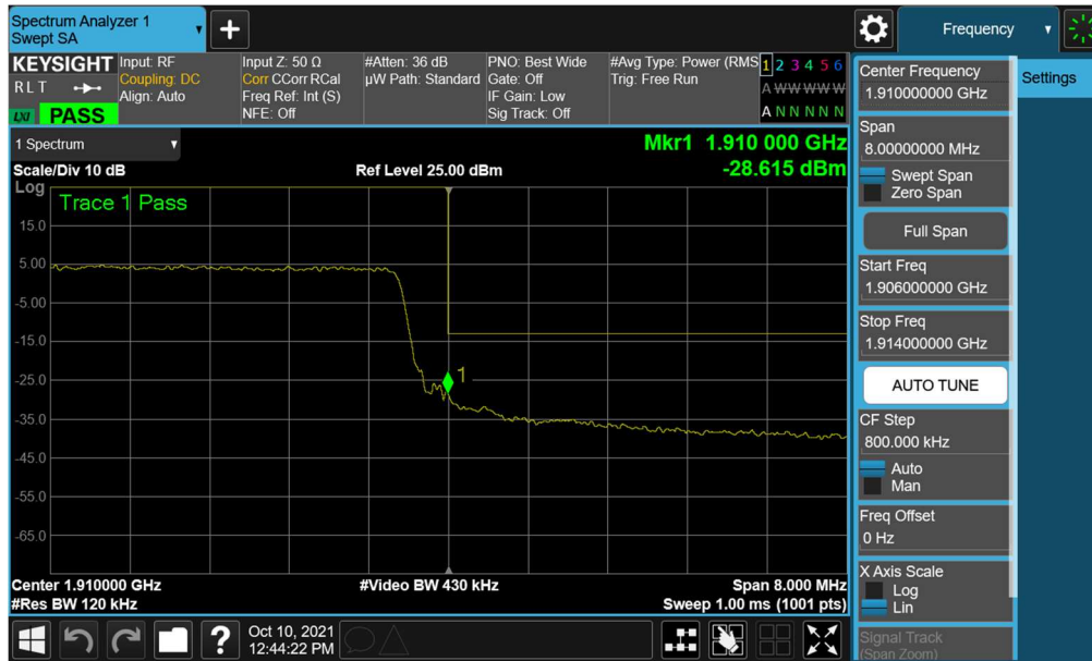
Plot 7-57. Upper Band Edge Plot (LTE Band 2 - 10MHz QPSK – Full RB)
