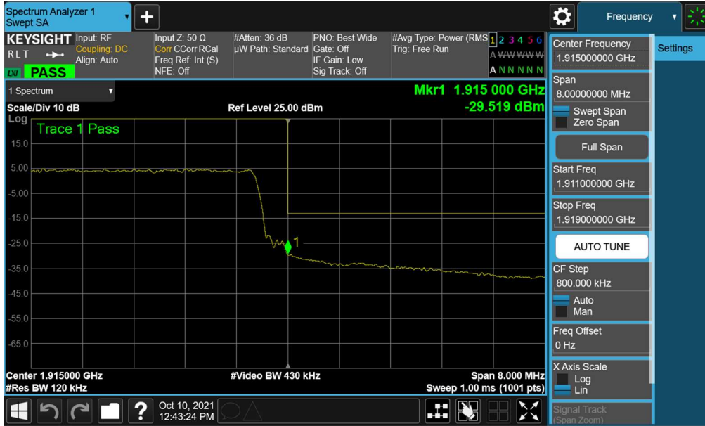
Plot 7-59. Upper Band Edge Plot (LTE Band 25 - 10MHz QPSK – Full RB)
