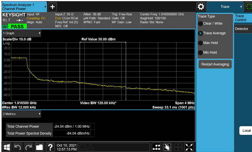
Plot 7-78. Extended Upper Band Edge Plot (LTE Band 25 – 1.4MHz QPSK – Full RB)
