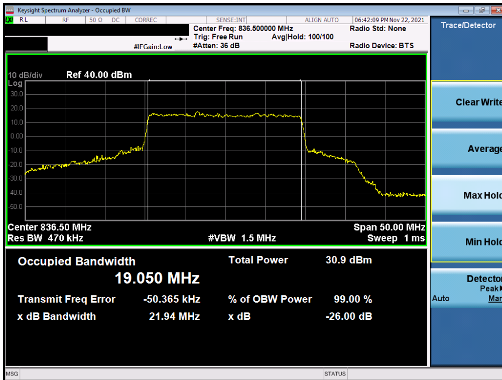
Plot 7-2. Occupied Bandwidth Plot (NR Band n5 - 20MHz QPSK - Full RB)
