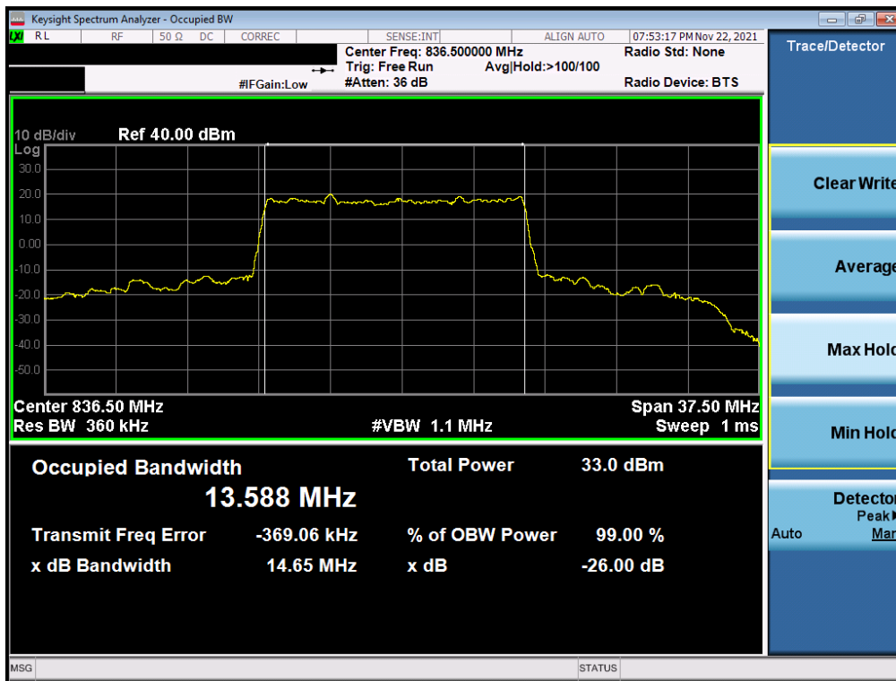
Plot 7-4. Occupied Bandwidth Plot (NR Band n5 - 15MHz \pi/2 BPSK - Full RB)
