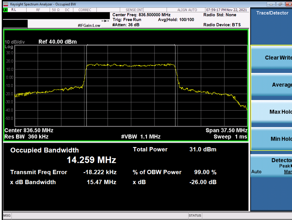
Plot 7-5. Occupied Bandwidth Plot (NR Band n5 - 15MHz QPSK - Full RB)
