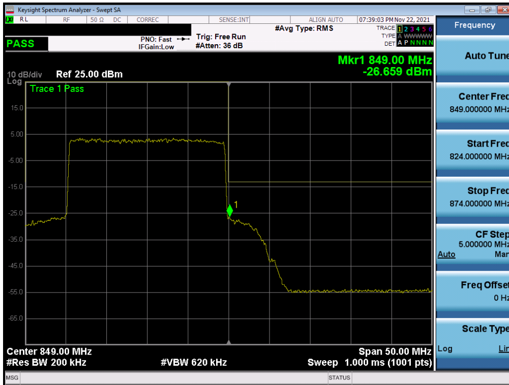
Plot 7-26. Upper Band Edge Plot (NR Band n5 – 20.0MHz - Full RB)
