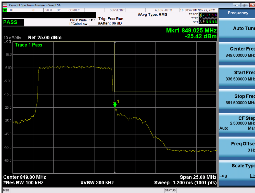
Plot 7-30. Upper Band Edge Plot (NR Band n5 – 10.0MHz - Full RB)
