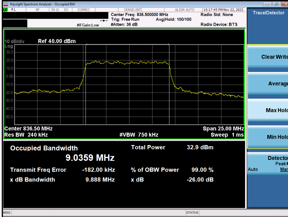
Plot 7-7. Occupied Bandwidth Plot (NR Band n5 - 10MHz \pi/2 BPSK - Full RB)
