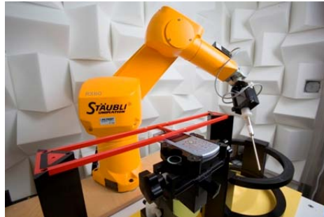
Figure 4-3 SPEAG Robotic System
