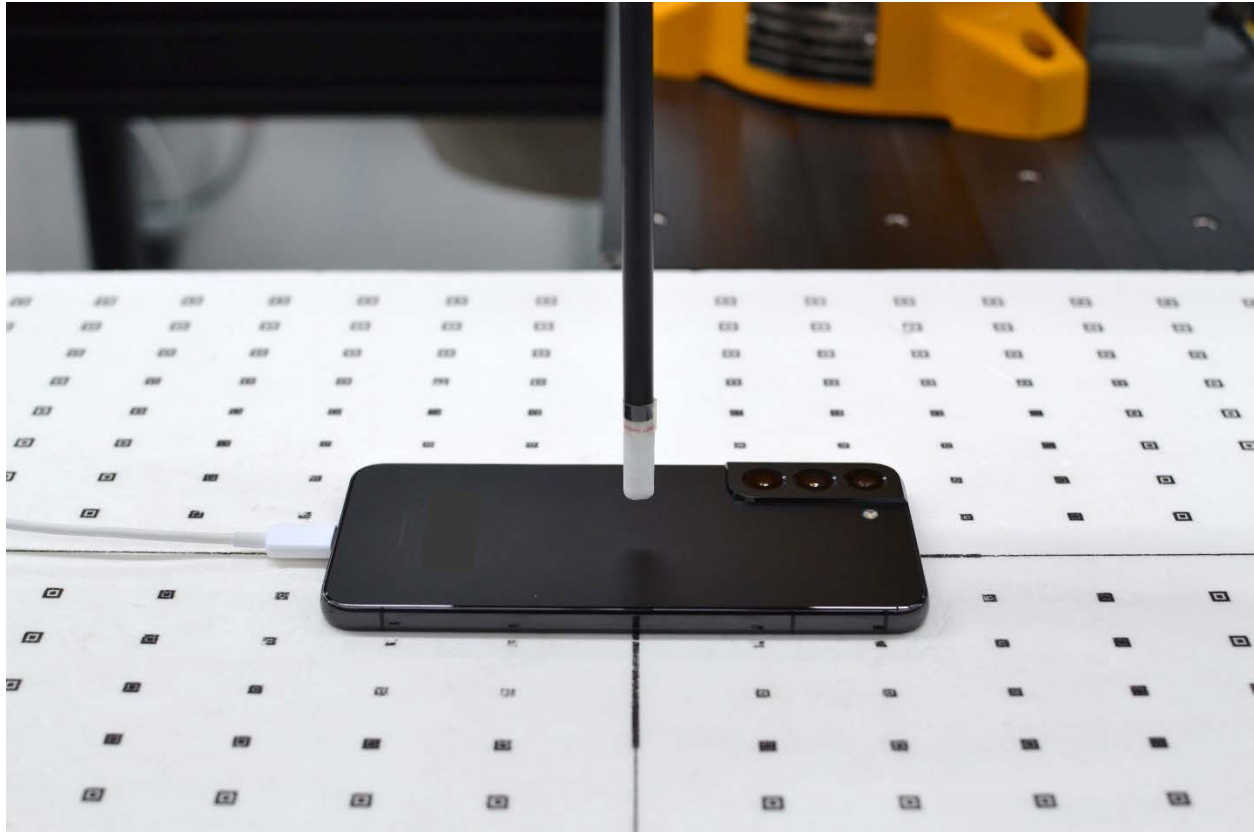
Figure D-6 Near Field Power Density Test Setup Photo – Back Side at 10mm
