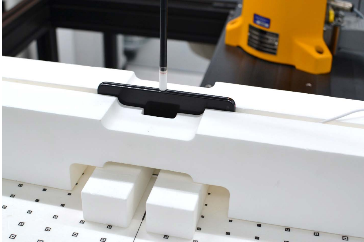
Figure D-4 Near Field Power Density Test Setup Photo –Right Edge at 2mm
