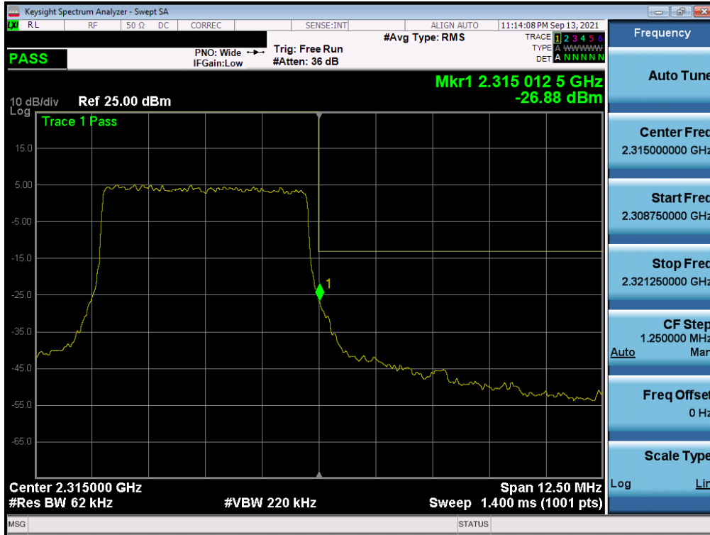
Plot 7-201. Upper Band Edge Plot (NR Band n30 - 5MHz CP-OFDM-QPSK – Full RB - Ant A)
