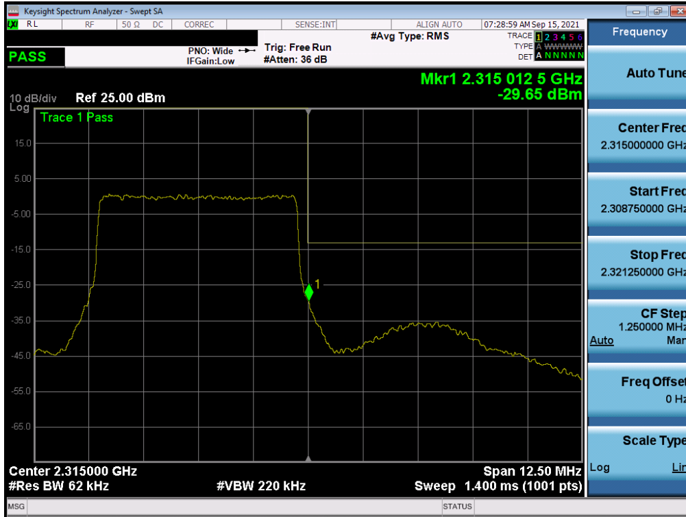
Plot 7-209. Upper Band Edge Plot (NR Band n30 - 5MHz CP-OFDM-QPSK – Full RB - Ant I)
