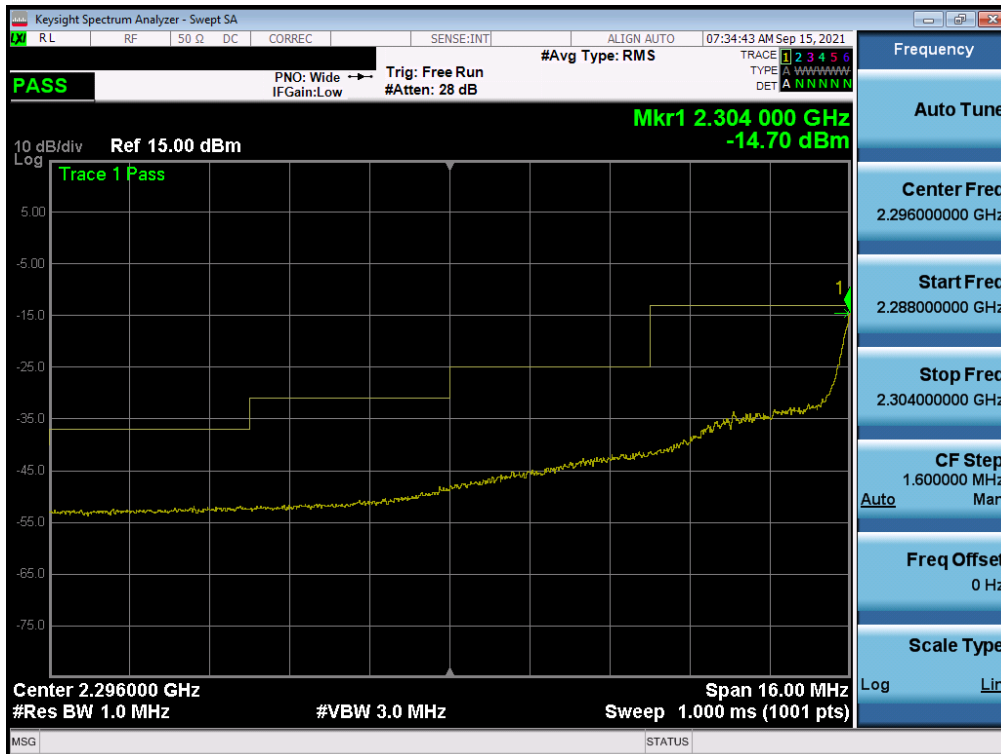
Plot 7-208. Extended Lower Band Edge Plot (NR Band n30 - 5MHz CP-OFDM-QPSK – Full RB - Ant I)
