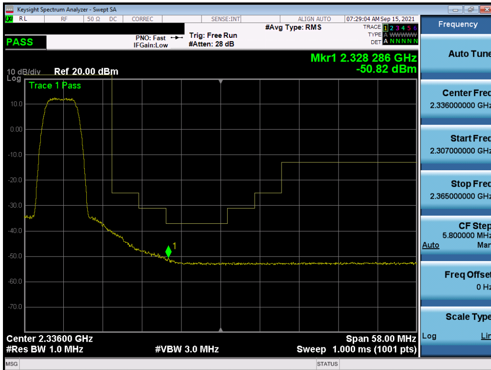
Plot 7-210. Extended Upper Band Edge Plot (NR Band n30 - 5MHz CP-OFDM-QPSK – Full RB - Ant I)
