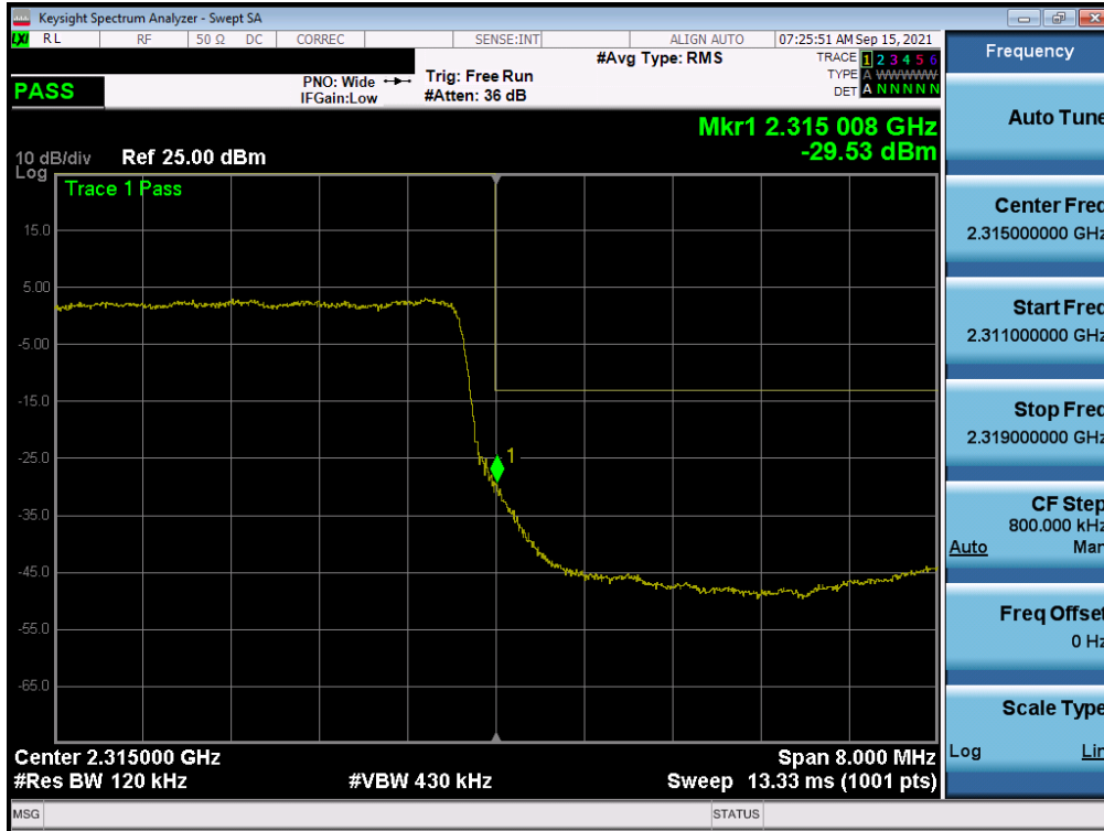
Plot 7-205. Upper Band Edge Plot (NR Band n30 - 10MHz CP-OFDM-QPSK – Full RB - Ant 1)
