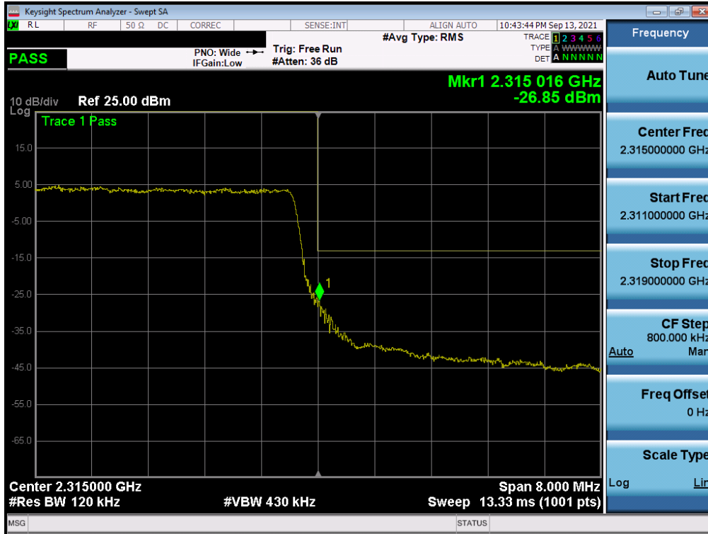
Plot 7-197. Upper Band Edge Plot (NR Band n30 - 10MHz CP-OFDM-QPSK – Full RB - Ant A)
