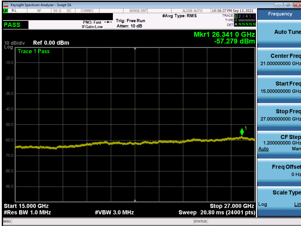
Plot 7-116. Conducted Spurious Plot (NR Band n30 - 10MHz QPSK - RB Size 1, RB Offset 0 – Ant A)
