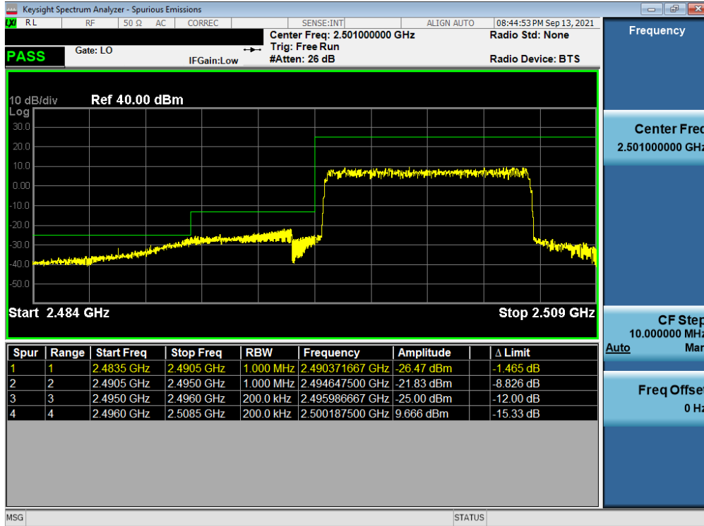
Plot 7-189. Lower ACP Plot (LTE Band 41(PC2) - 10MHz QPSK - Full RB)
