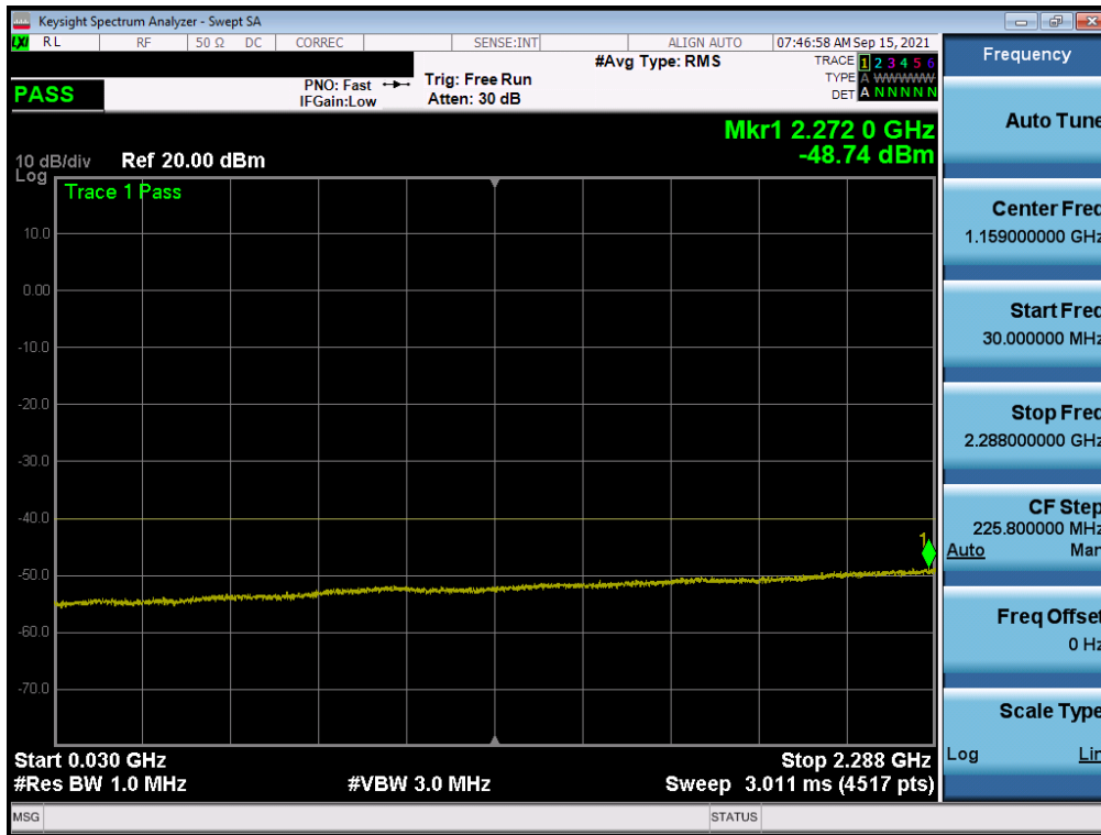
Plot 7-117. Conducted Spurious Plot (NR Band n30 - 10MHz QPSK - RB Size 1, RB Offset 0 – Ant I)
