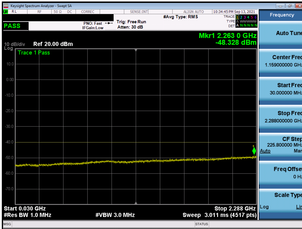
Plot 7-114. Conducted Spurious Plot (NR Band n30 - 10MHz QPSK - RB Size 1, RB Offset 0 – Ant A)
