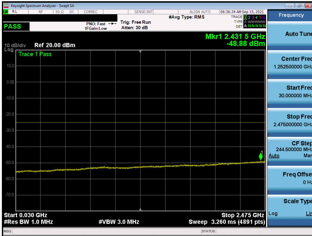
Plot 7-120. Conducted Spurious Plot (NR Band n7 - 20MHz QPSK - RB Size 1, RB Offset 0 - Low Channel Ant B)
