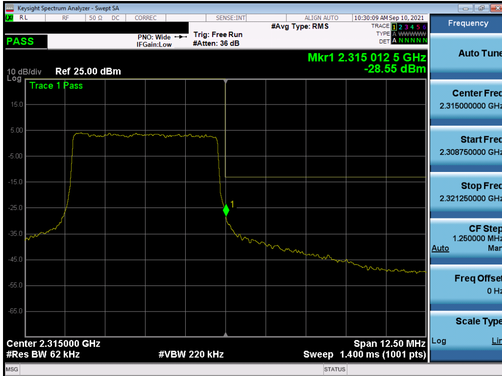
Plot 7-175. Upper Band Edge Plot (LTE Band 30 - 5MHz QPSK - Full RB)
