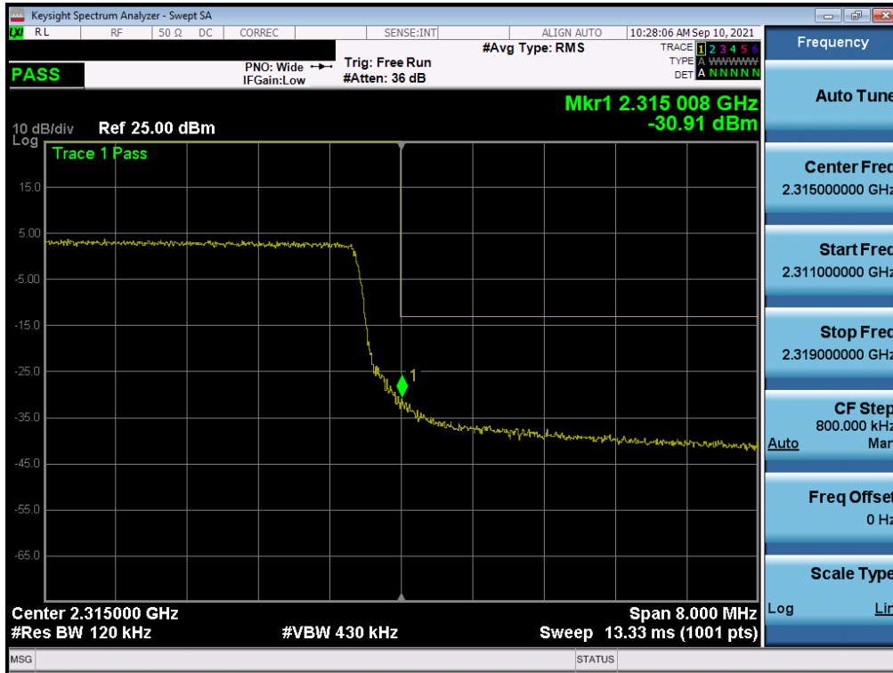
Plot 7-171. Upper Band Edge Plot (LTE Band 30 - 10MHz QPSK – Full RB)
