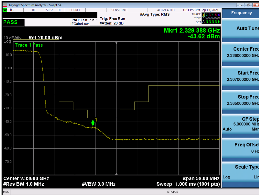
Plot 7-198. Extended Upper Band Edge Plot (NR Band n30 - 10MHz CP-OFDM-QPSK – Full RB - Ant A)
