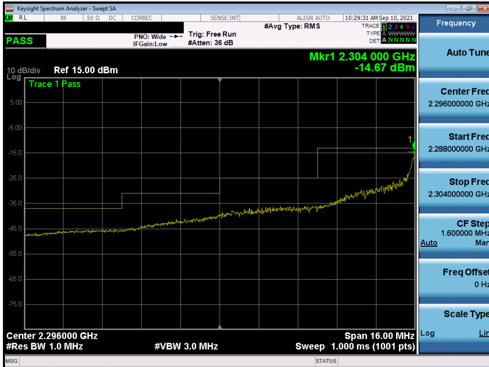
Plot 7-174. Extended Lower Band Edge Plot (LTE Band 30 - 5MHz QPSK – Full RB)
