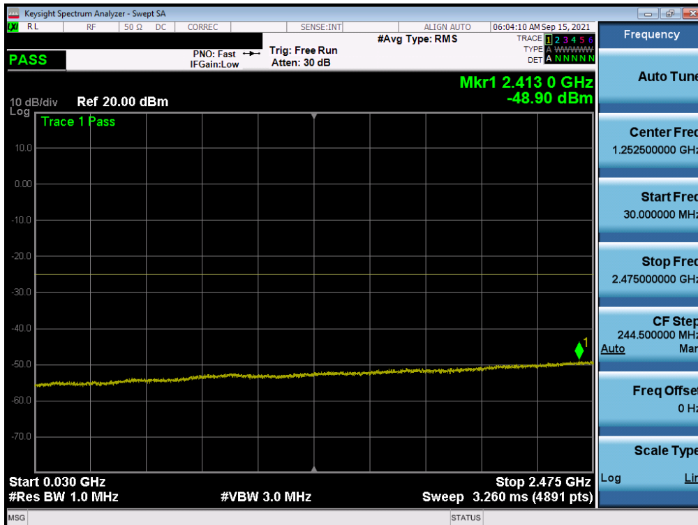
Plot 7-123. Conducted Spurious Plot (NR Band n7 - 20MHz QPSK - RB Size 1, RB Offset 0 - Mid Channel Ant B)
