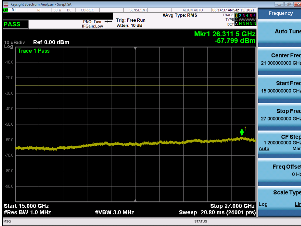
Plot 7-128. Conducted Spurious Plot (NR Band n7 - 20MHz QPSK - RB Size 1, RB Offset 0 - High Channel Ant B)
