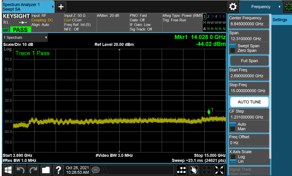
Plot 7-160. Conducted Spurious Plot (NR Band n41 - 100MHz QPSK - RB Size 1, RB Offset 0 - Mid Channel Ant D)
