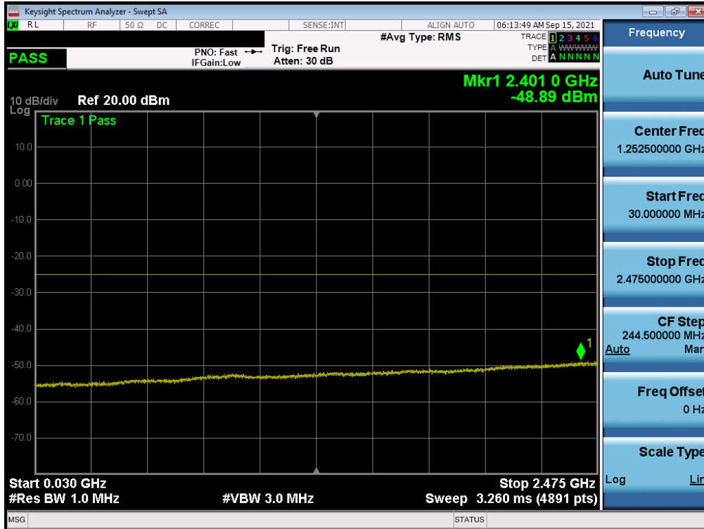
Plot 7-126. Conducted Spurious Plot (NR Band n7 - 20MHz QPSK - RB Size 1, RB Offset 0 - High Channel Ant B)
