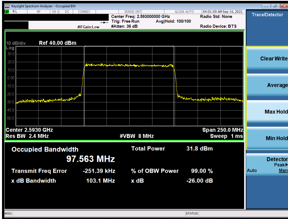
Plot 7-56. Occupied Bandwidth Plot (NR Band n41 - 100MHz 16-QAM - Full RB - Ant I)
