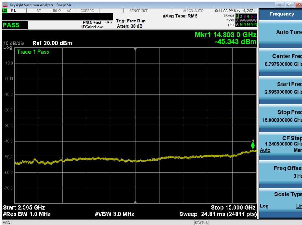
Plot 7-91. Conducted Spurious Plot (LTE Band 7 - 20MHz QPSK - RB Size 1, RB Offset 0 - High Channel)
