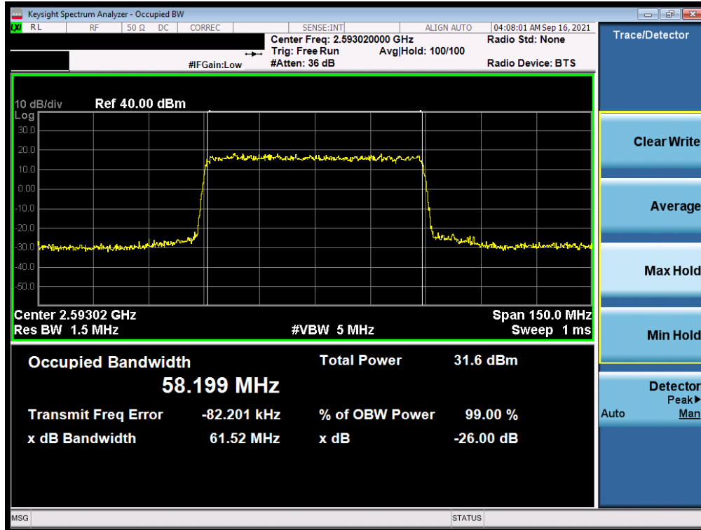
Plot 7-68. Occupied Bandwidth Plot (NR Band n41 - 60MHz 16-QAM - Full RB - Ant I)
