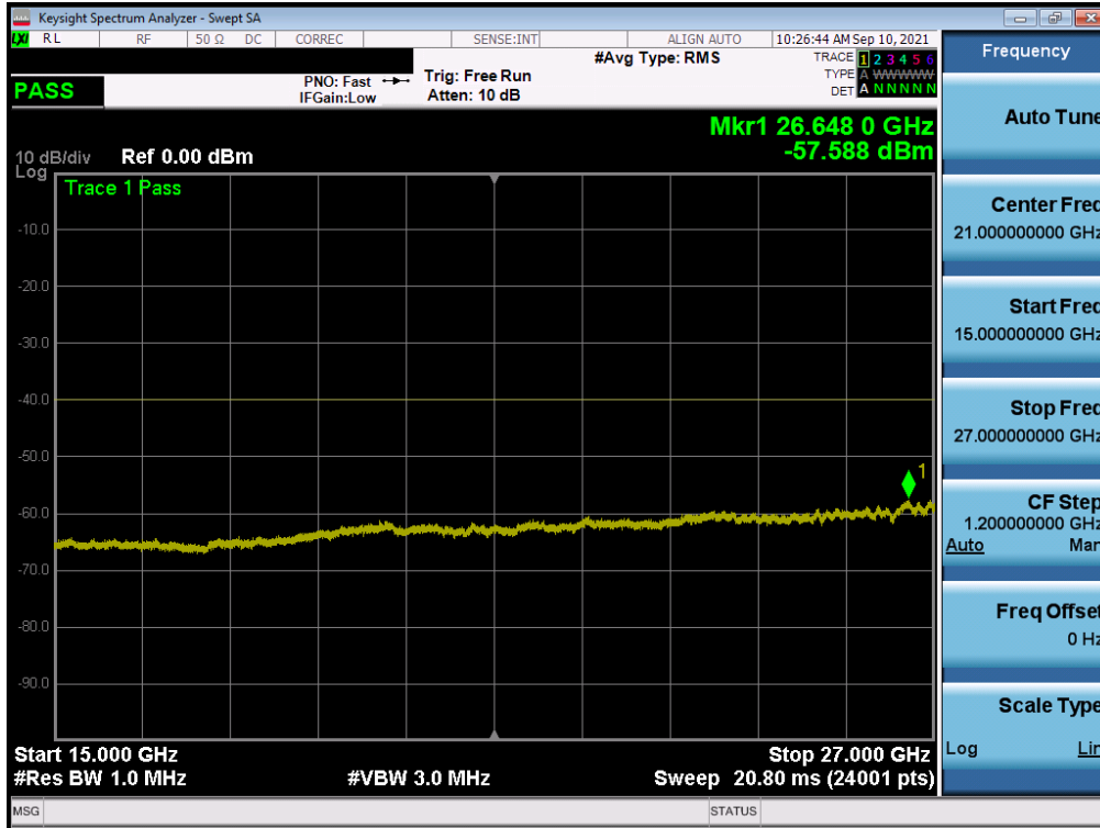
Plot 7-83. Conducted Spurious Plot (LTE Band 30 - 10MHz QPSK - RB Size 1, RB Offset 0)
