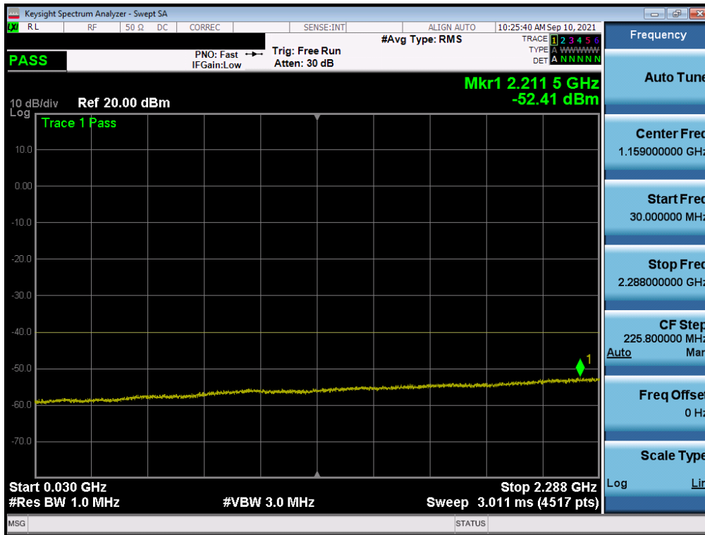
Plot 7-81. Conducted Spurious Plot (LTE Band 30 - 10MHz QPSK - RB Size 1, RB Offset 0)
