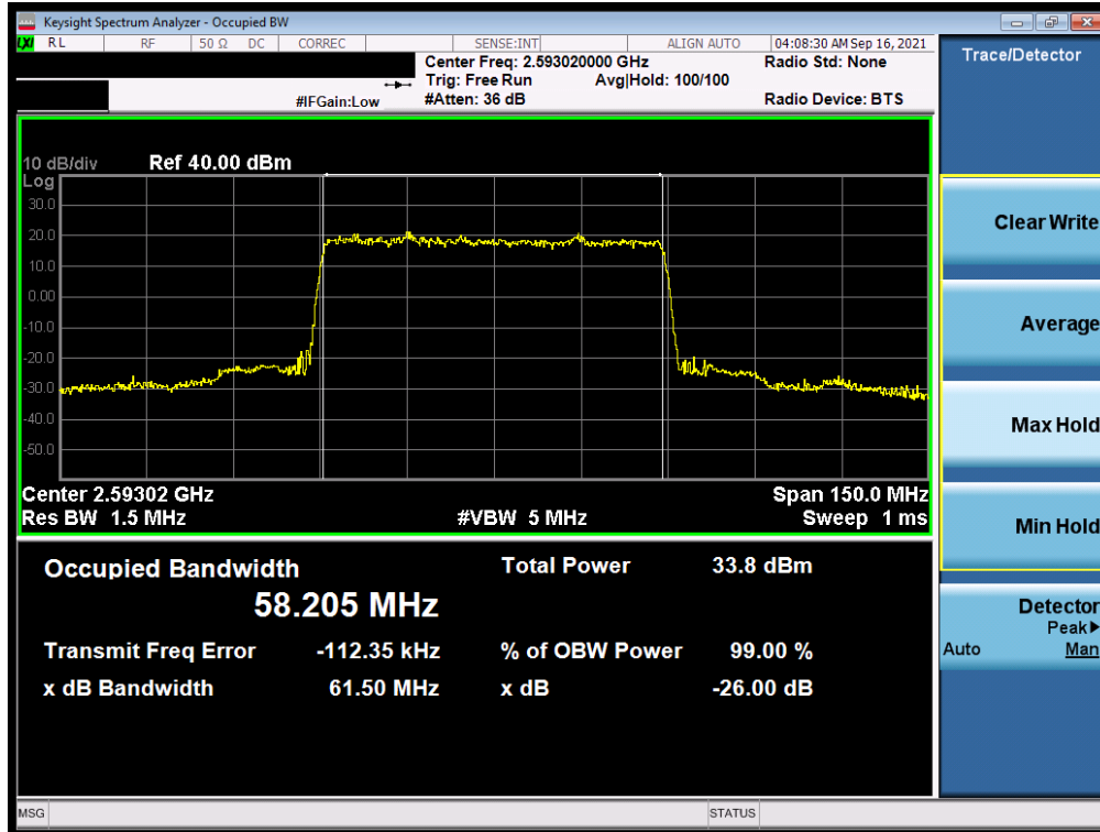
Plot 7-66. Occupied Bandwidth Plot (NR Band n41 - 60MHz \pi/2 BPSK - Full RB - Ant I)
