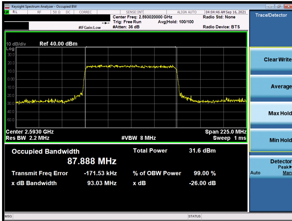
Plot 7-59. Occupied Bandwidth Plot (NR Band n41 - 90MHz 16-QAM - Full RB - Ant I)
